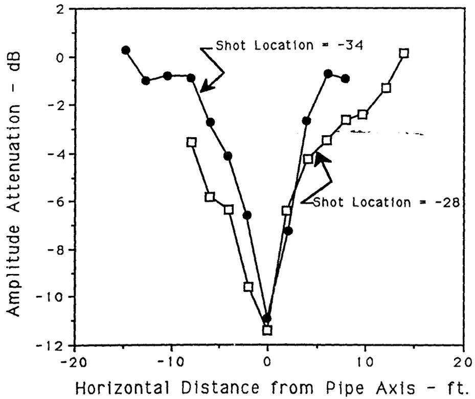
Figure 7. Love wave amplitude attenuation due to scattering.
