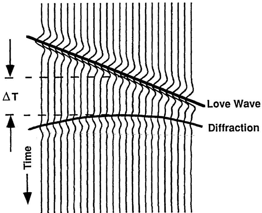
Figure 1b. Synthetic seismogram for Love wave-tunnel interaction.
