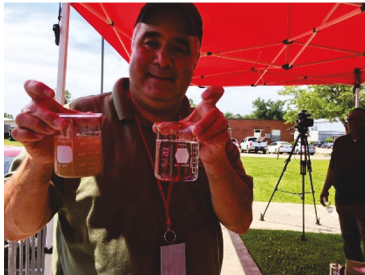
Figure 46. Comparison of samples collected from the system influent (left) and effluent (right).
