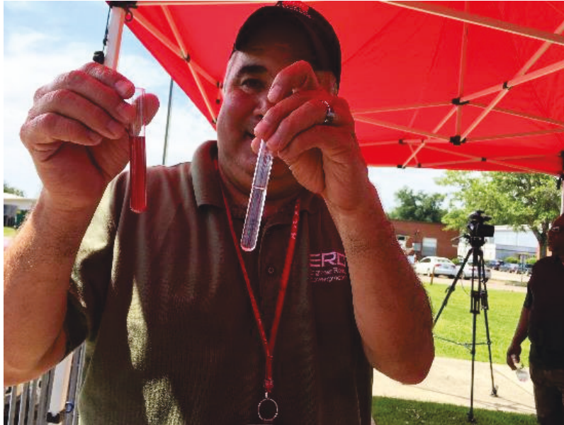
Figure 53. Colorimetric results for total chlorine. Sample on the left is the influent sample and has red color indicating high total chlorine concentration. The sample on the right is from the effluent and has no color, as chlorine is largely removed.
