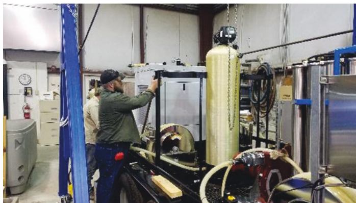
Figure 61. Bracing added to trailer to enhance support for system components (30 November 2017).
