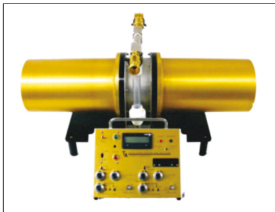
Figure 57. NEX-BETA-ABG radiological detector that could be adapted for the DETS.
