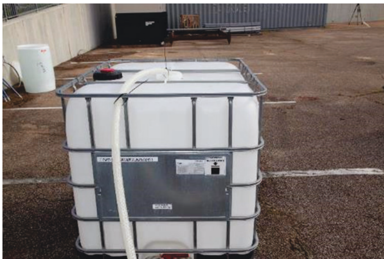
Figure 21. 250 gallon tote used as the influent vessel for the treatment system.
