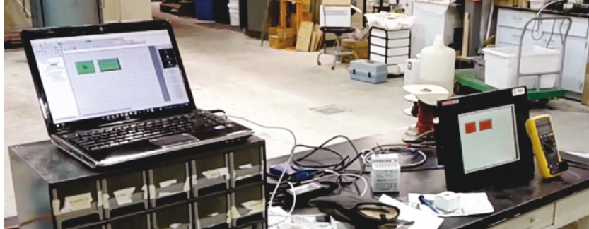
Figure 8. Programming the EZ-touch processor using a laptop computer.
