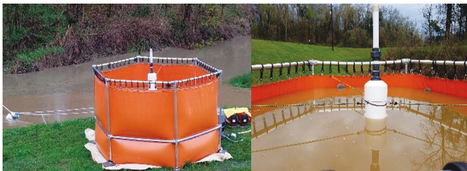
Figure 31. Pictures of the 2,500 gallon sedimentation tank setup for sediment removal testing near creek at WES and picture inside tank showing sediment colored water.
