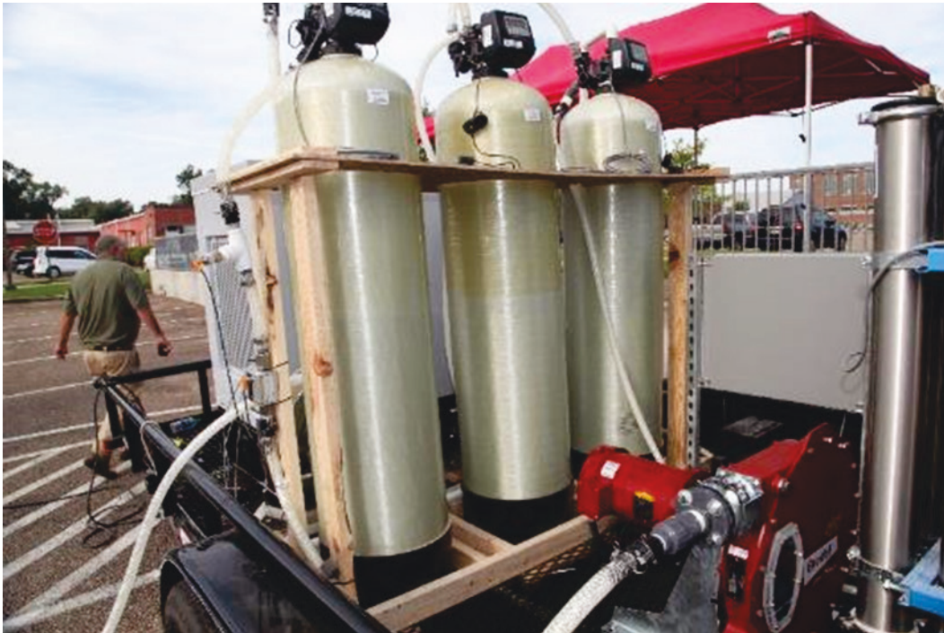
Figure 44. Wood bracing used for unit processes in this study. The wood bracing was replaced by welded metal bracing (Figure 61).
