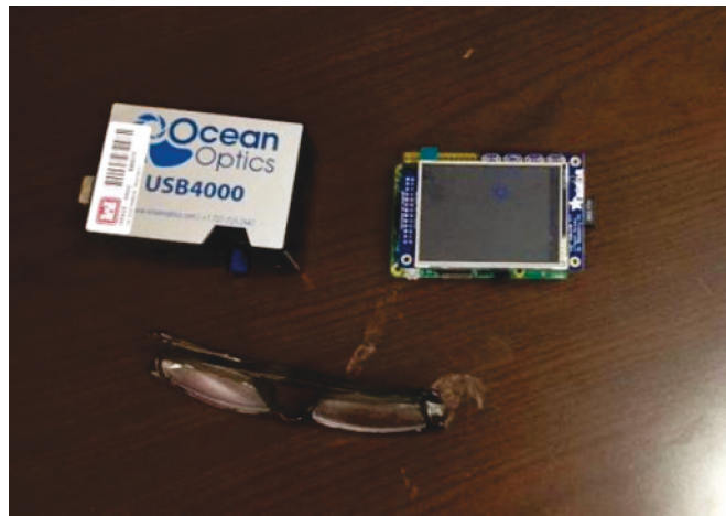
Figure 58. A small, contained spectrophotometer that could be adapted for online monitoring.
