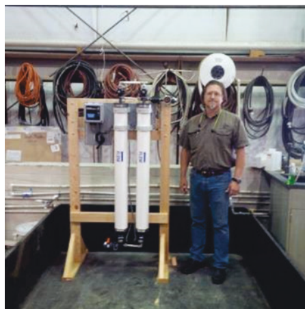
Figure 30. Ultrafiltration columns tested for treatment of cesium and Malathion.
