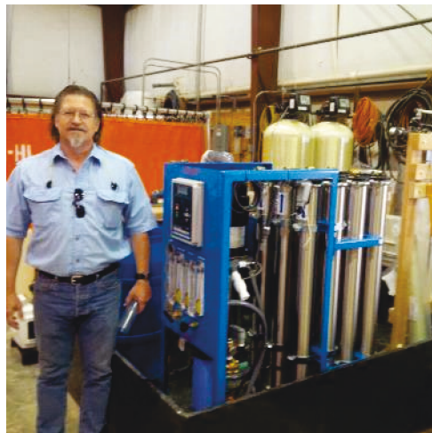
Figure 40. The Applied Membranes Inc. six-stage RO system.
