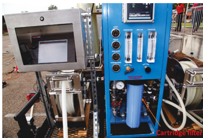
Figure 43. Cartridge Filter protecting the RO system from fine sediments.
