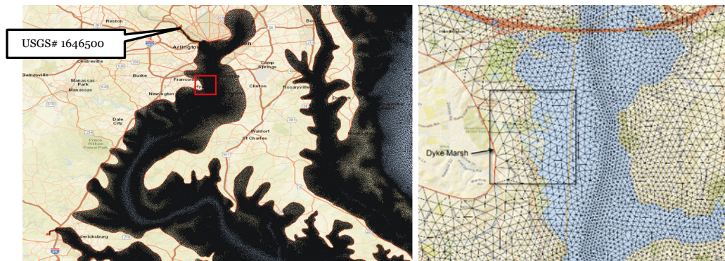
Figure 1-3. Existing NACCS ADCIRC mesh for the Potomac River, with Dyke Marsh region indicated in detail on right. The USGS hydrologic station No. 1646500 is shown in the figure.
