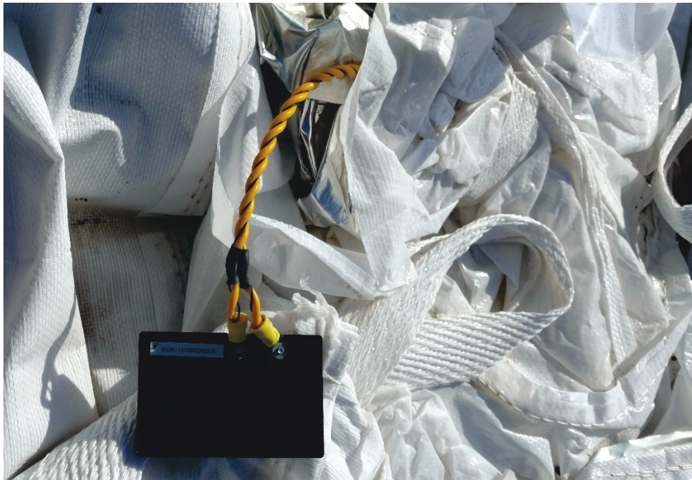
Figure 6. Sensor 2 with RFID transmitter.
