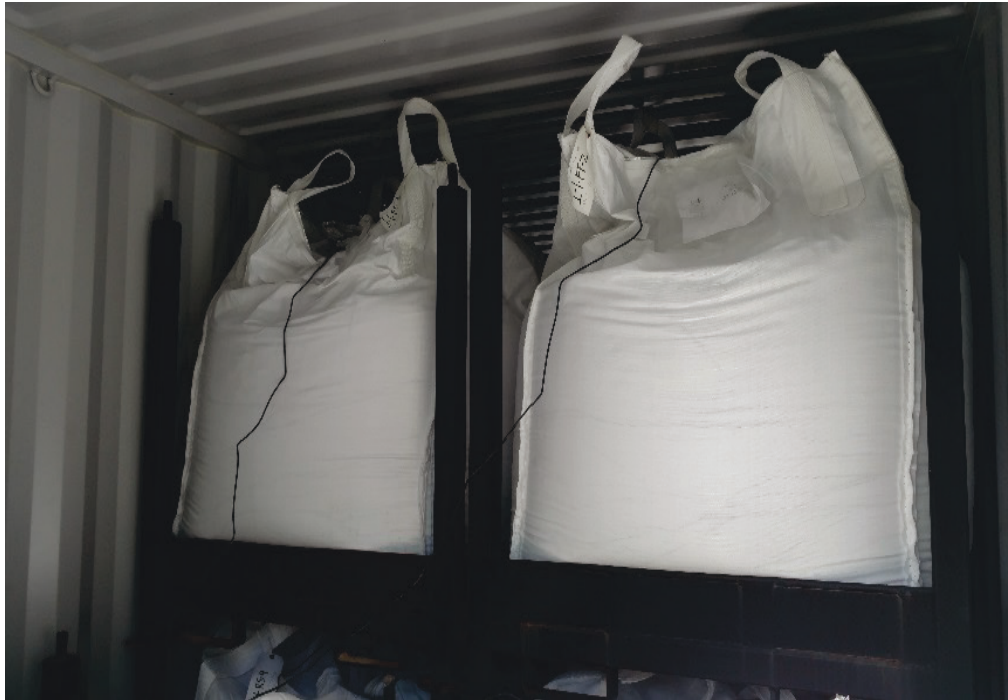
a. Sensor 1 embedded in Super Sacks.
