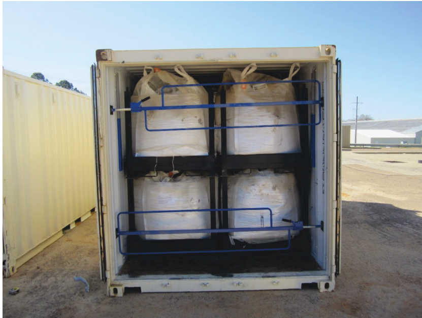
Figure 1. Conex container with Super Sacks in racks.
