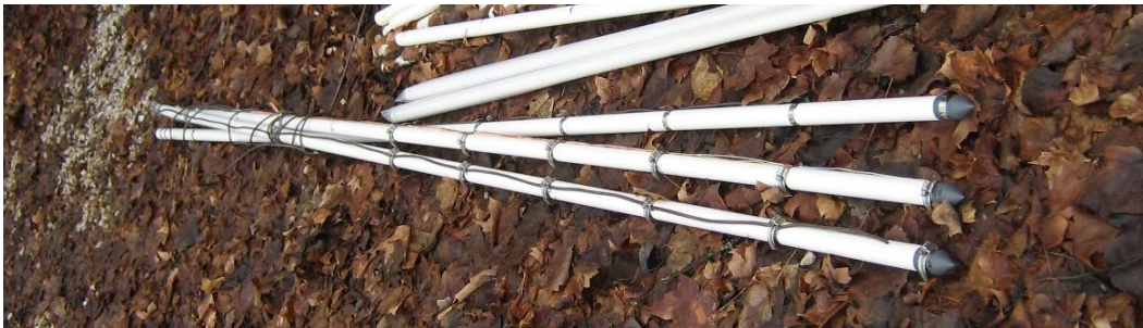
Figure A6. Photograph of the piezometric wells with electric field measurement bands placed every foot from the bottom up to 5 ft then at 7 ft.
