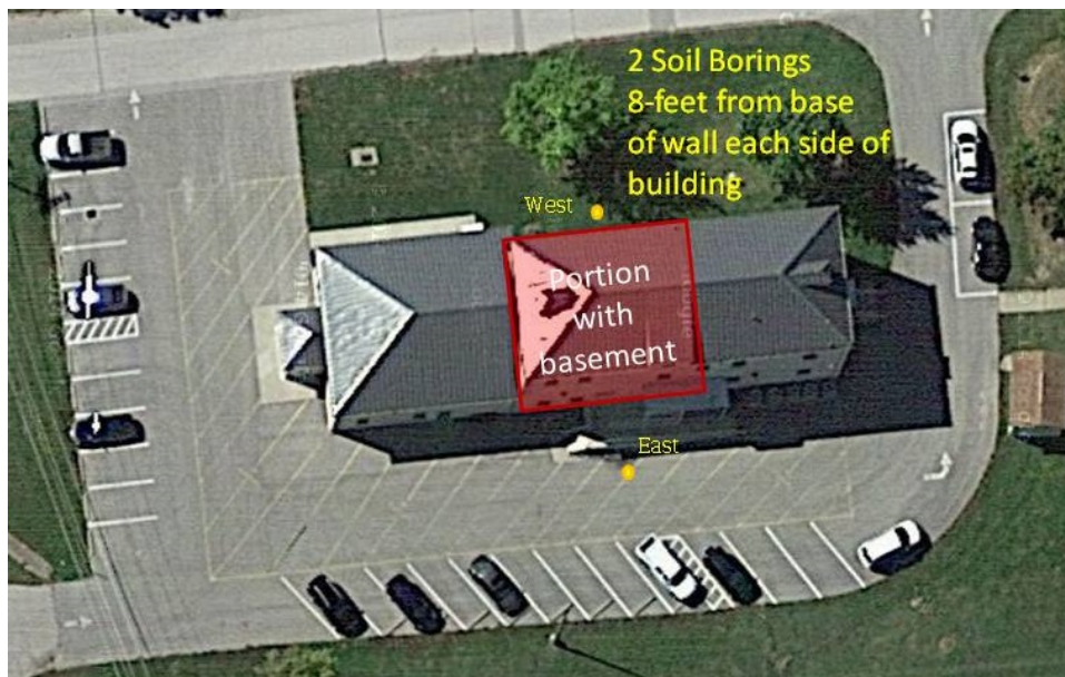
Figure B1. Satellite view showing where soil samples were taken and piezometers were installed at BGAD.
