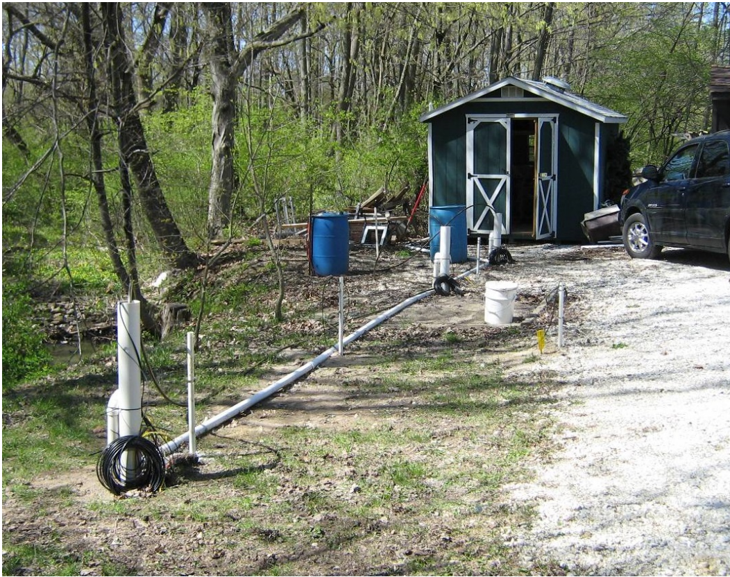
Figure A3. Photograph of ISWEOD pilot site showing piezometer (PZ-5) 18 in. from Well 3 (foreground).
