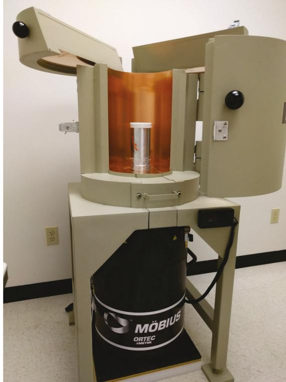
Figure 5. The gamma spectroscopy system operated at the ERDC. This system utilizes a 70 mm planar germanium detector, an ultra-low background Pb shield, and a liquid nitrogen recycling system allowing for continuous, high-resolution analysis of low-activity samples.
