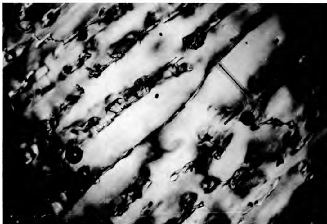
Figure 7. Thin section of a crystal of sea ice showing individual brine pockets interspersed between the ice plates. The spacing between successive layers of brine pockets (also called plate spacing) is about 0.6 mm. The c-axis direction (arrow) is normal to the platy substructure.
