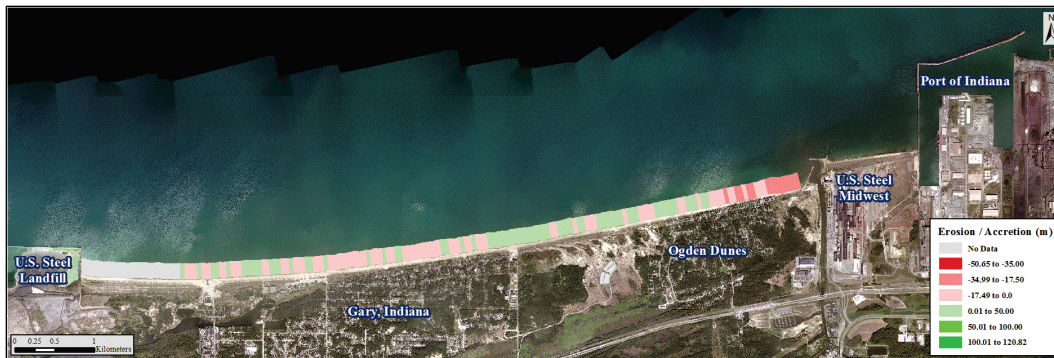
Figure 3. Shoreline change from the Port of Indiana to the U.S. Steel Landfill from 1969 to 1973.
