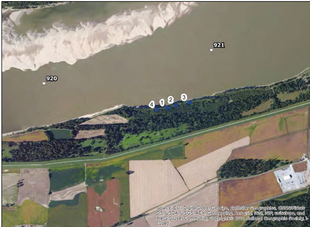
Figure 19. 2013 roto sonic borings at the Hickman scour pool area.
