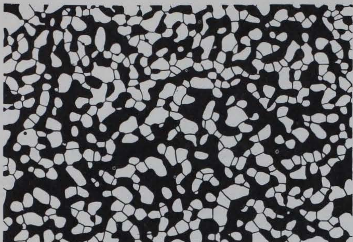
Figure 8a. Thin section of 10-yr-old névé. Density 0.5 \text{ g/cm}^3 . Pore area is black. Magnification 3.8x . (From Fuchs, ref. 13).
