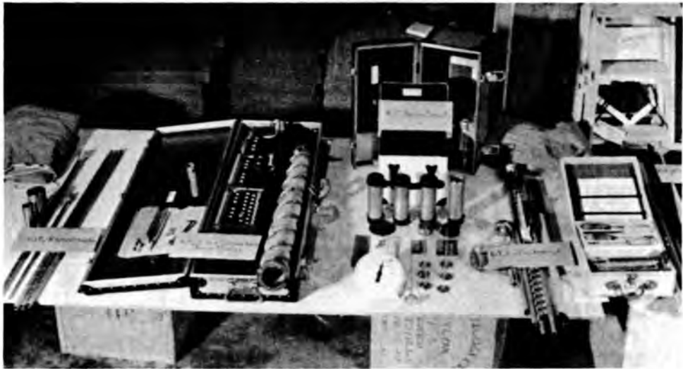
Figure XI-4. CRREL (formerly SIPRE) test kits. The items are, from left to right: Rammsonde kit (see Fig. XI-5). 3-in. ice coring auger kit (comprising 1 m long core barrel, coring head with removable bits, core barrel connector, brace and T-bar, extension rod adapters and connecting pins, spare cutting bits and small tools for removing and sharpening bits. The box containing 1 m long extension rods is not shown). Snow density kit (see Fig. XI-6). Ice thickness kit (see Fig. XI-7). Salinity kit (comprising four hydrometers calibrated in salinity units at 15C, and covering the range 0-40‰; flotation cylinder with thermometer; temperature correction chart).
