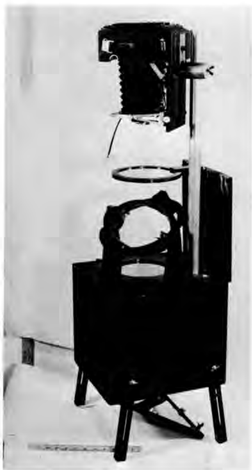
Figure XI-11. Four-axis universal stage with camera. (Photo from Langway, ref. 23)
