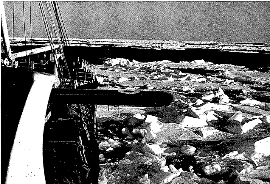
(a) Open pack ice. The floes are well separated by open water, and ice-strengthened ships can move freely. Some evidence of old rafting can be seen in the foreground.
