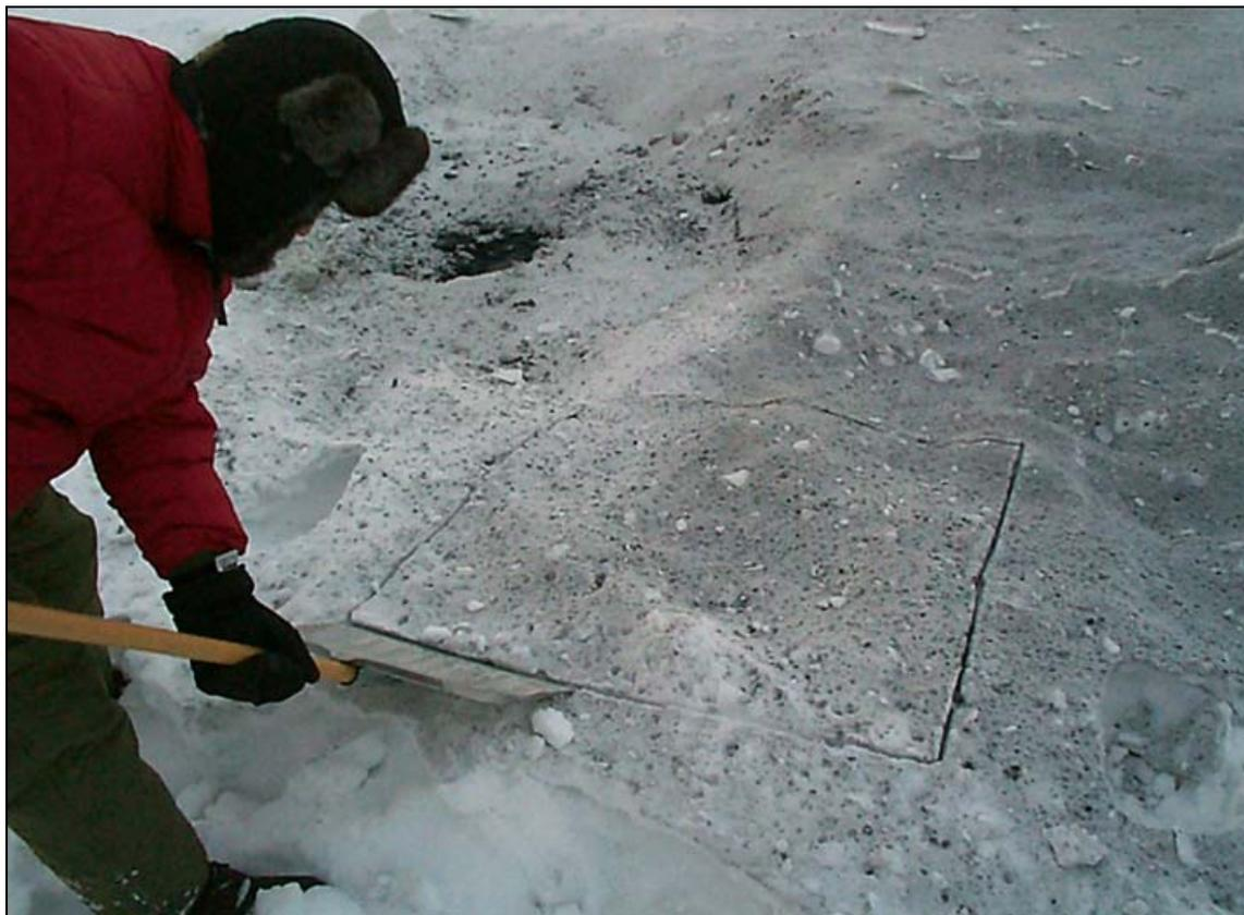
**Figure 7. Sampling a 1-m<sup>2</sup> area of snow next to a detonation point.**
