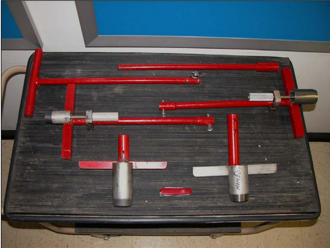
**Figure 1. CRREL coring tools for cohesive soils.**
