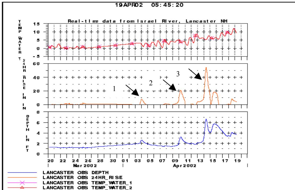
Figure 4. Lancaster Web page interface, showing three events. The first event did not exceed alarm thresholds and did not result in flooding. The second and third events did trigger alarms.
