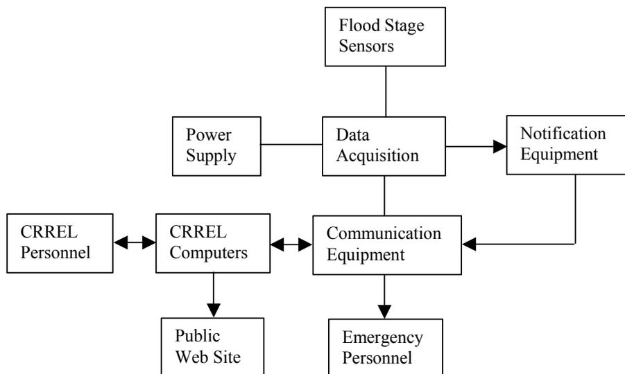
Figure 1. Simple early warning flood stage system tested at CRREL.
