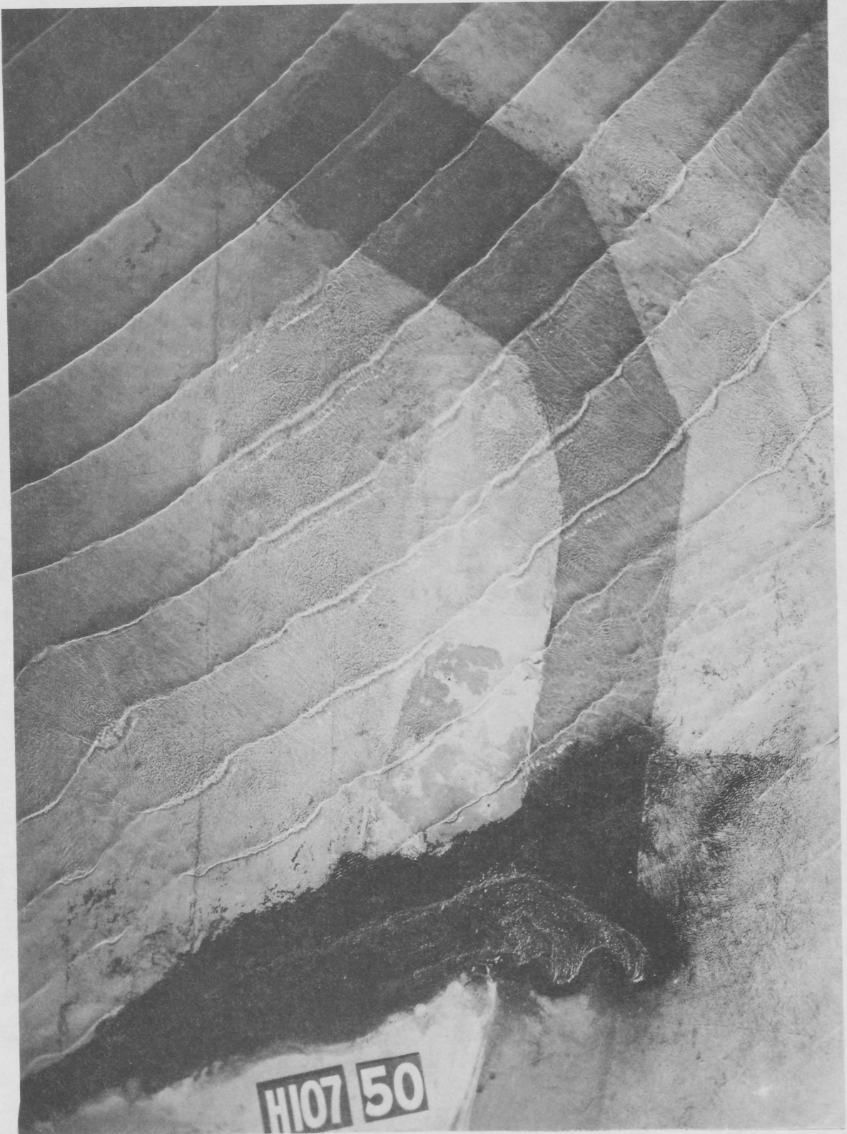
Figure 5-6. Typical shoaling pattern at Cattaraugus Creek for existing conditions.
