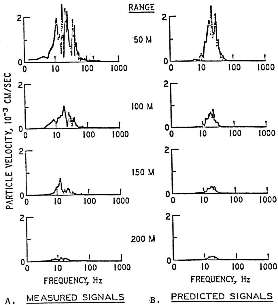
Figure A5. M-151 (jeep) signals, 32 km/hr,
