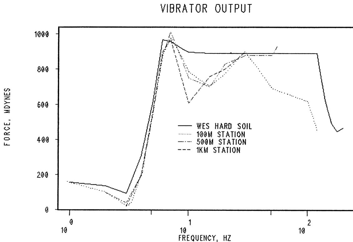
Figure 2. WES electrohydraulic vibrator output for calibration tests at WES and at each test site
