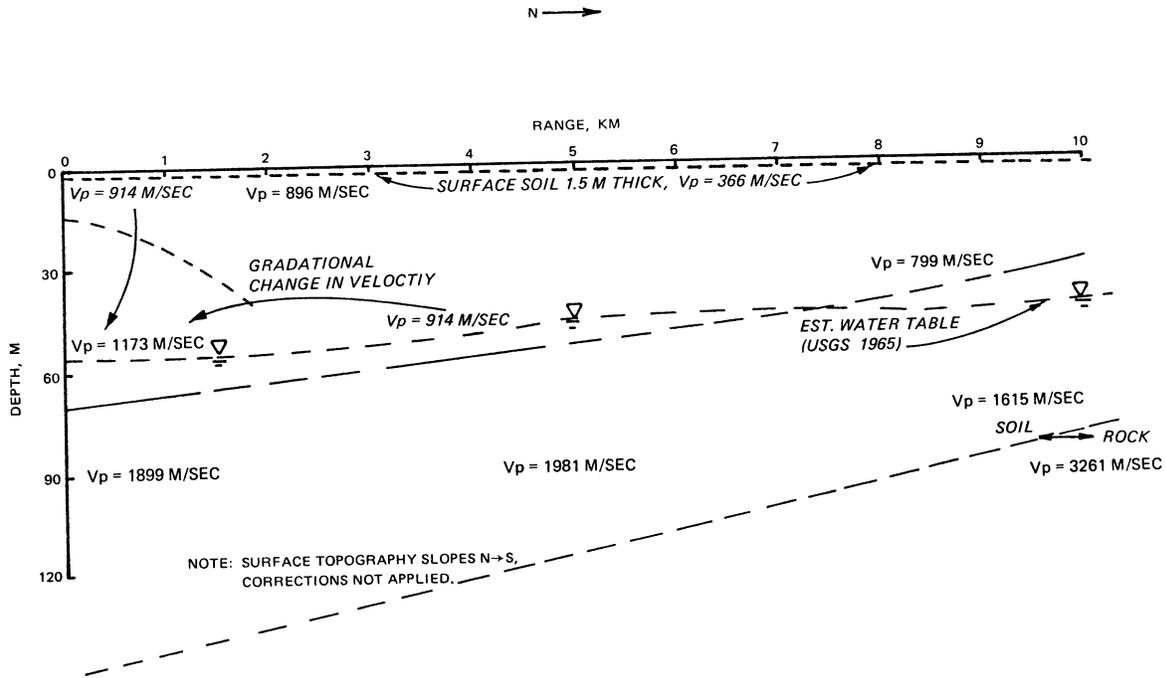
Figure B19. Seismic profile of test site
