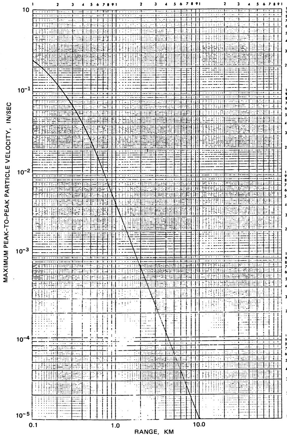
Figure B17. Maximum peak-to-peak particle velocity attenuation versus range
