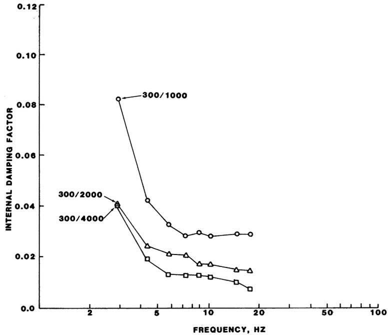
Figure 34. Internal damping factor versus frequency calculated from attenuation ratio for explosive-source test data. Numbers indicate locations of compared data.
