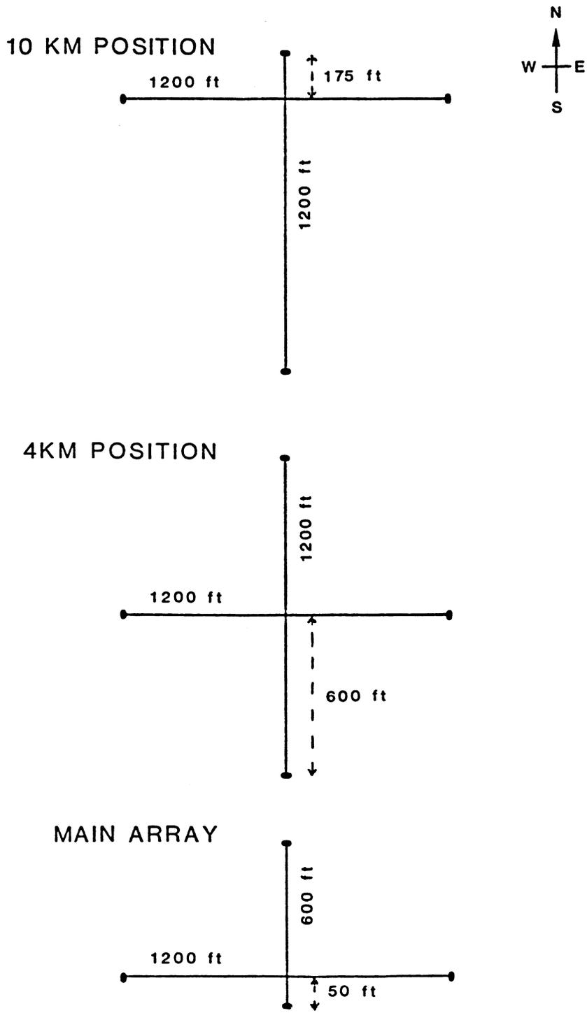
Figure B2. Seismic refraction survey line layout
