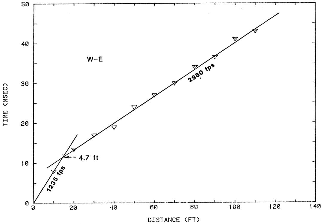
Figure B3. Main array, overburden test
