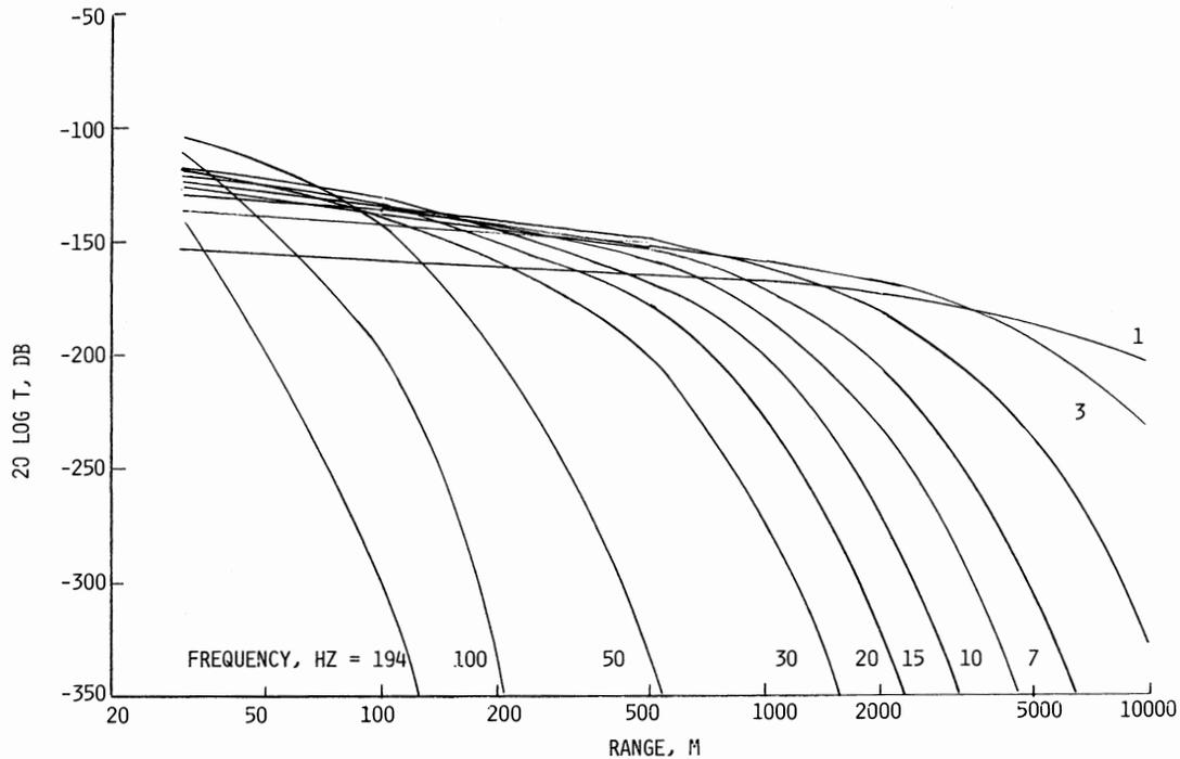
Figure 23. Transfer function T versus range predicted by model
