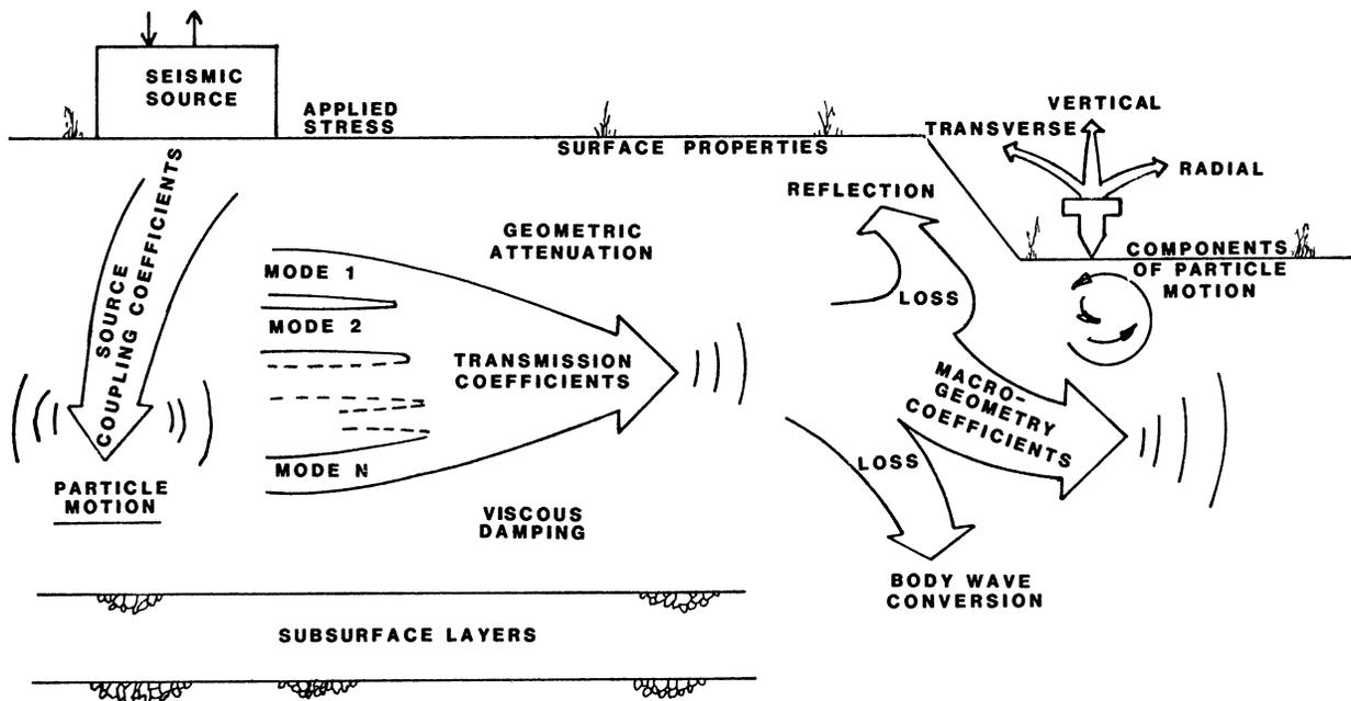
Figure 16. Properties of seismic attenuation
