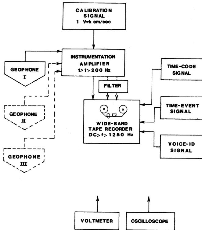
Figure 6. Schematic of typical analog recording system
