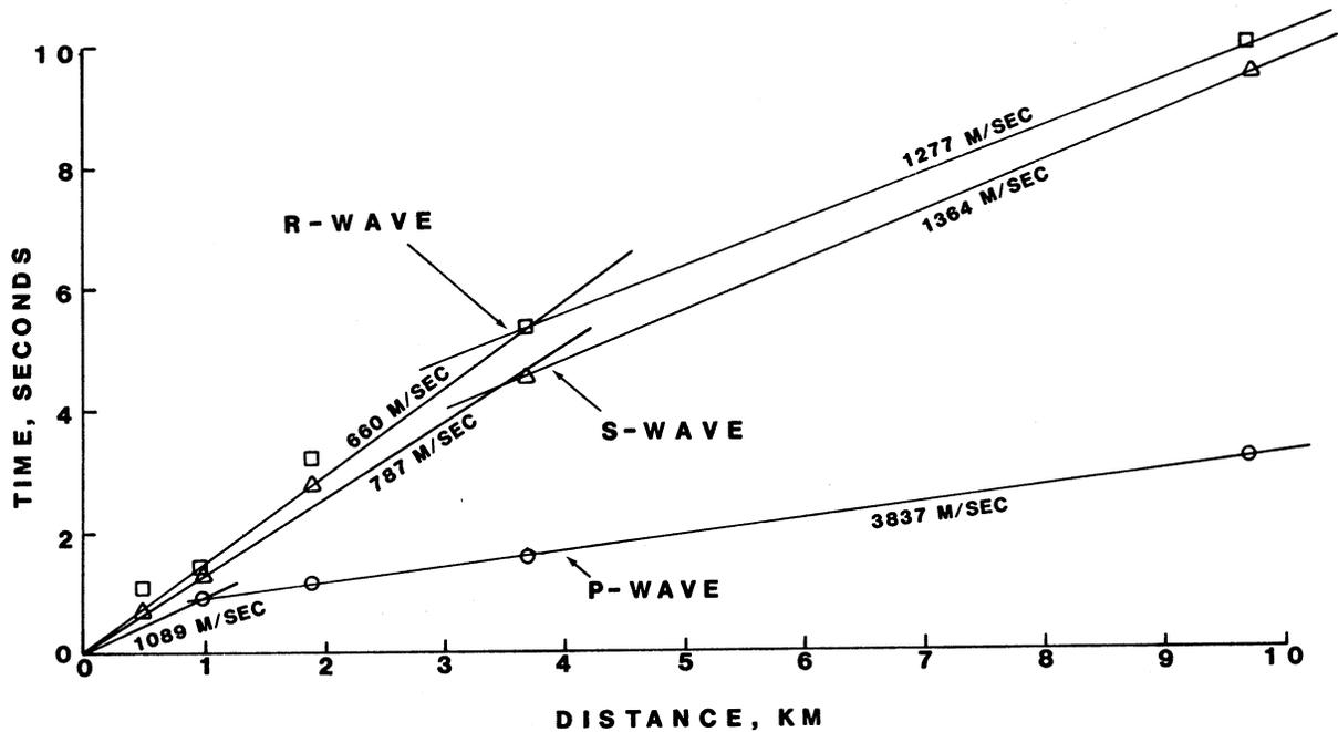
Figure 17. Time versus distance plots for explosive-source tests
