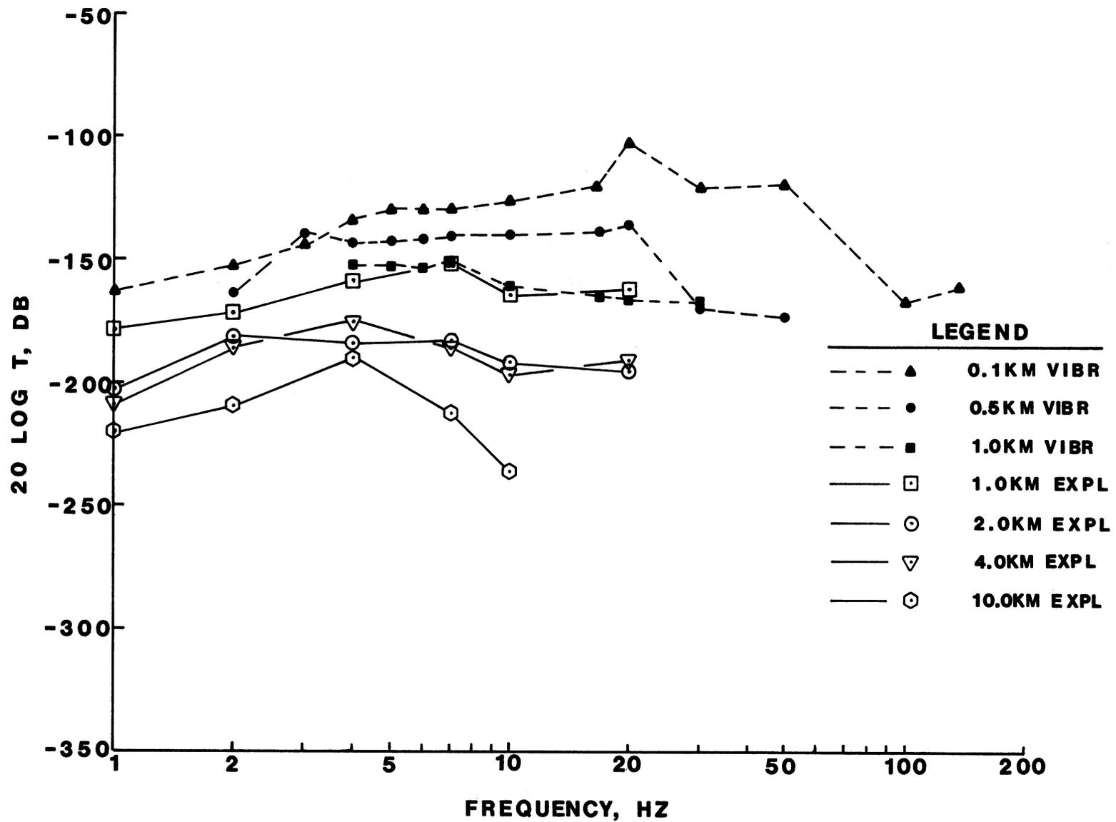
Figure 36. Transfer function  $T$  versus frequency calculated for discrete frequency vibration tests (top three curves) and for explosive-source tests
