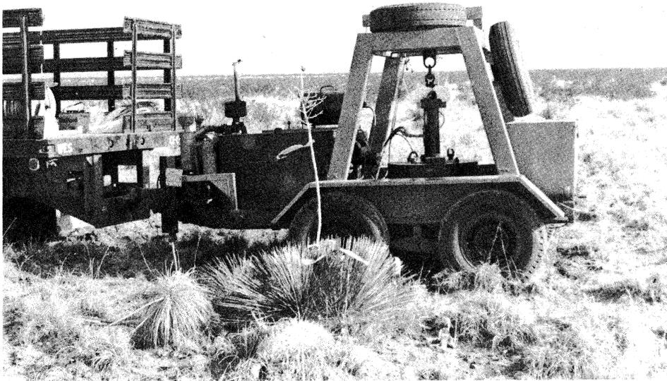
Figure 1. WES electrohydraulic vibrator
