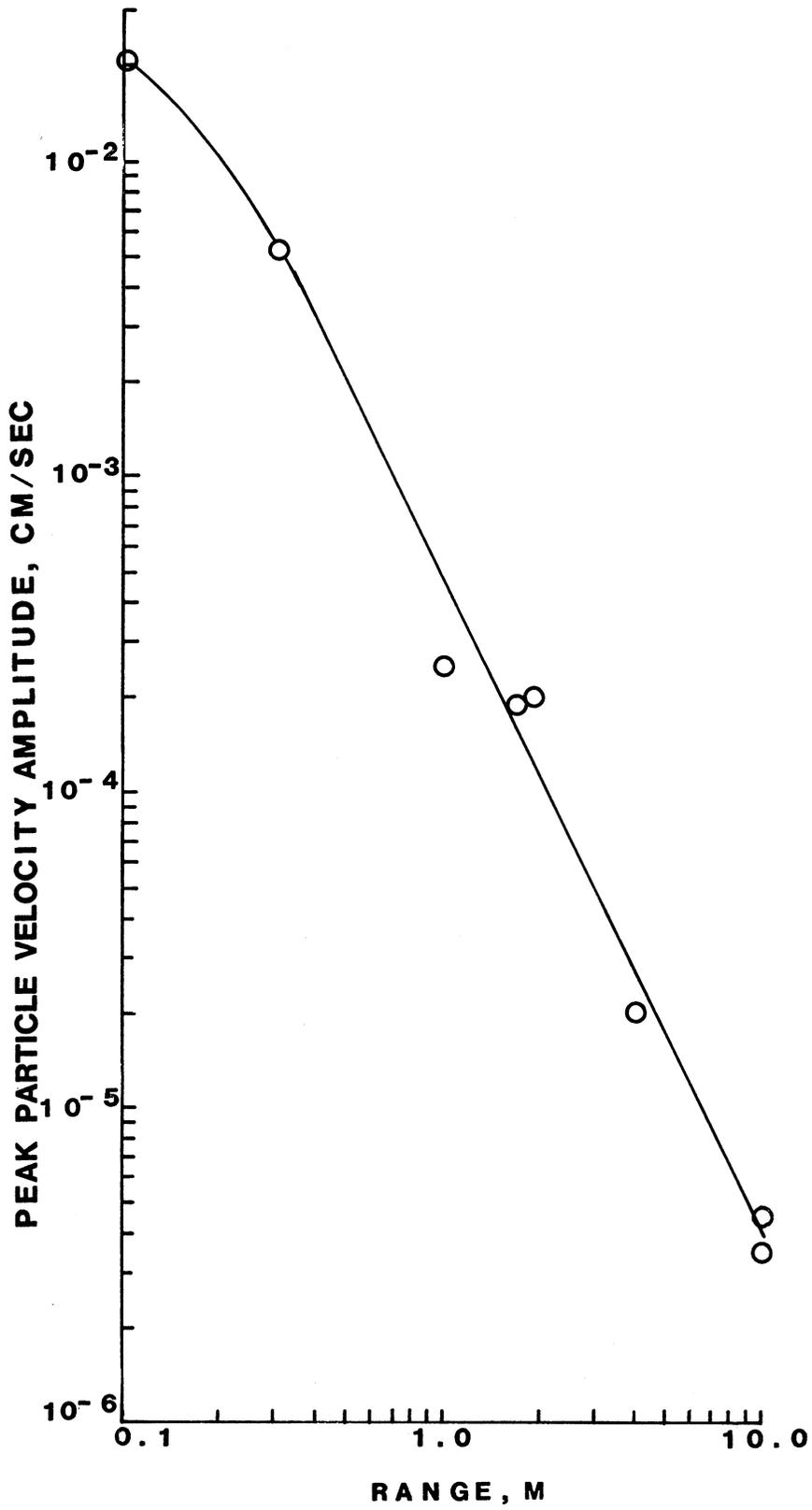
Figure 18. Attenuation curve generated from explosive-source test data
