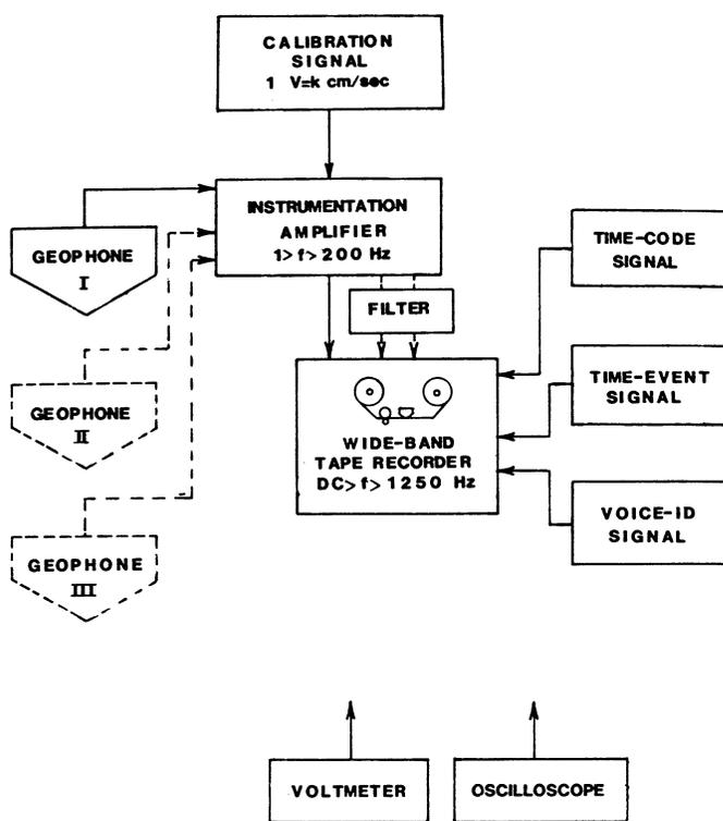
Figure A2. Block diagram of the major components in a typical seismic analog recording system
