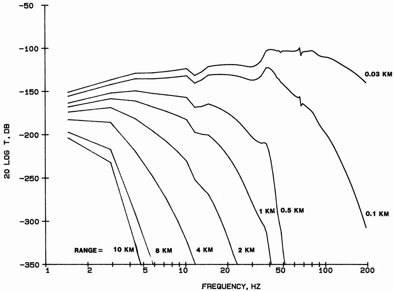
Figure 22. Transfer function  $T$  versus frequency predicted by model
