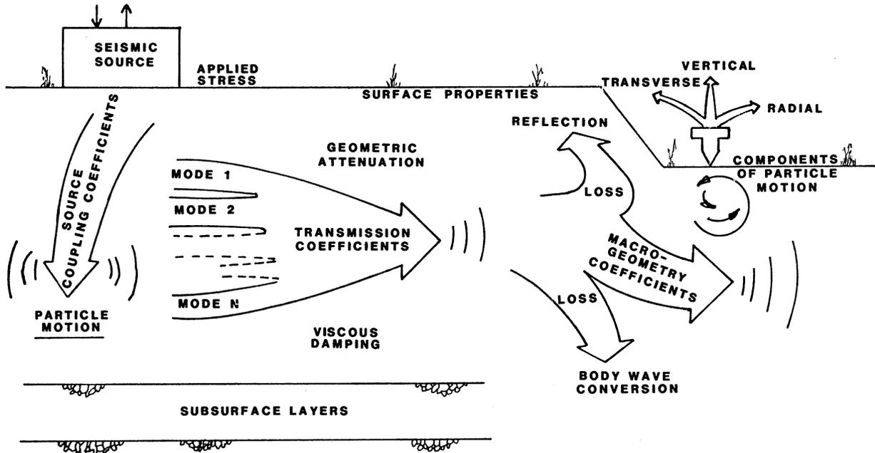
Figure A3. Seismic wave propagation
