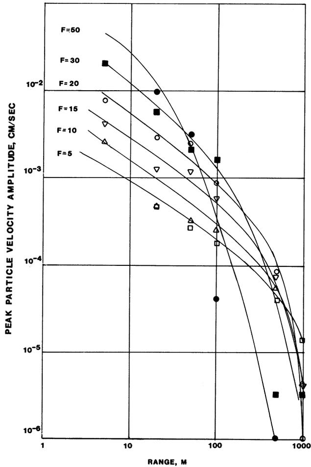
Figure 19. Attenuation curves for discrete frequency vibration tests
