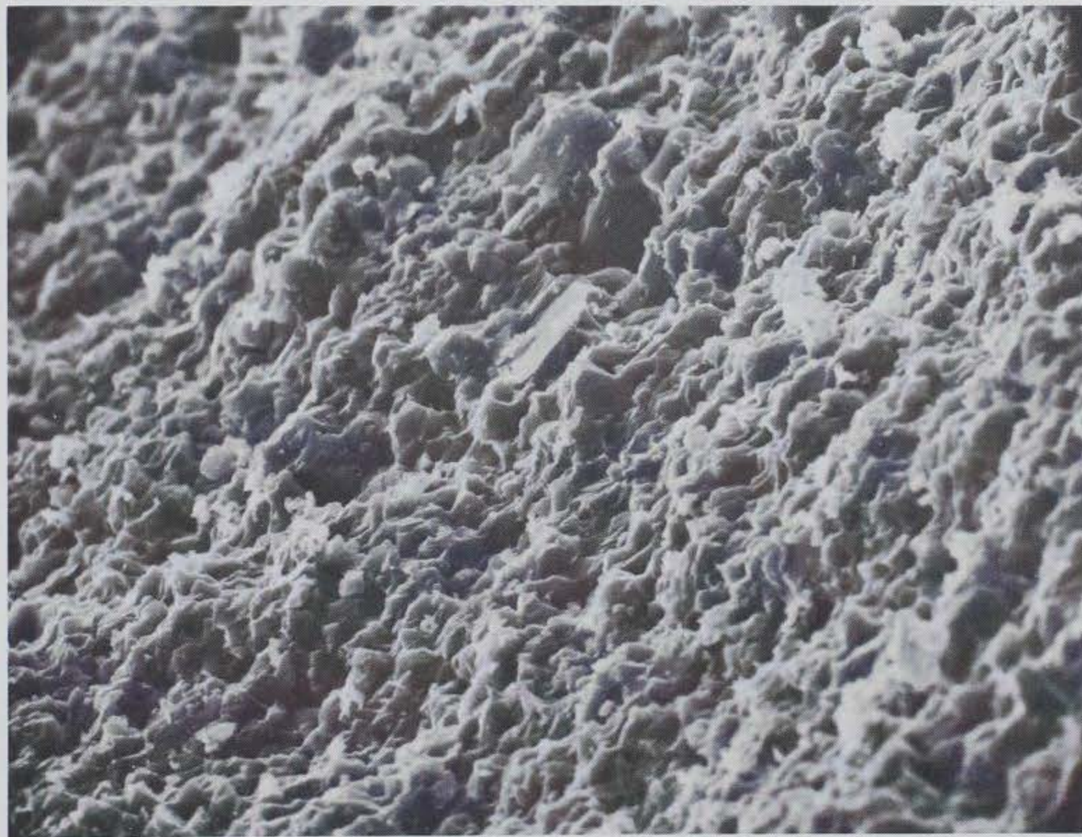
b. Hermitage rock from 34-month-old concrete bar 6-8, \times 1000 (010472-11)
