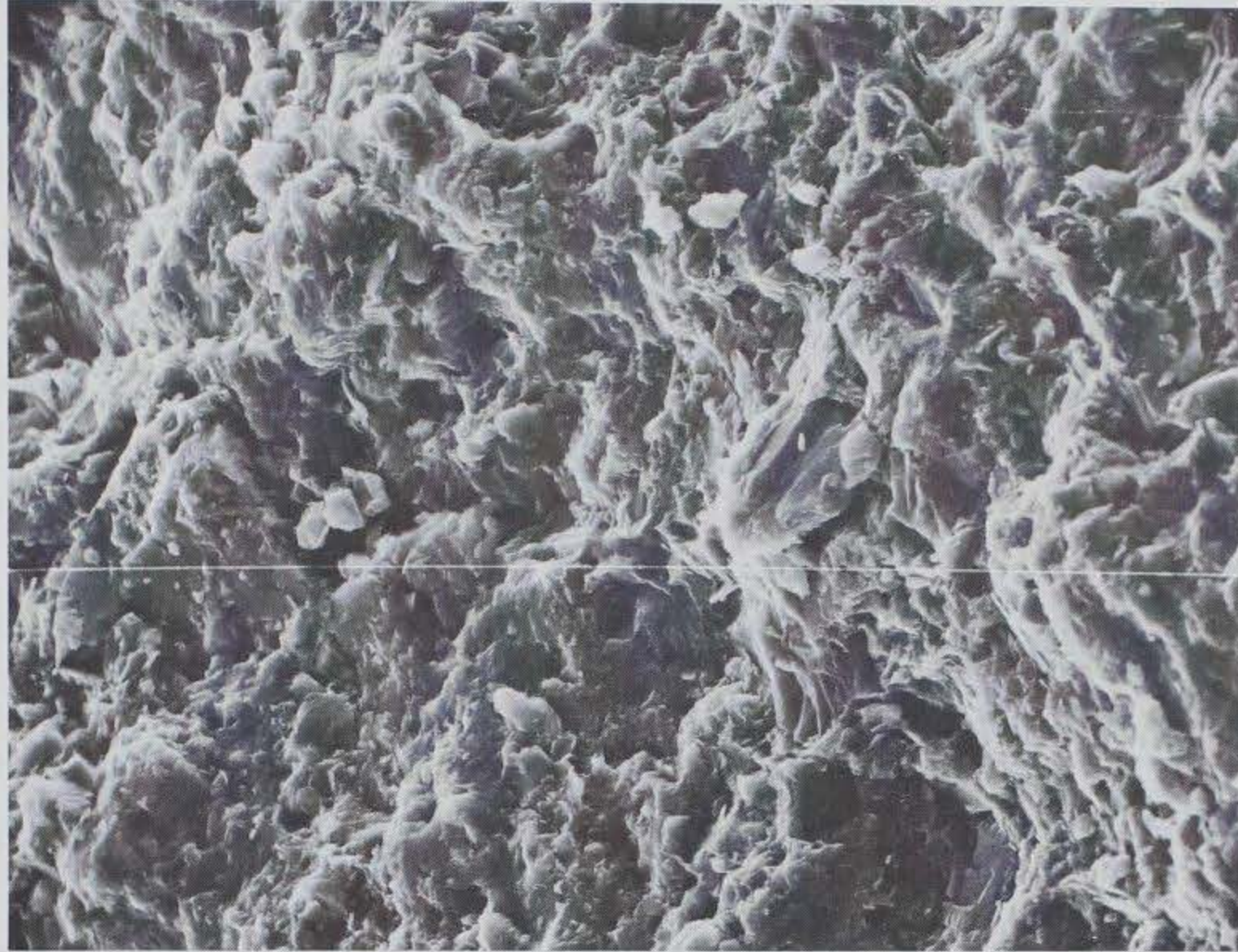
a. Unreacted 1-8 rock, \times 1000 (010472-5)
