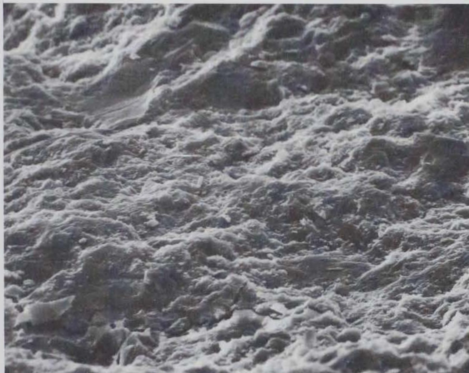
c. Fresh fracture surface of 34-month-old RC-167 cement paste about 1 in. away from surface of 1-8 slab 2, \times 1000 . Should be out of reaction zone (010572-11)
