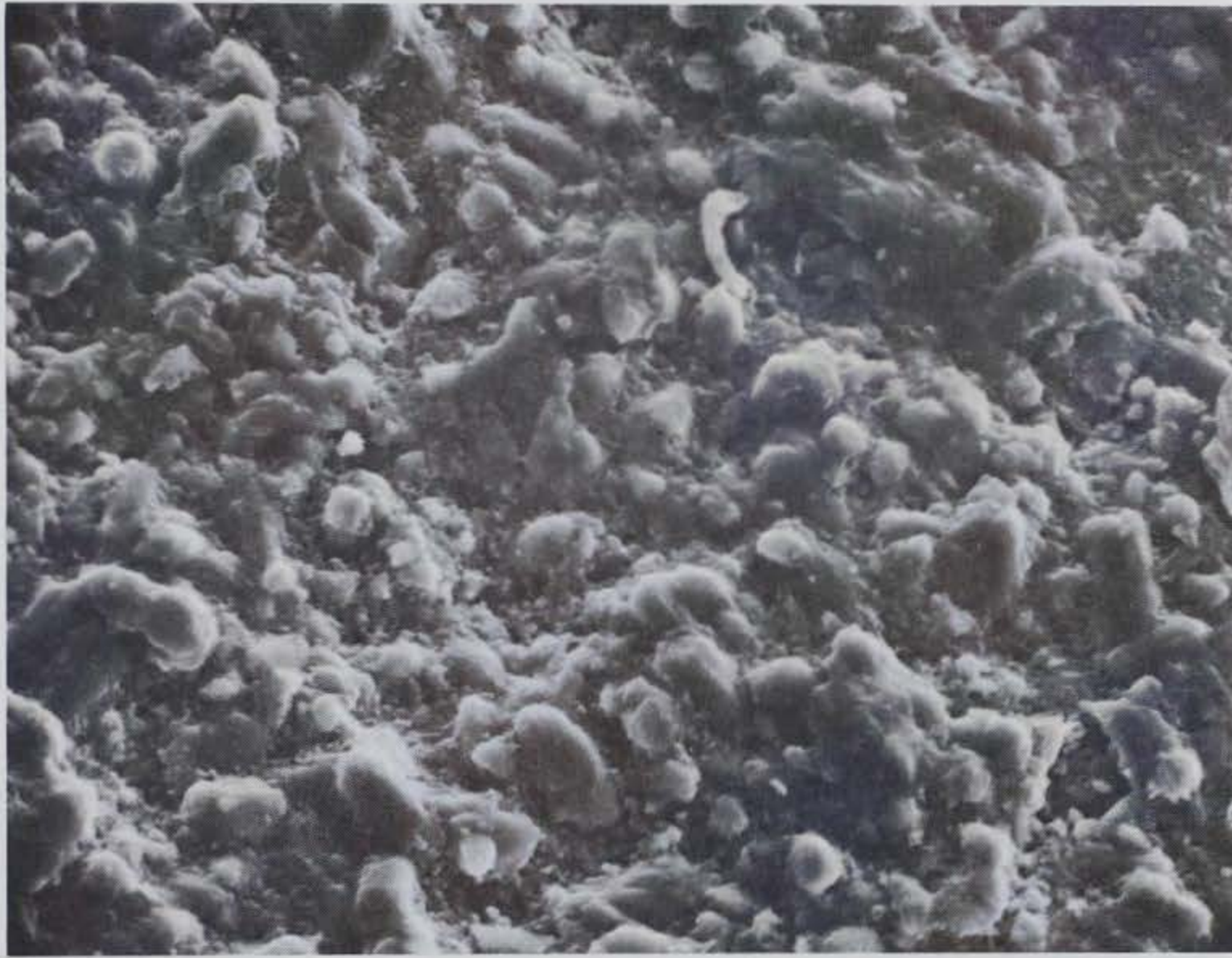
c. Reacted 1-8 slab 3 after 19 months in 1 N NaOH solution, \times 1000 (010472-23)
