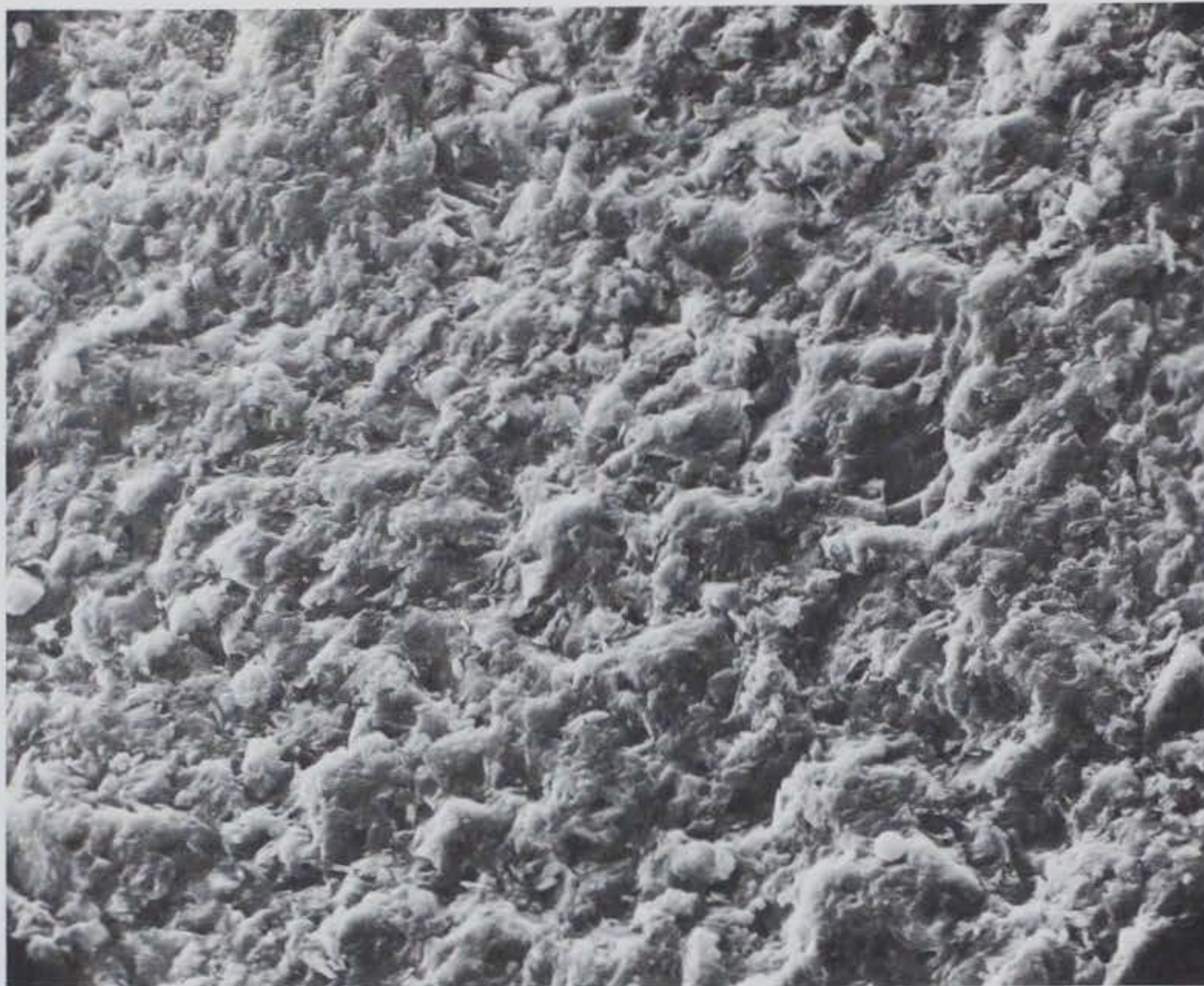
a. Unreacted 1-8 rock, \times 1000 (010472-8)
