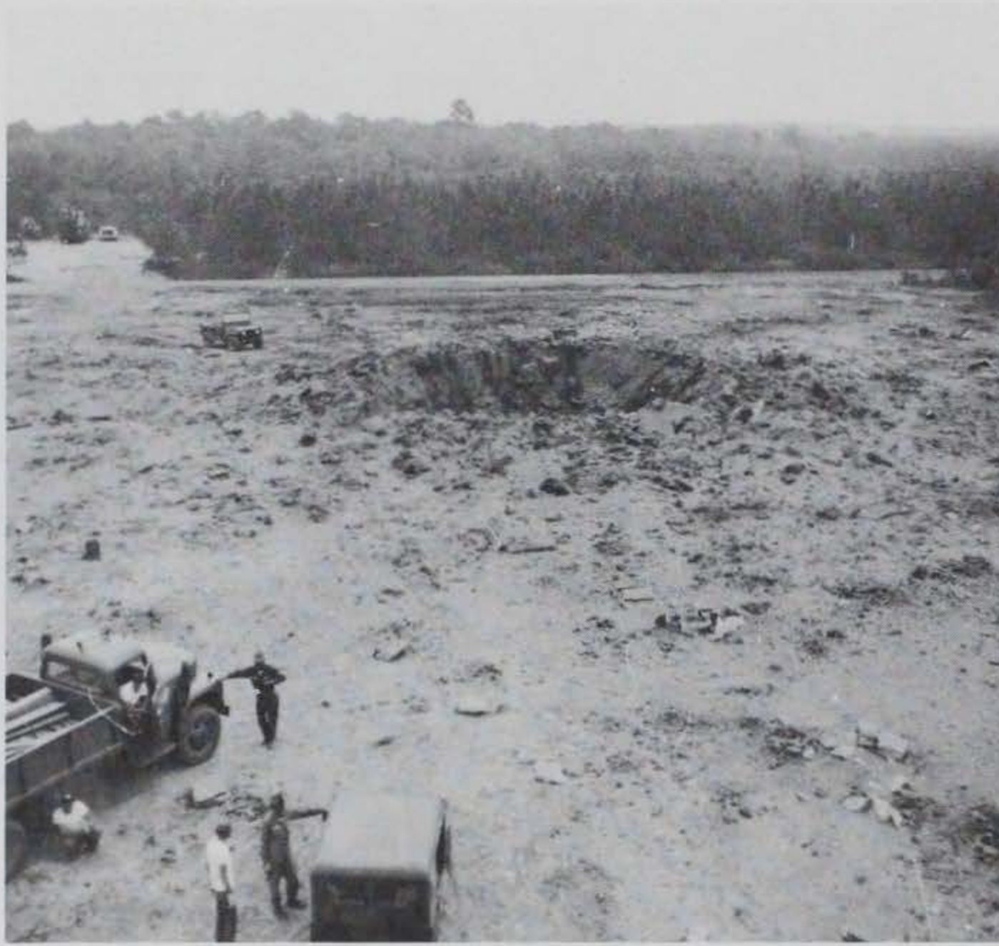
Figure 1.5 Crater and debris from a 750-pound bomb explosion.
