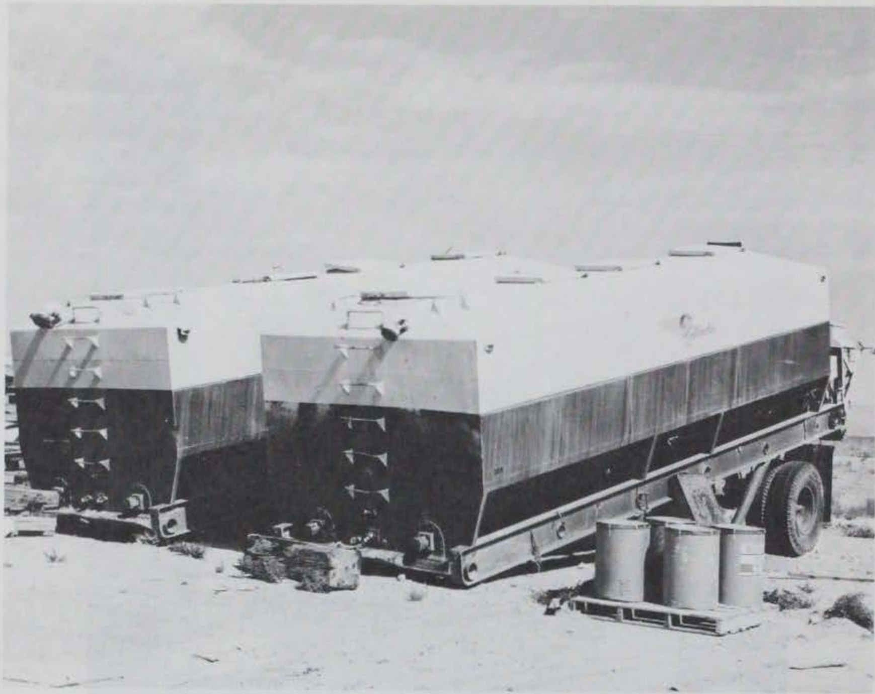
Figure 4.3 900-ft 3 mobile storage tanks.
