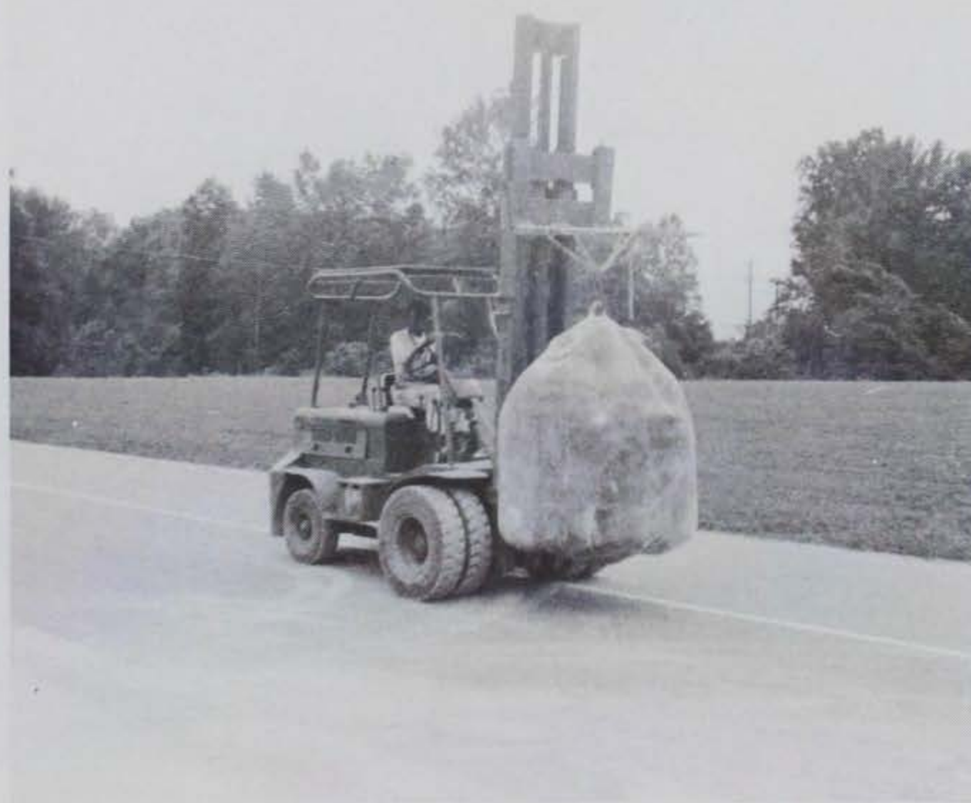
Figure 4.2 Rubberized storage bag for cement.
