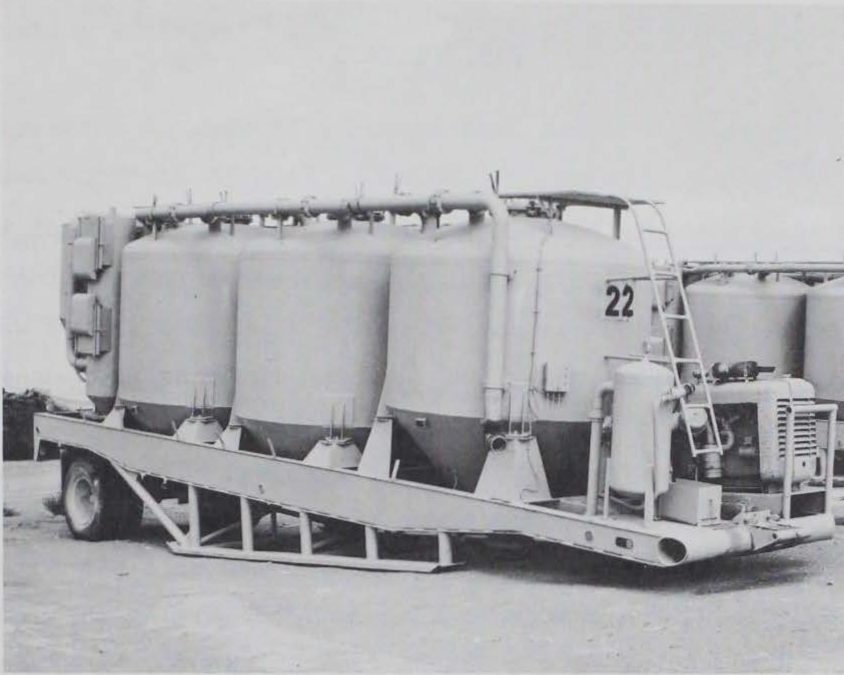
Figure 4.5 750-ft 3 field storage tank.
