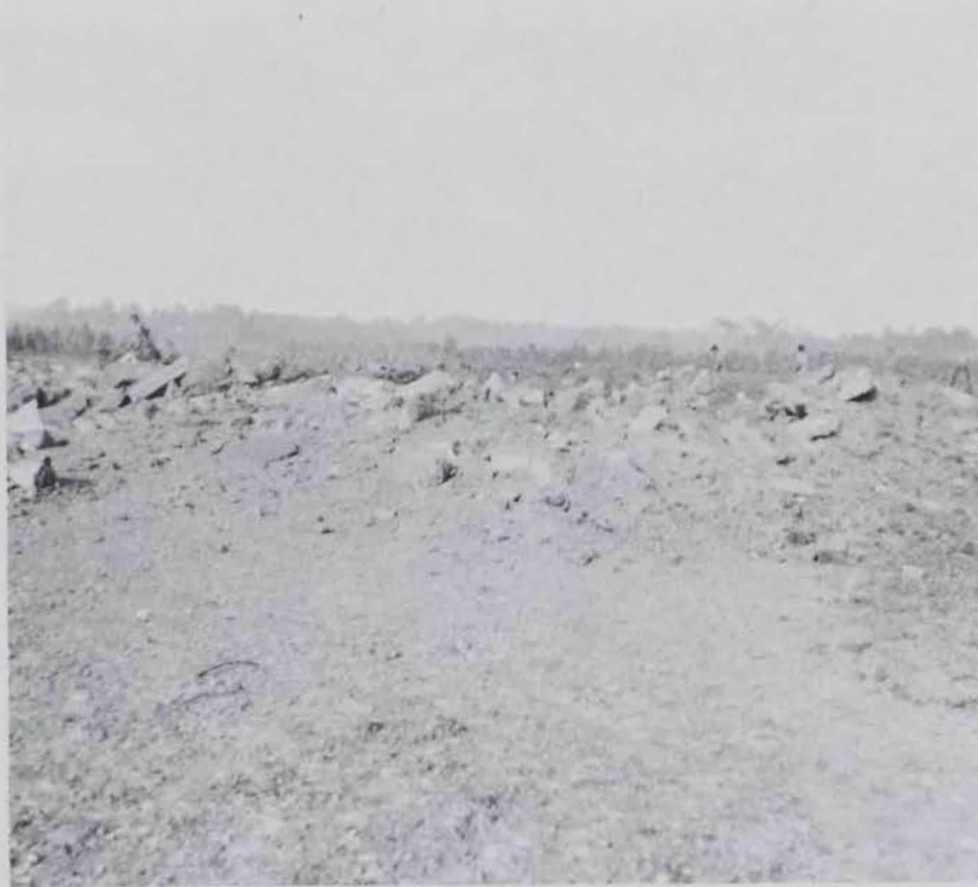
Figure 1.7 Debris on crater lip.
