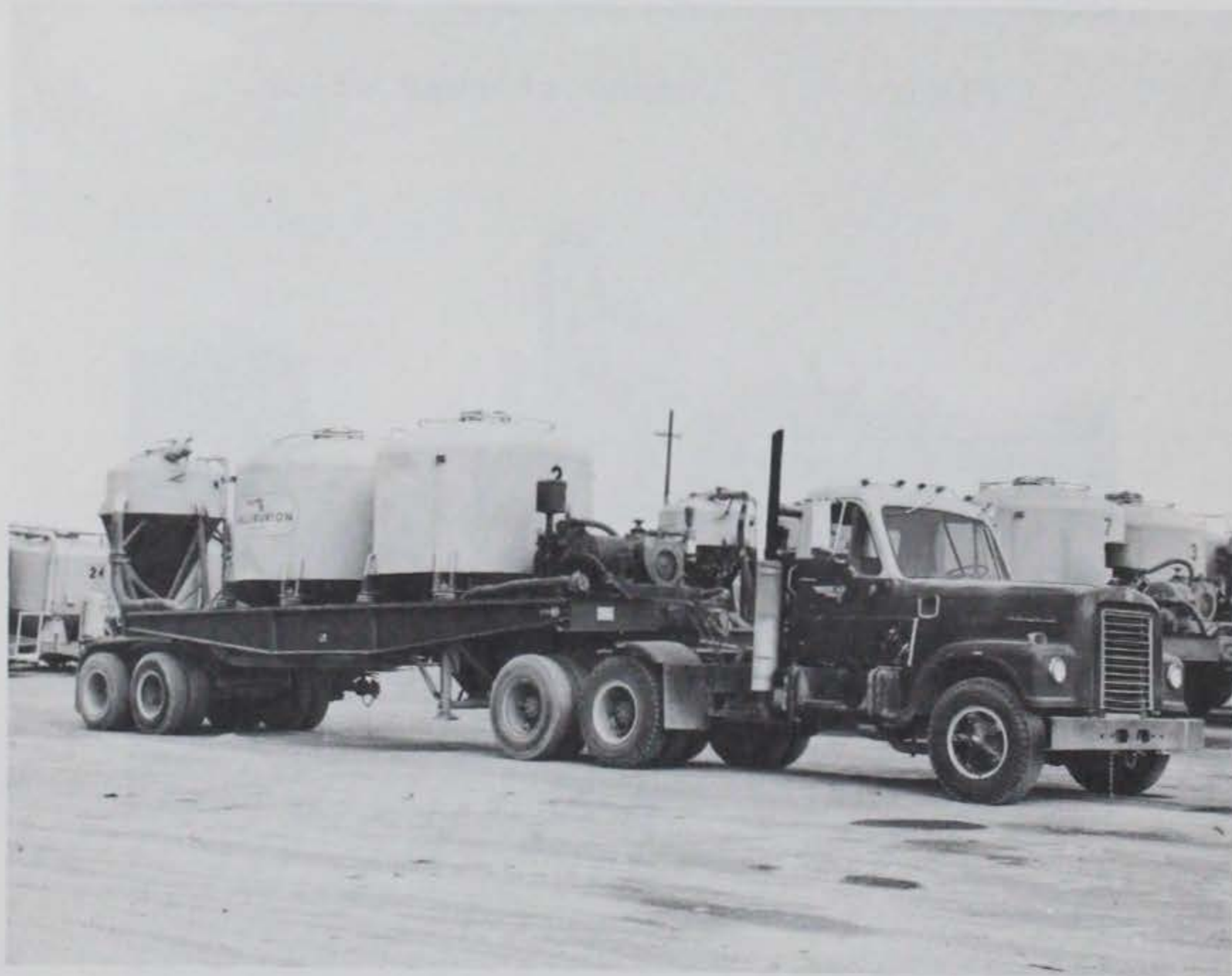
Figure 4.4 500-ft 3 pneumatic bulk tanks.
