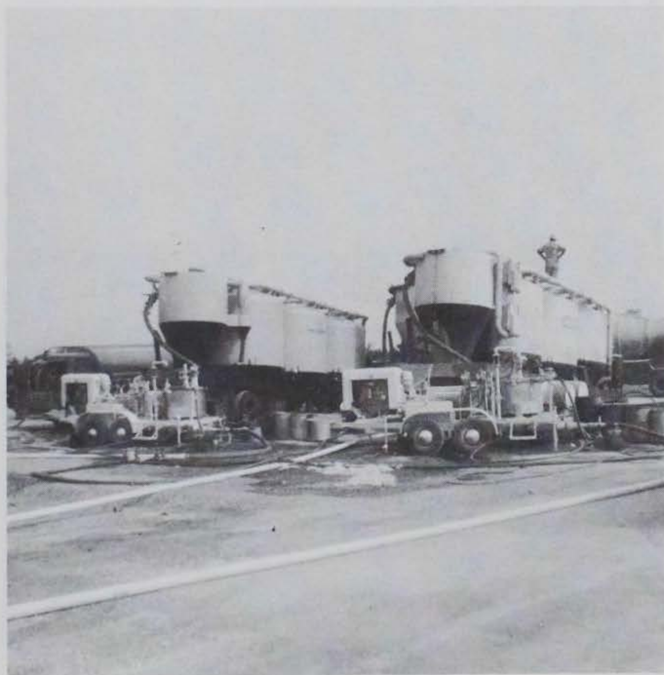
Figure 5.34 Mobile field storage tanks.
