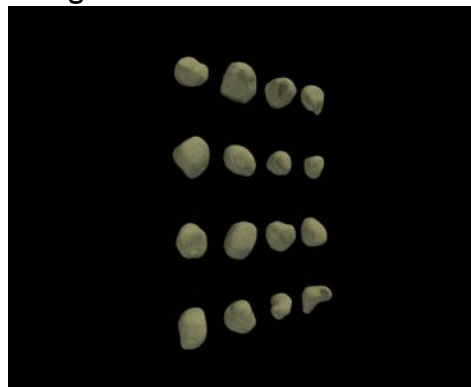
(b) Sample of several particle geometries generated from microCT scans.
