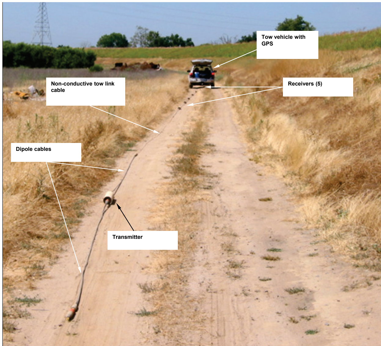
Figure 6-9. Illustration of the Geometrics OhmMapper capacitively-coupled resistivity system being vehicle-towed along a levee toe.
