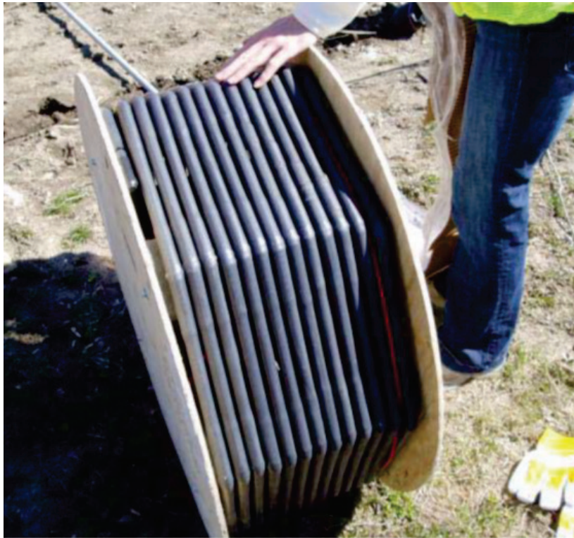
Figure 5-24. SAA/MEMS inclinometer string on shipping wheel (Barendse 2012).
