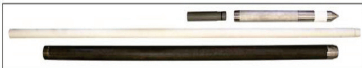
Figure 5-44. Push-in open standpipe piezometer (RST Instruments 2013).
