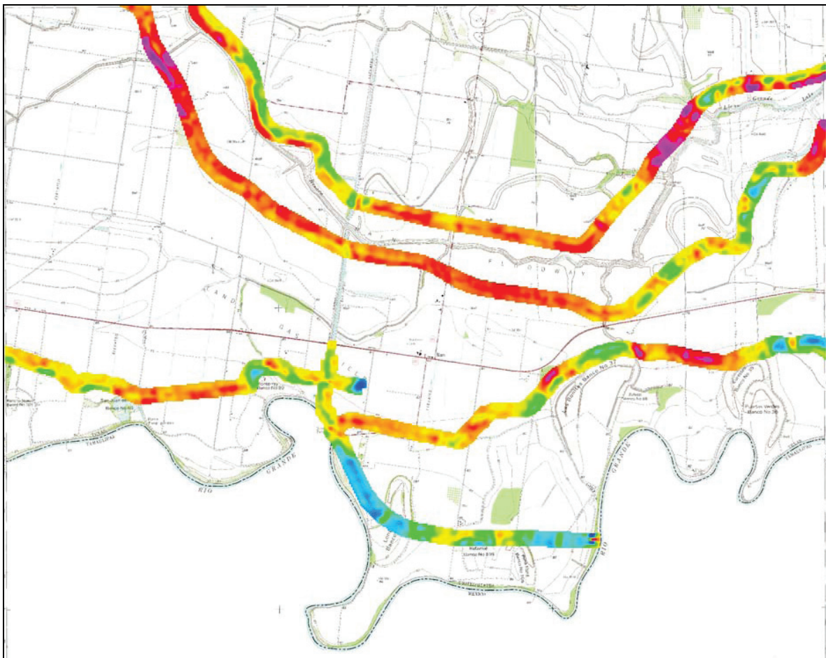
Figure 2-7. Example conductivity map in millisemens/meter from helicopter EM survey of Rio Grande levees created by three survey transects along the levee right-of-way (center line and both levee toes with spacing of 50 m between transects).
