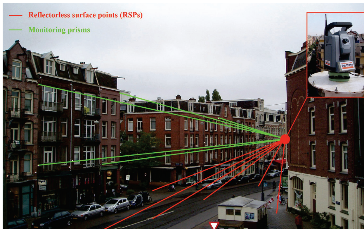
Figure 5-3. Example of remote monitoring of surface deformation using a robotic total station mounted to a building (Tamagnan and Beth 2012).
