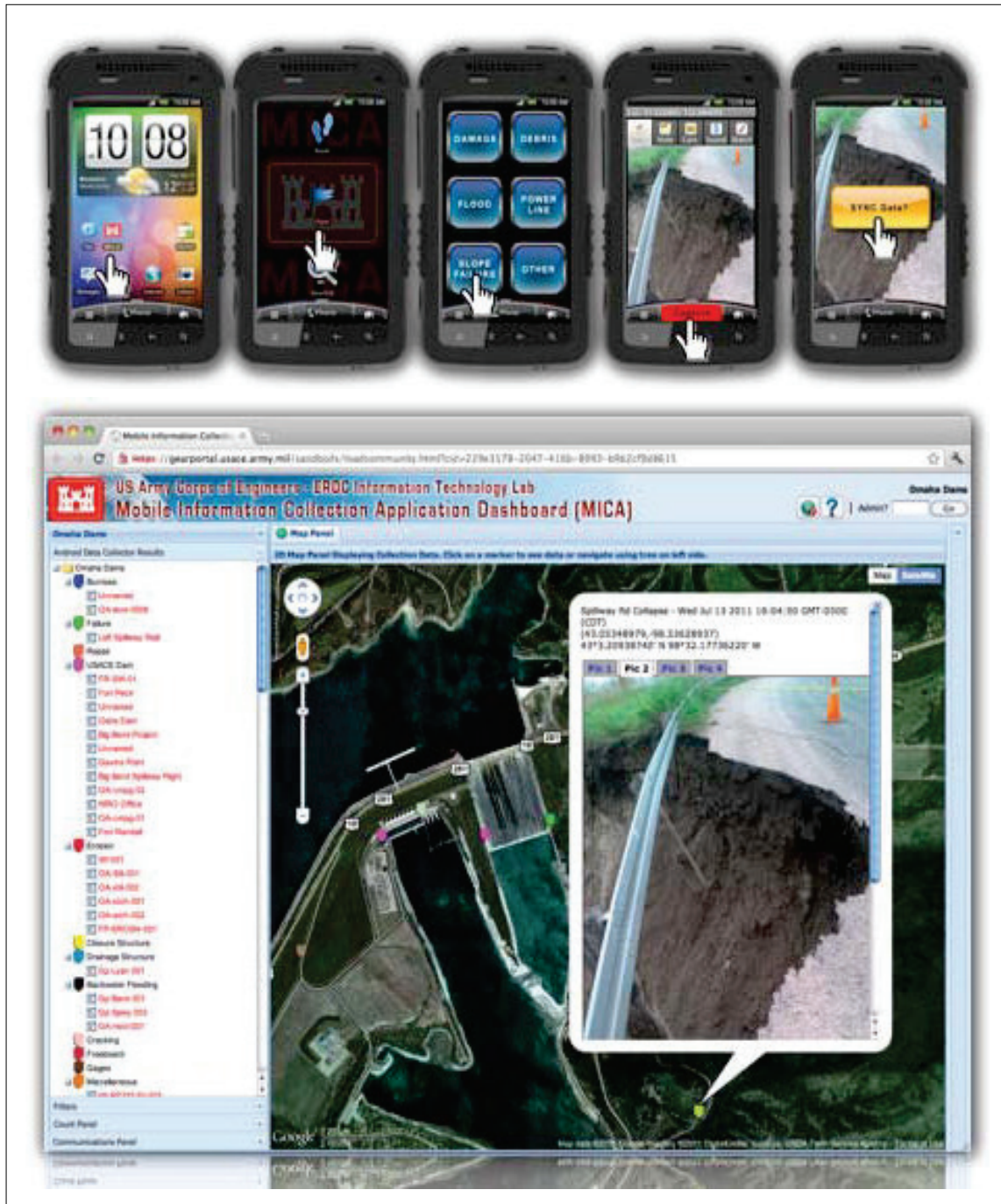
Figure 4-4. MICA Android phone application for reporting seepage incidents to command centers during the May 2011 Mississippi River Flood (USACE 2011b). Example problem area shown in Figure 4-3 and 4.5. The phone app permits communication of written information and integration of GPS imagery to decision-makers.
