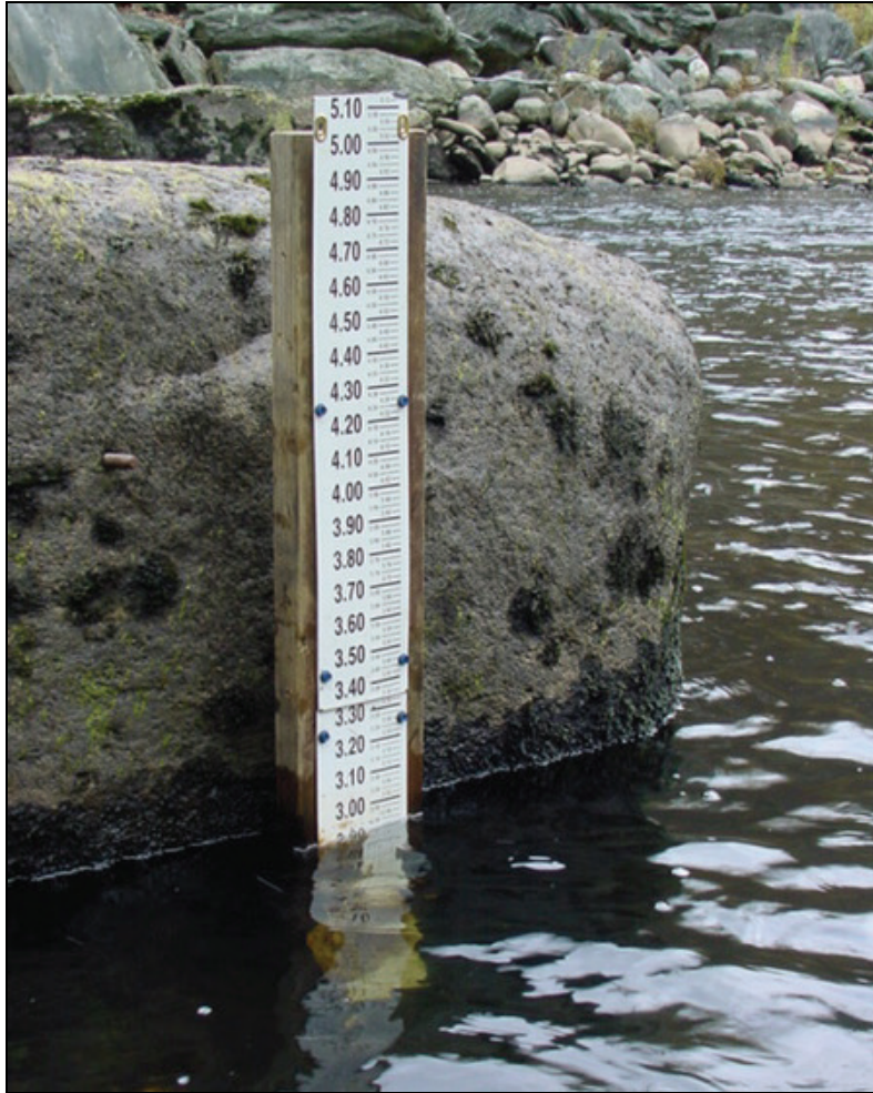
Figure 5-47. Staff gage to measure water levels (USGS 2013).
