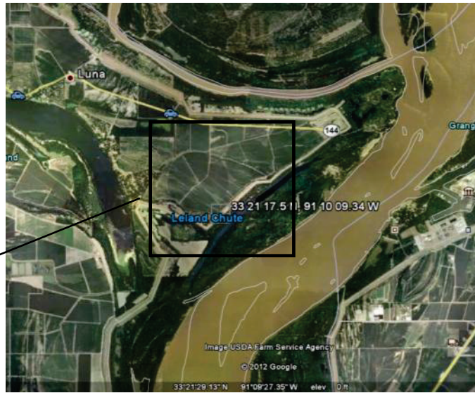
Figure 4-3. View looking southwest (downstream) during the May 2011 Mississippi River Flood north of Lake Chicot, AR (Eric Woerner, personal communication, Vicksburg District 2012). Light to moderate seepage (see Table 3-1) collecting in the low lying point bar swales. These swales developed as ends of Lake Chicot converged to form an abandoned channel or oxbow of the Mississippi River. The tree line at landside levee toe was site of numerous sand boils (see Figure 4-5 for view of the LiDAR data).
