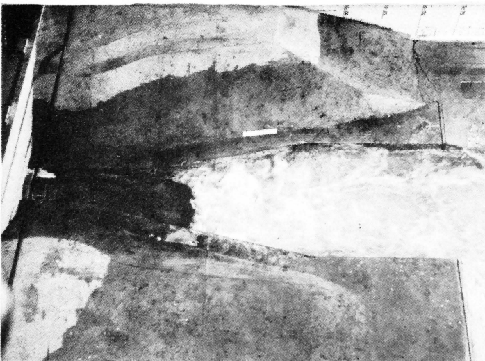
Photograph 42. Basic design H.W. = 381.3 T.W. = 350.0 Q = 14,550 c.f.s.
