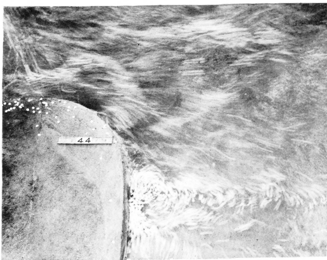
Photograph 53. View showing eddy at rounded wing wall. Radius at top of wall = 30 ft.
