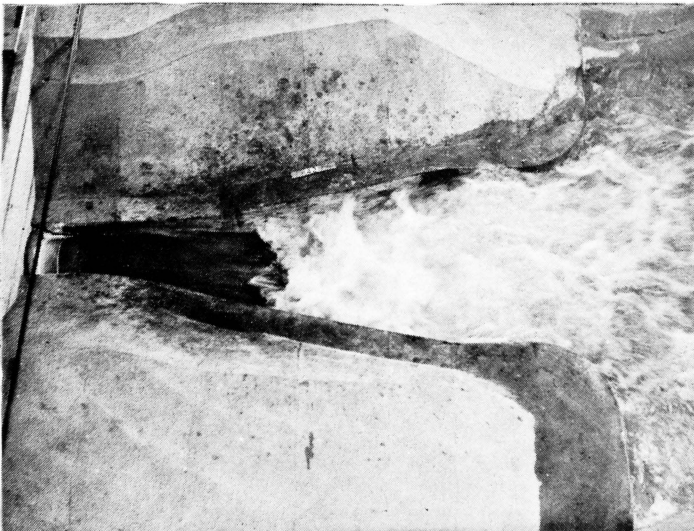
Photograph 51. Basin type DD. H.W. = 391.0 T.W. = 350.4 Q = 17,000 c.f.s.
