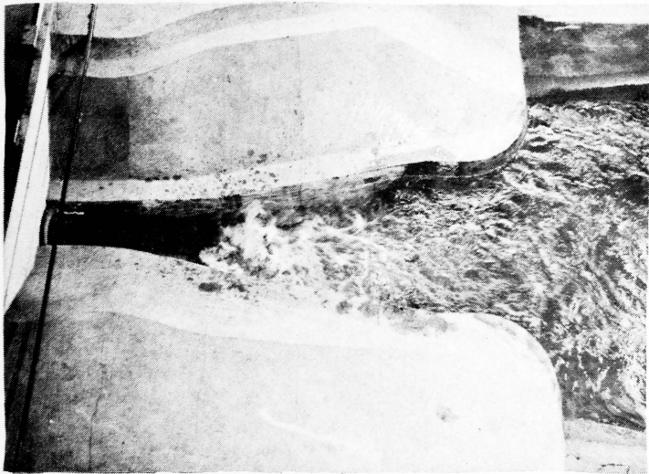
Photograph 58. Basin type GG. H.W. = 362.5 T.W. = 344.0 Q = 7,500 c.f.s.
