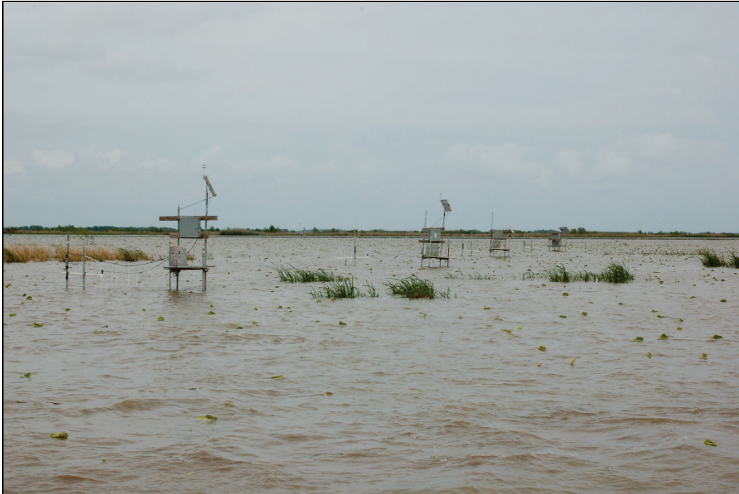
Figure 3. Mike Island stations looking eastward. Station 1 is the closest platform on the left. The photograph was taken in May 2014 before the emergence of Nelumbo lutea . The ADVs and wave gauges are mounted on the two poles at the left of each station.
