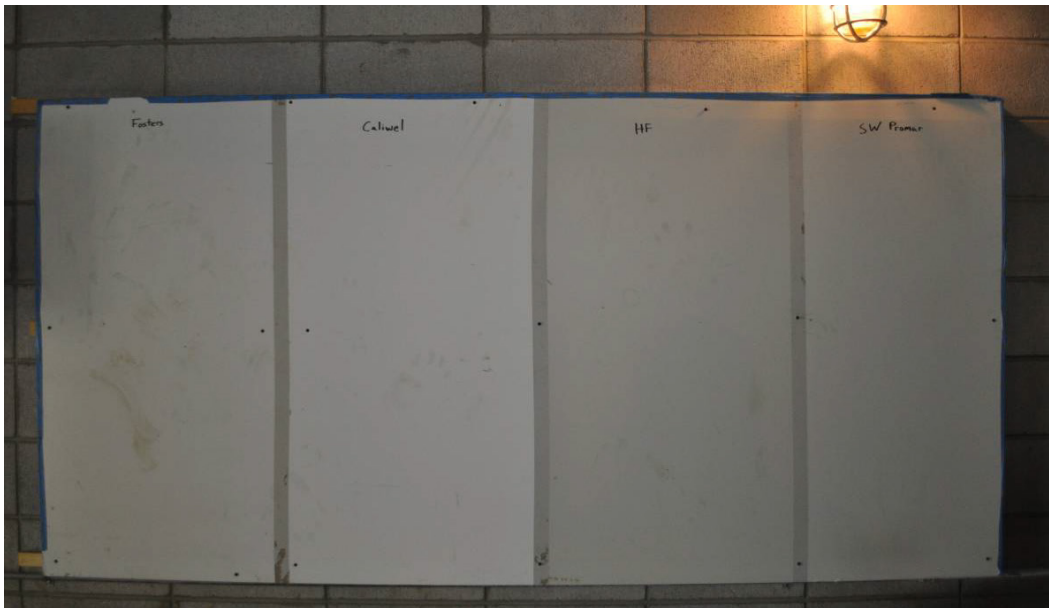
Figure 20. Test panels in the mechanical room after 8 months.
