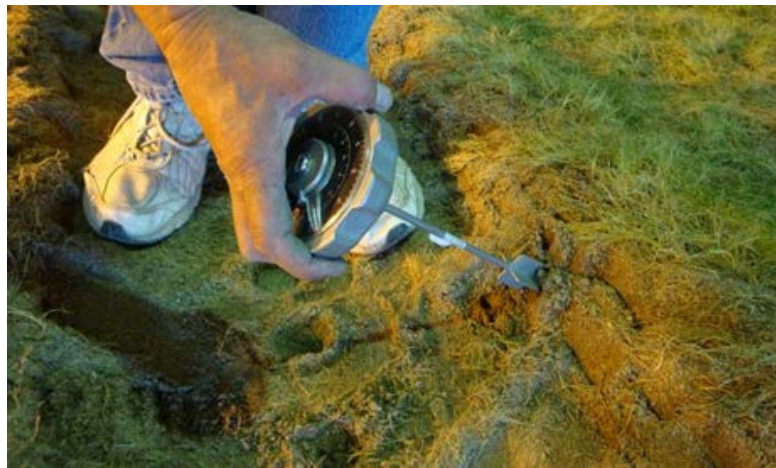
Figure 14. Pilcon shear vane used on a vegetation test section (Shoop et al. 2013).
