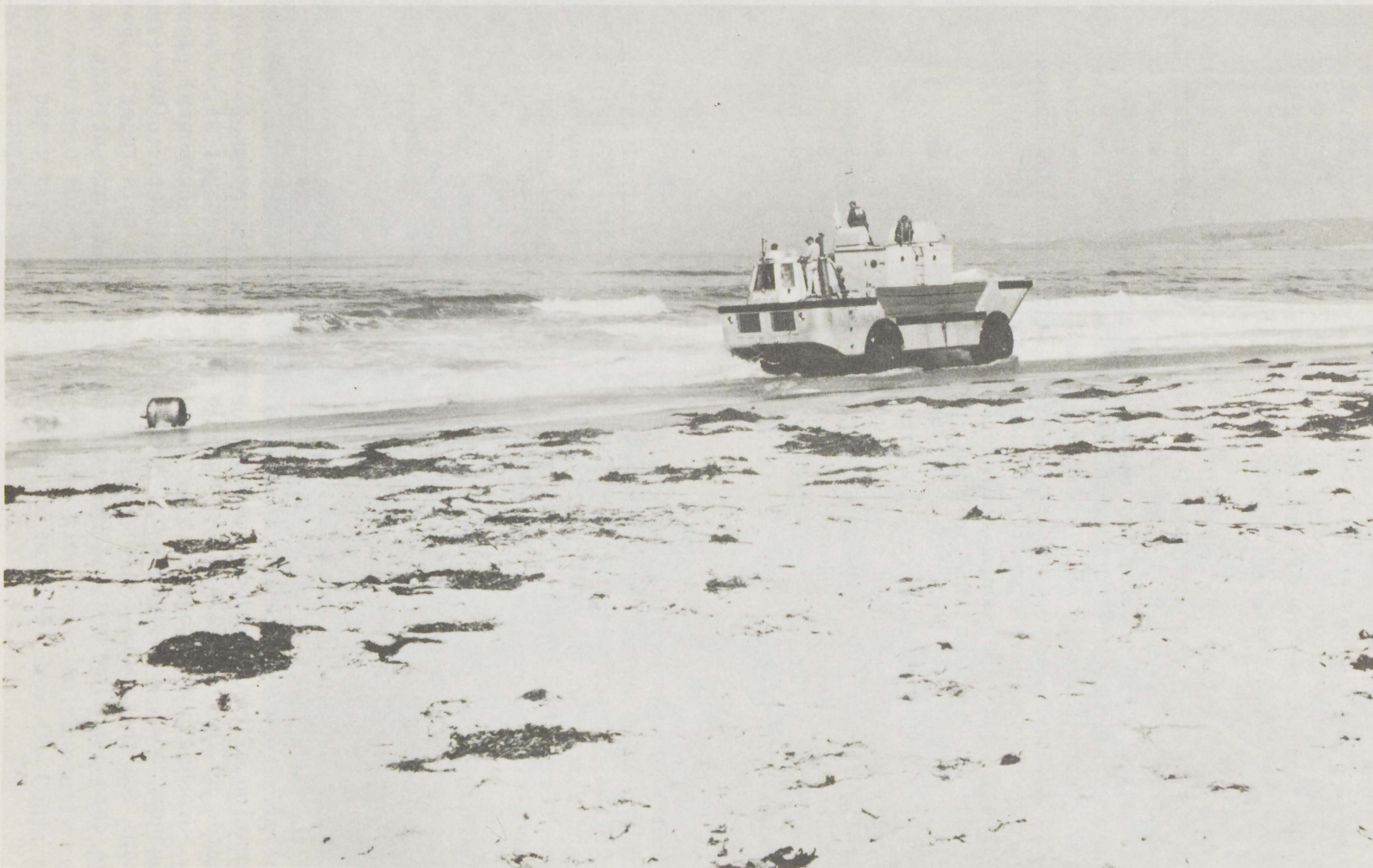
Figure 5. Amphibious LARC XV towing radiation detector vehicle entering surf. The ball-like device is connected to the LARC and the data acquisition system by means of electro-mechanical cable.
