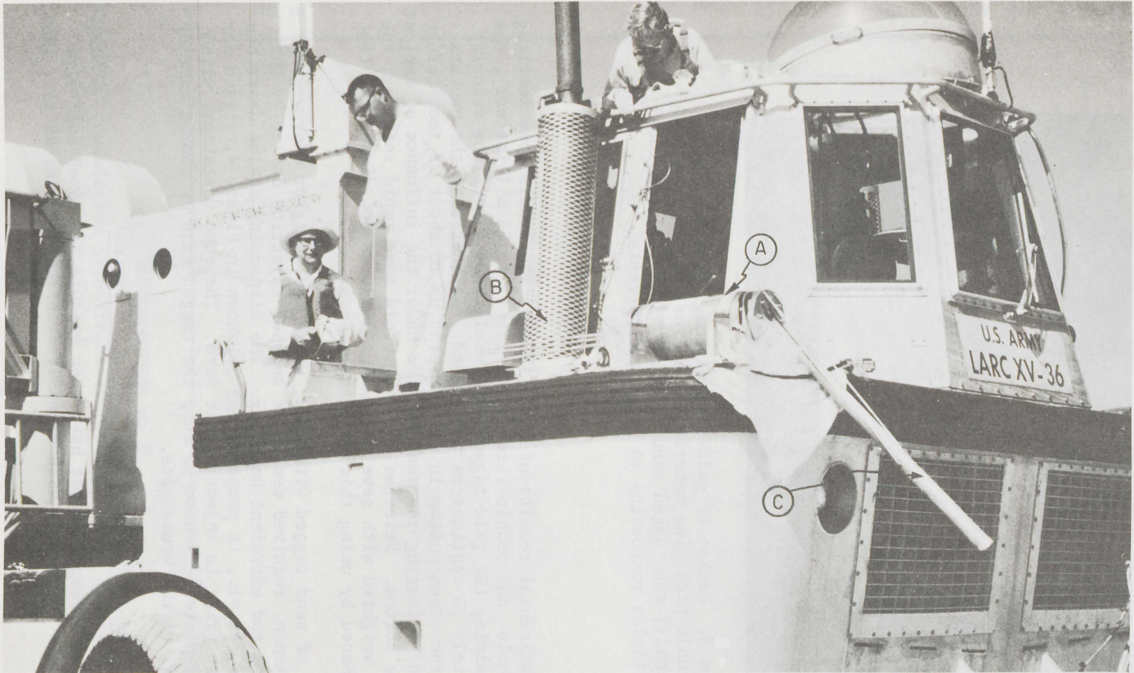
Figure 4. Tagged sand carrier-dispenser installed on stern of LARC XV. Slotted trays containing 12 packets of sand lie in the shielded cylinder "A"; push rods by which the three trays are extruded are installed at the left, "B", and on the right side of the cylinder is the chute "C" into which the packets fall and slide into the ocean.
