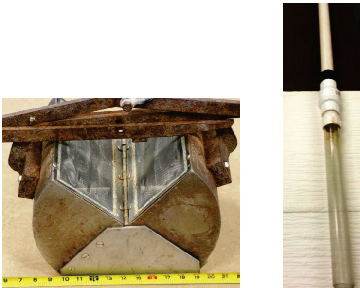
Figure 3. Images of the sampling devices used for sediment collection. A petite Ponar sampler is shown in the left panel, and an image of the 5 cm (2 in.) diameter push corer is shown in the right panel.
