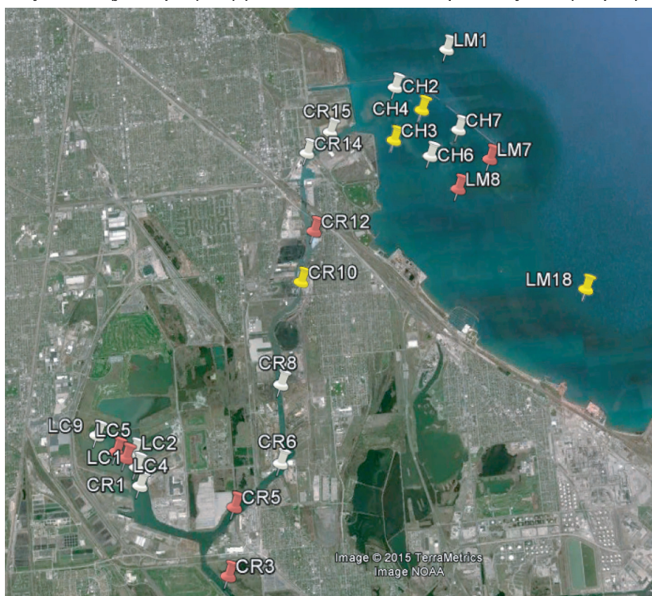
Figure 6. Location of radioisotope samples classified by (1) measurable gamma activity of ^7\text{Be} , ^{137}\text{Cs} , ^{234}\text{Th} , and/or ^{210}\text{Pb} (white pins); (2) measurable alpha activity only of ^{210}\text{Pb} (yellow pins); or (3) no measurable radioisotope activity at all (red pins).
