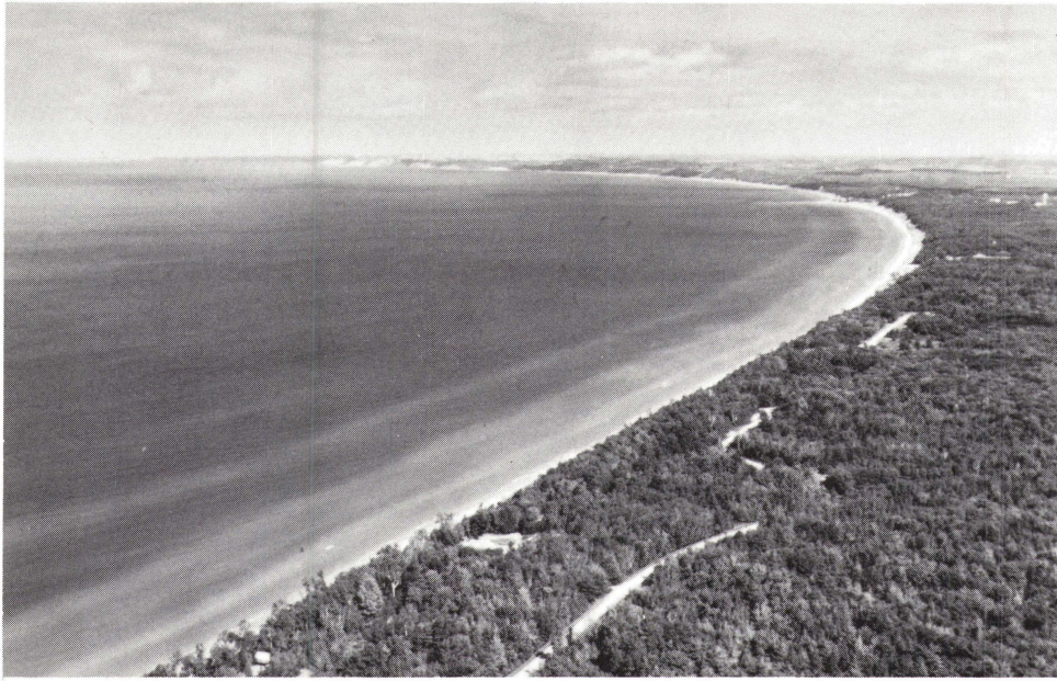
Figure 6. Longshore continuity of bars in the Great Lakes. The inner two to three bars are usually visible when viewed from high bluffs and dunes along the shore. In the above photo (taken about 900 meters above lake level) the inner three bars can be seen following the curve of the shoreline from station 10 toward Pentwater Harbor in the upper right corner (a distance of about 6 kilometers).
