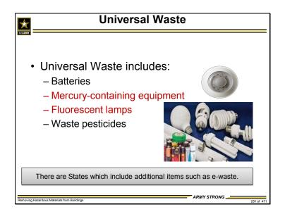
The items in red are those which are most likely to be encountered when conducting renovation and/or demolition, and that also are likely to contain mercury.
