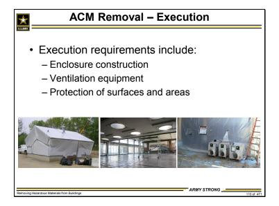
The idea is to keep the work area as small as possible and to keep that area under negative pressure to ensure that no airborne fibers leave the work area. Specific criteria for barrier construction and equipment performance are detailed in the requirements.
