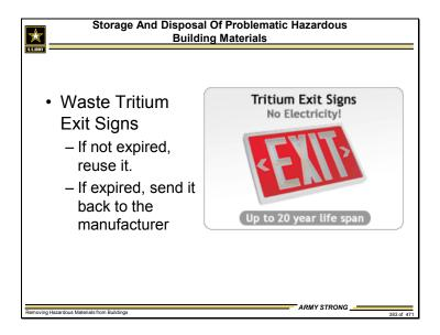
Many exit signs contain tritium, the radioactive form of hydrogen. Mixing tritium with a chemical that emits light in the presence of radiation, known as "phosphor in a tube" (a sealed source), creates a continuous self-powered light source. This useful property of tritium can be applied to situations where a dim light is needed, but where using batteries or electricity is not possible or practical.
