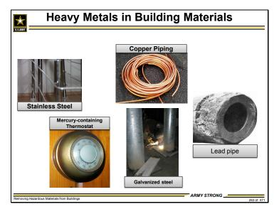
Today, *mercury* is found in such building parts as thermometers, barometers, switches, thermostats, flow meters, lamps, paints, stains, batteries, and fluorescent lamps.
