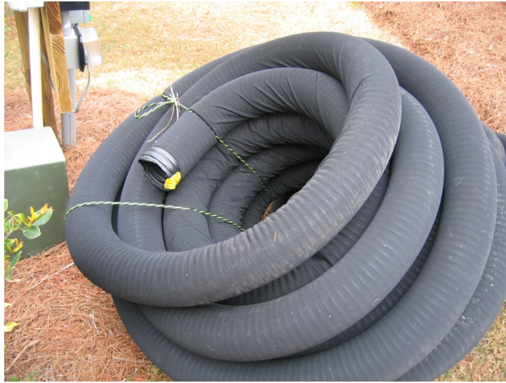
Figure 21. Drain tile with protective cover.
