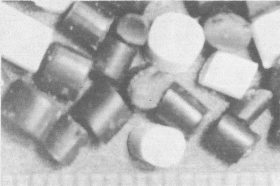
PVC cylinders, \gamma' = 0.3 D_{50} = 3 \text{ mm}
