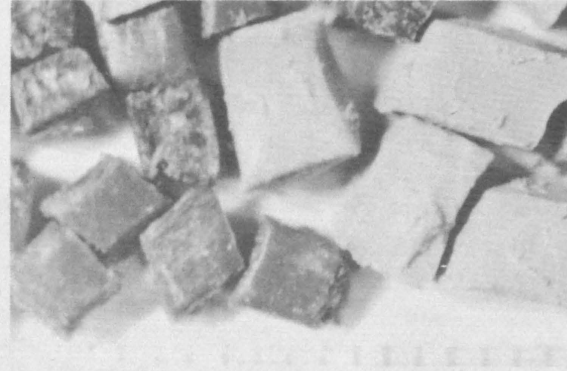
PVC cubes, \gamma' = 0.3 D_{50} = 3 \text{ mm}
