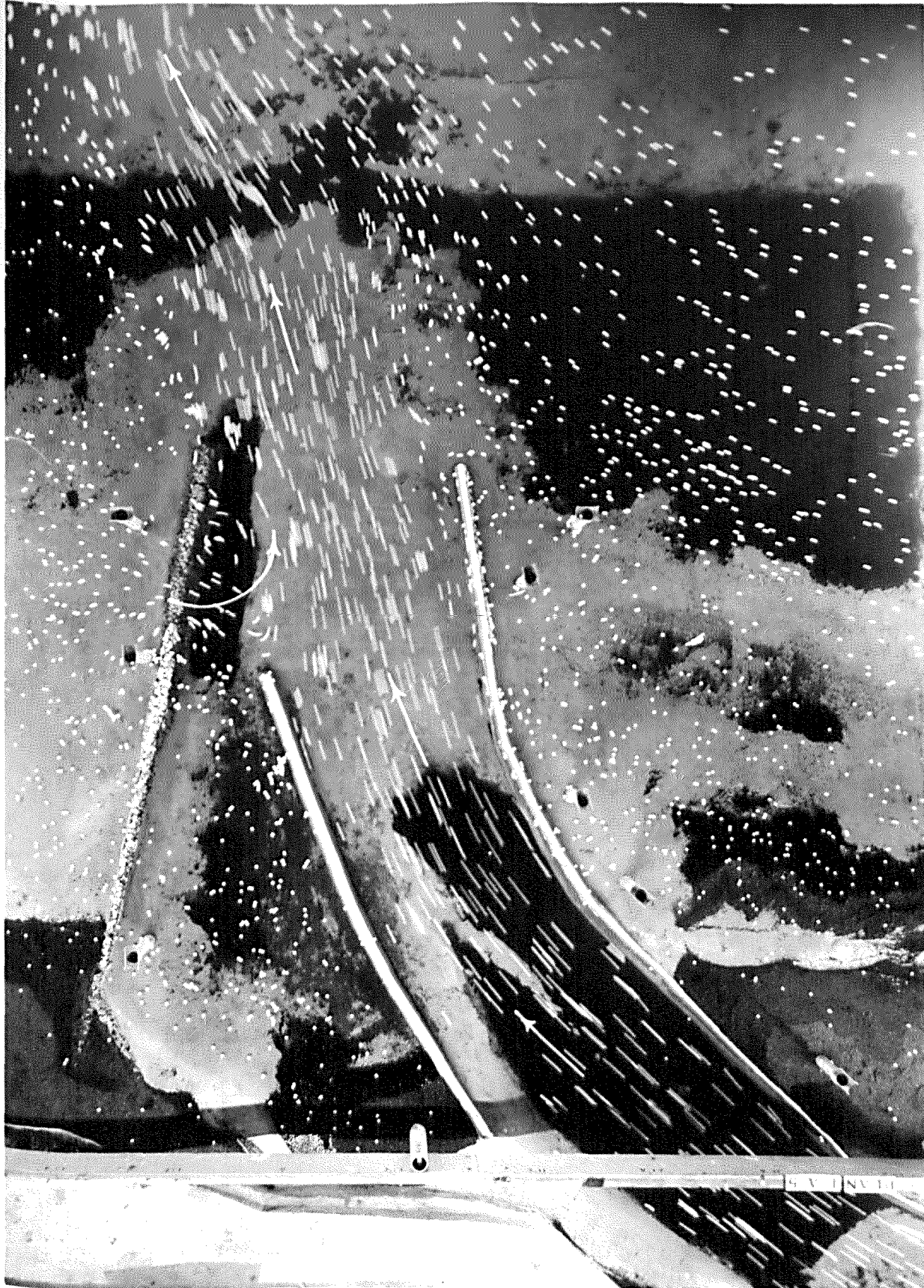
PHOTOGRAPH 17. Plan 1-A - Current directions at strength of ebb after LHW (hr. 4.0)
