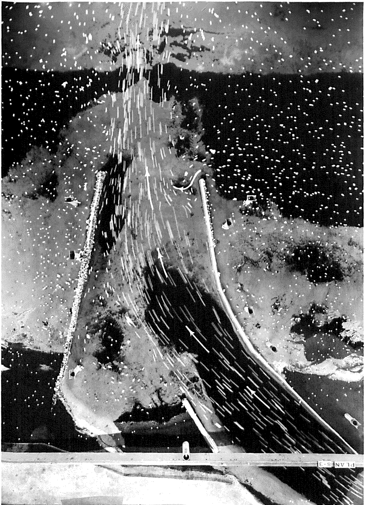
PHOTOGRAPH 23. Plan 8 - Current directions at strength of ebb after HHW (hr. 16.5)
