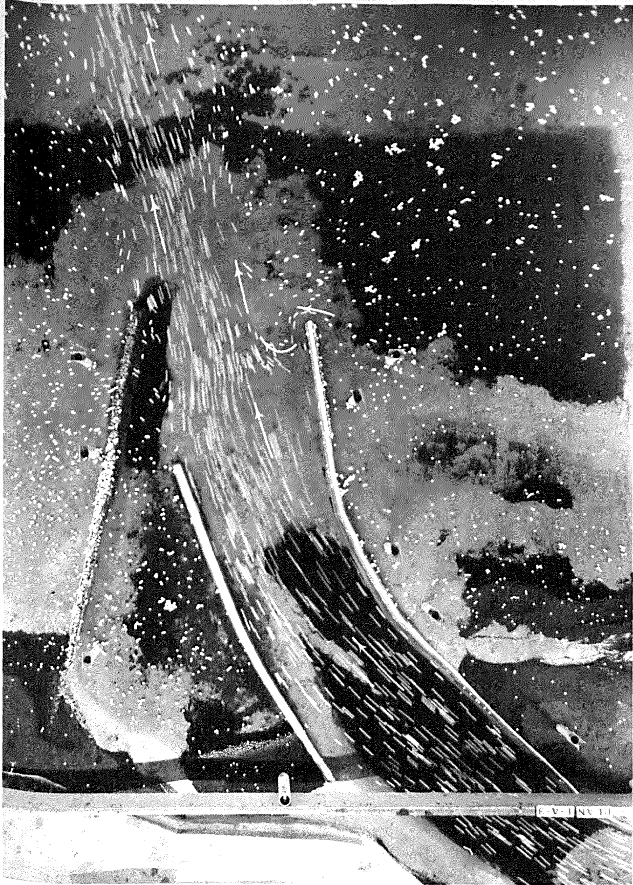
PHOTOGRAPH 15. Plan 1-A - Current directions at strength of ebb after HHW (hr 16.5)
