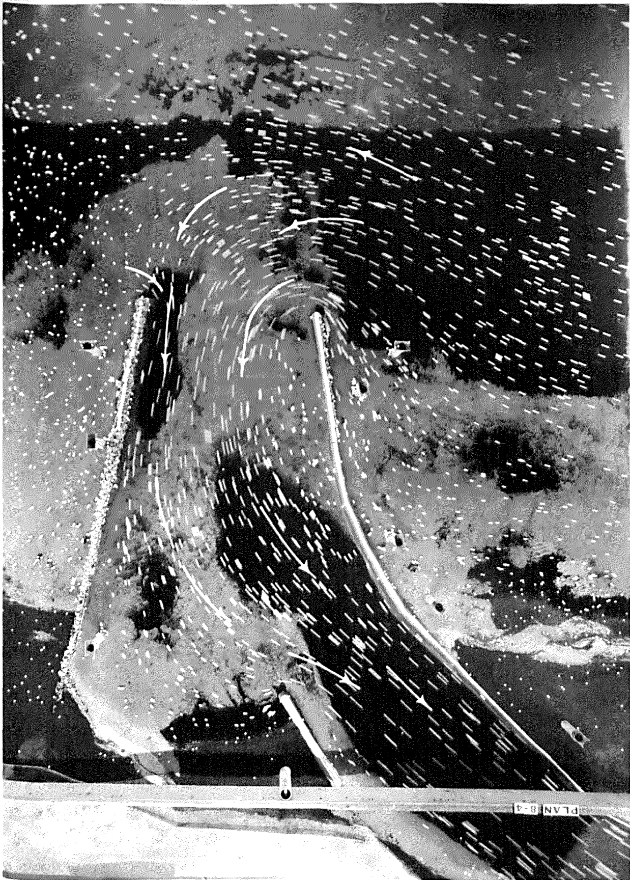
PHOTOGRAPH 24. Plan 8 - Current directions at strength of flood before LHW (hr. 23.0)
