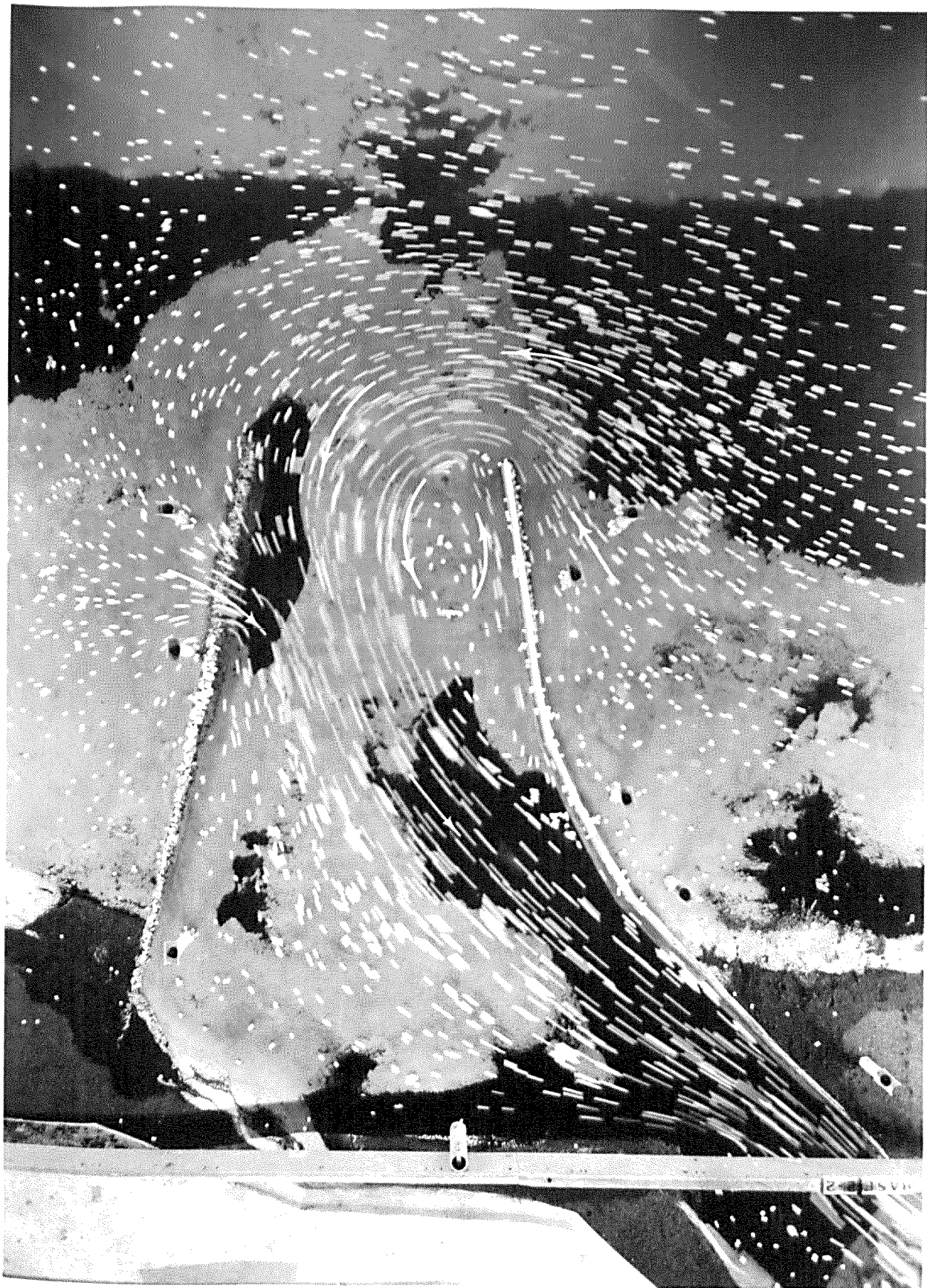
PHOTOGRAPH 6. Base Test - Current directions at strength of flood before HHW (hr. 10.5)
