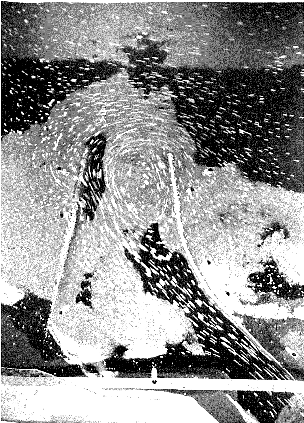
PHOTOGRAPH 8. Base Test - Current directions at strength of flood before LHW (hr. 23.0)
