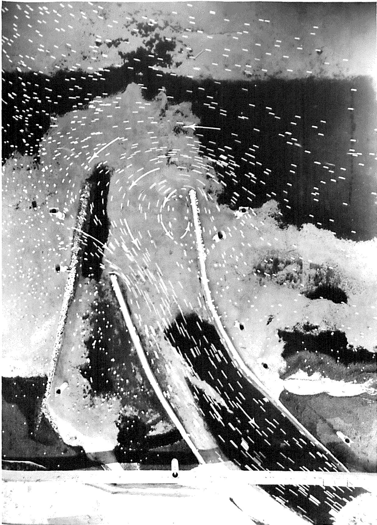
PHOTOGRAPH 16. Plan 1-A - Current directions at strength of flood before LHW (hr. 23.0)
