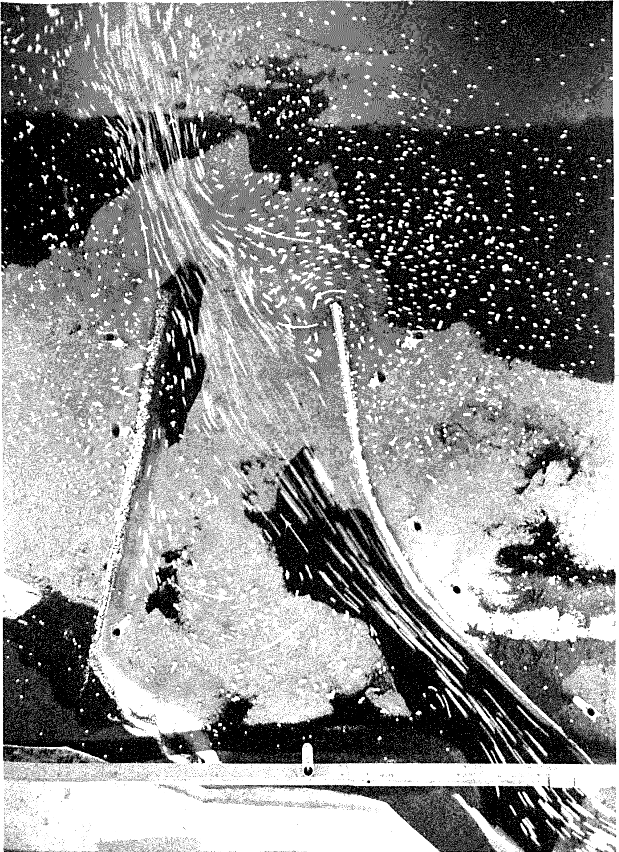
PHOTOGRAPH 7. Base Test - Current directions at strength of ebb after HHW (hr. 16.5)
