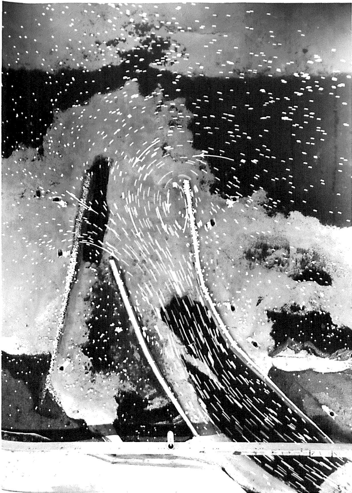
PHOTOGRAPH 14. Plan 1-A - Current directions at strength of flood before HHW (hr. 10.5)
