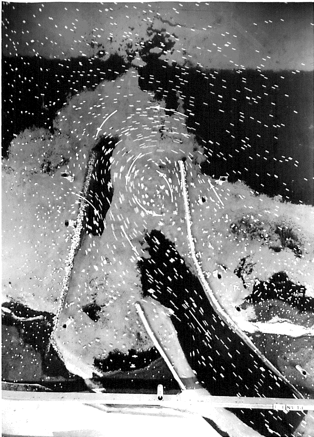
PHOTOGRAPH 12. Plan 1 - Current directions at strength of flood before LHW (hr. 23.0)
