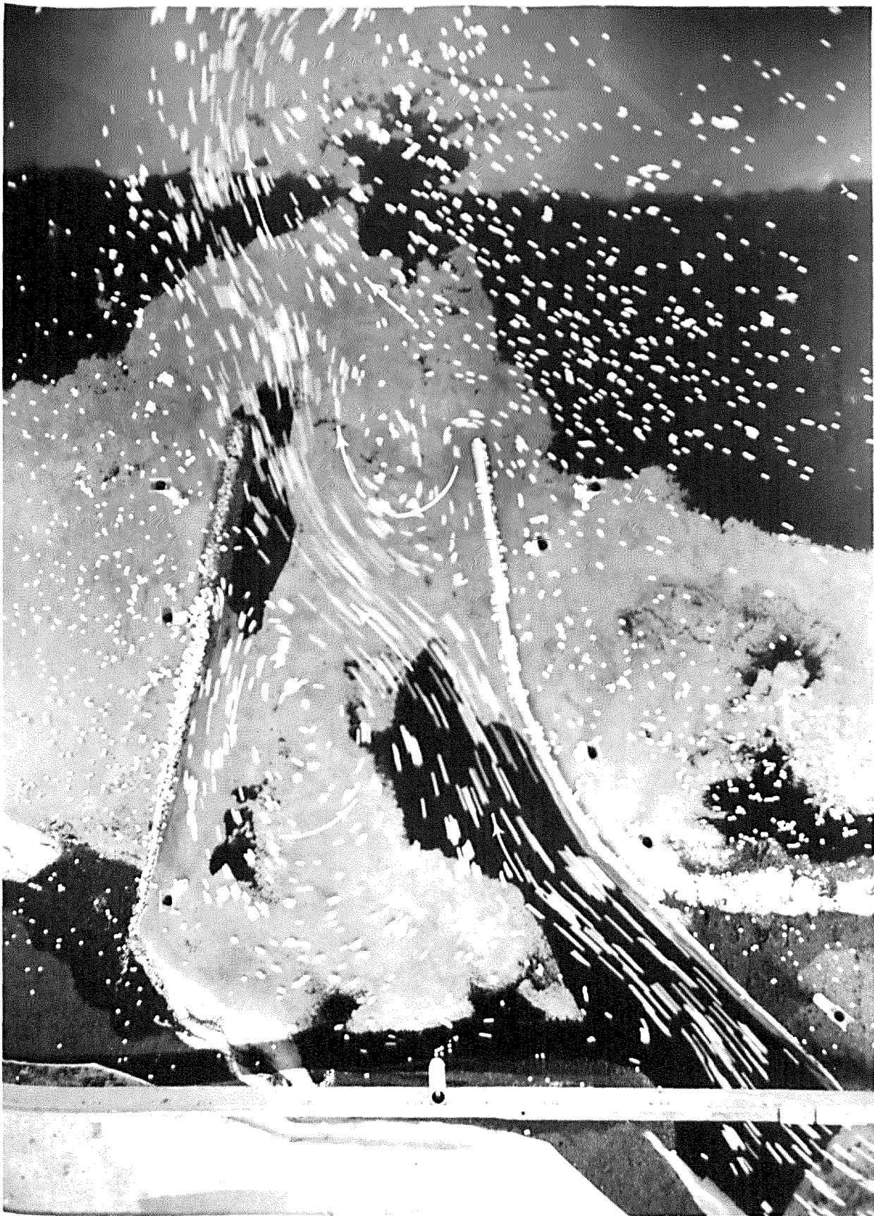
PHOTOGRAPH 9. Base Test - Current directions at strength of ebb after LHW (hr. 4.0).
