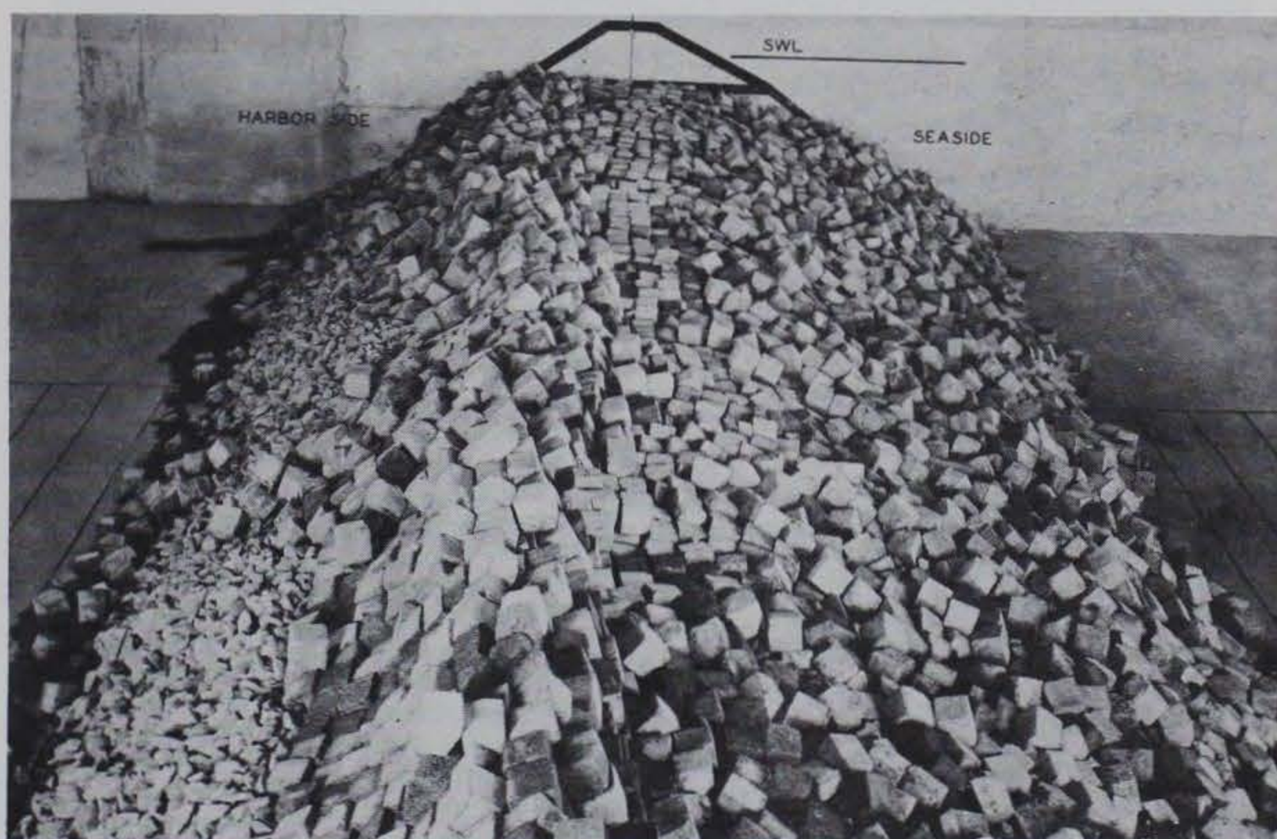
Fig. 10. Test series 4, complete breakwater section after 21-ft wave attack, class A stone of molded concrete blocks
