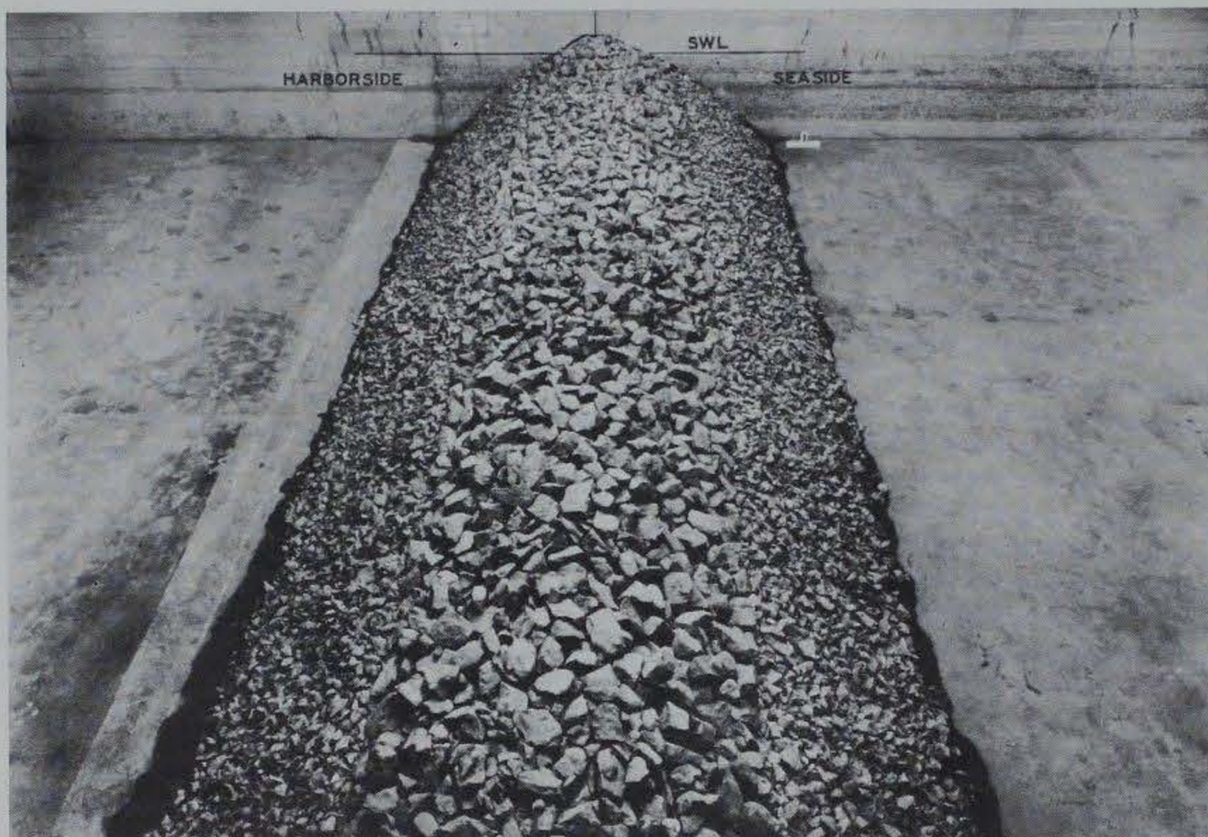
Fig. 11. Test series 4, complete breakwater section before wave attack, class A stone of crushed limestone
