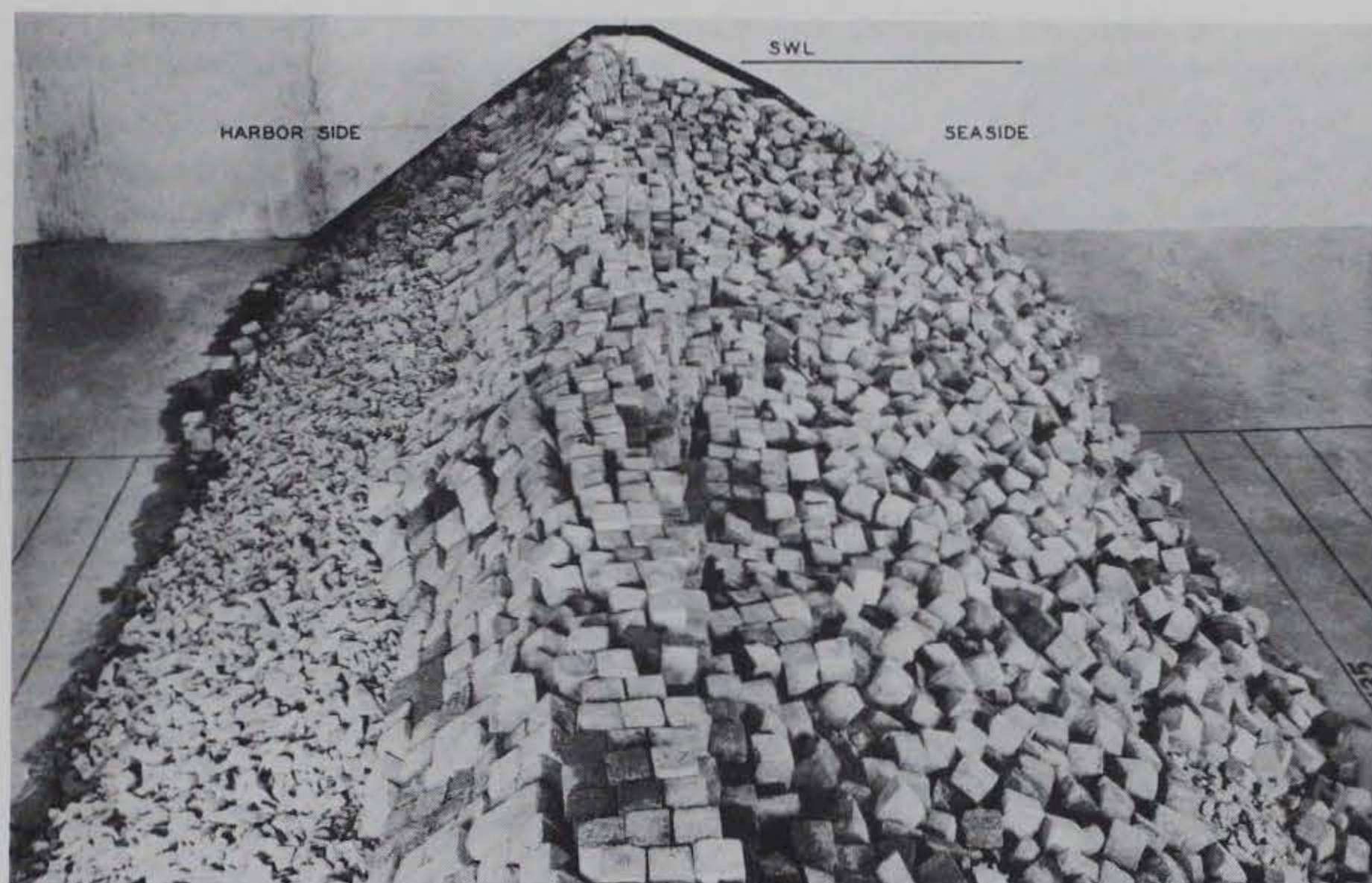
Fig. 9. Test series 4, complete breakwater section after 15-ft wave attack, class A stone of molded concrete blocks
