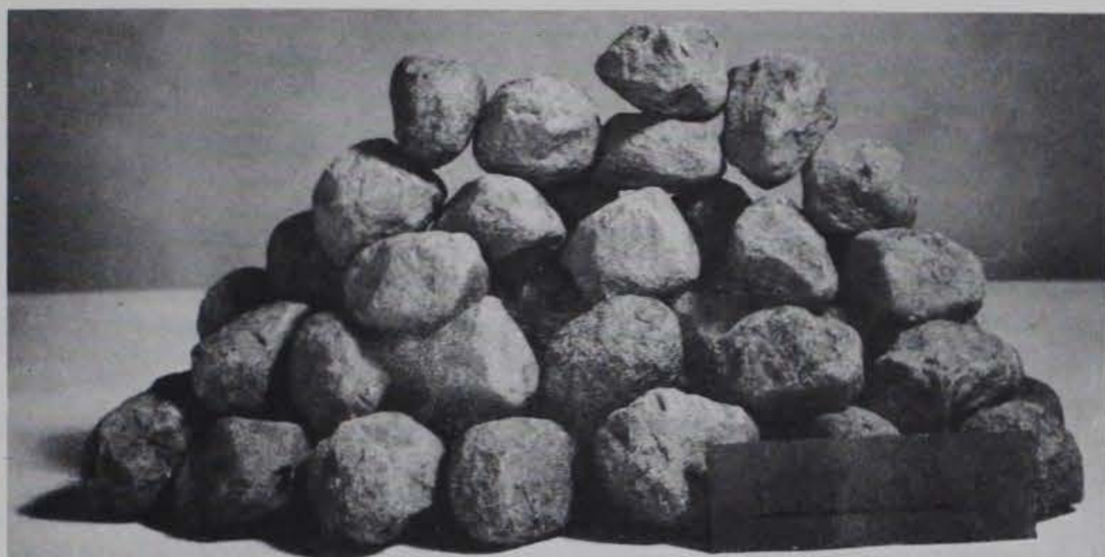
Fig. 16. Investigation of Iribarren's formula, 13.5-ton, 2.8-specific-gravity cap rock
