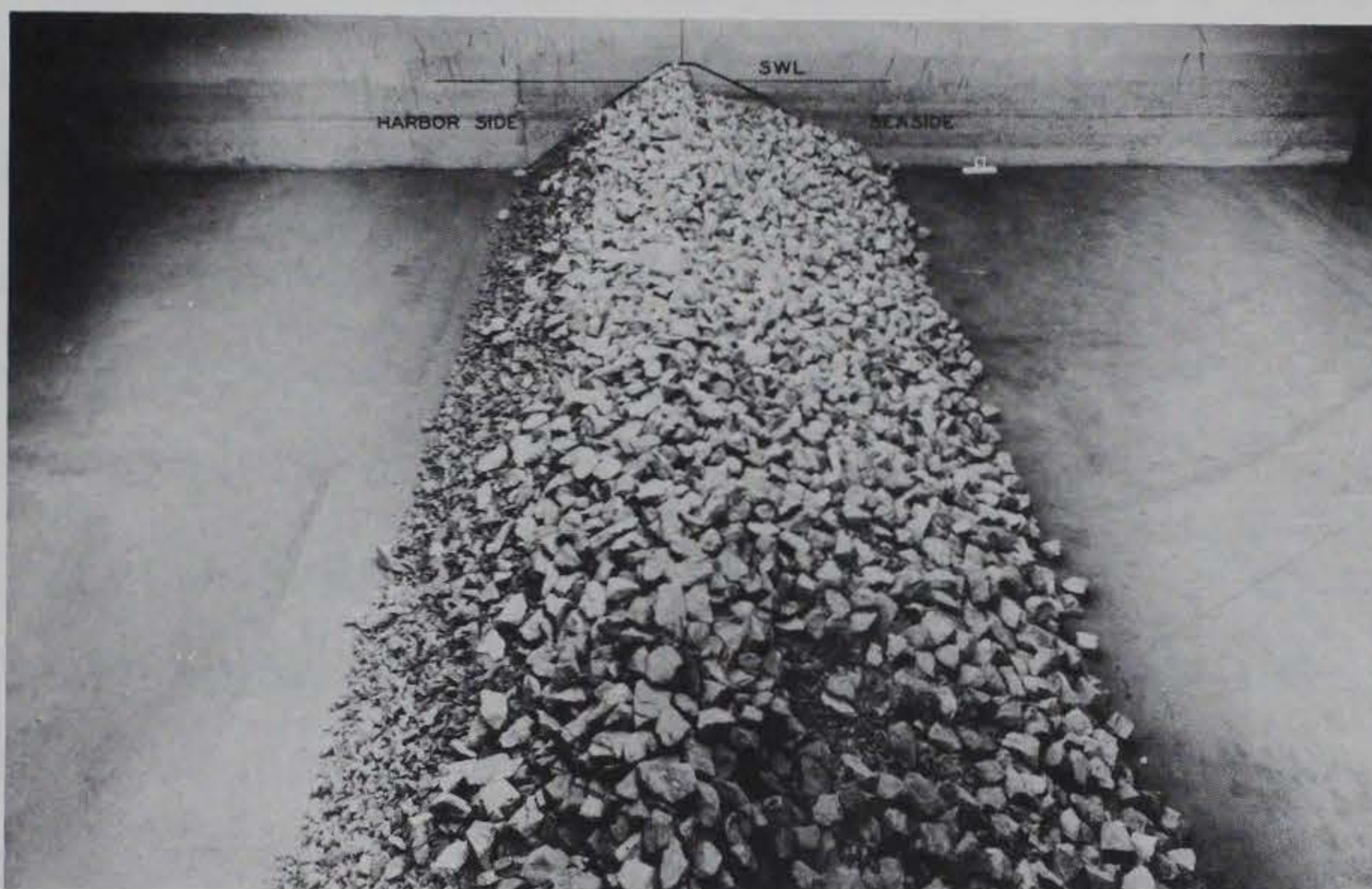
Fig. 12. Test series 4, complete breakwater section after 15-ft wave attack, class A stone of crushed limestone
