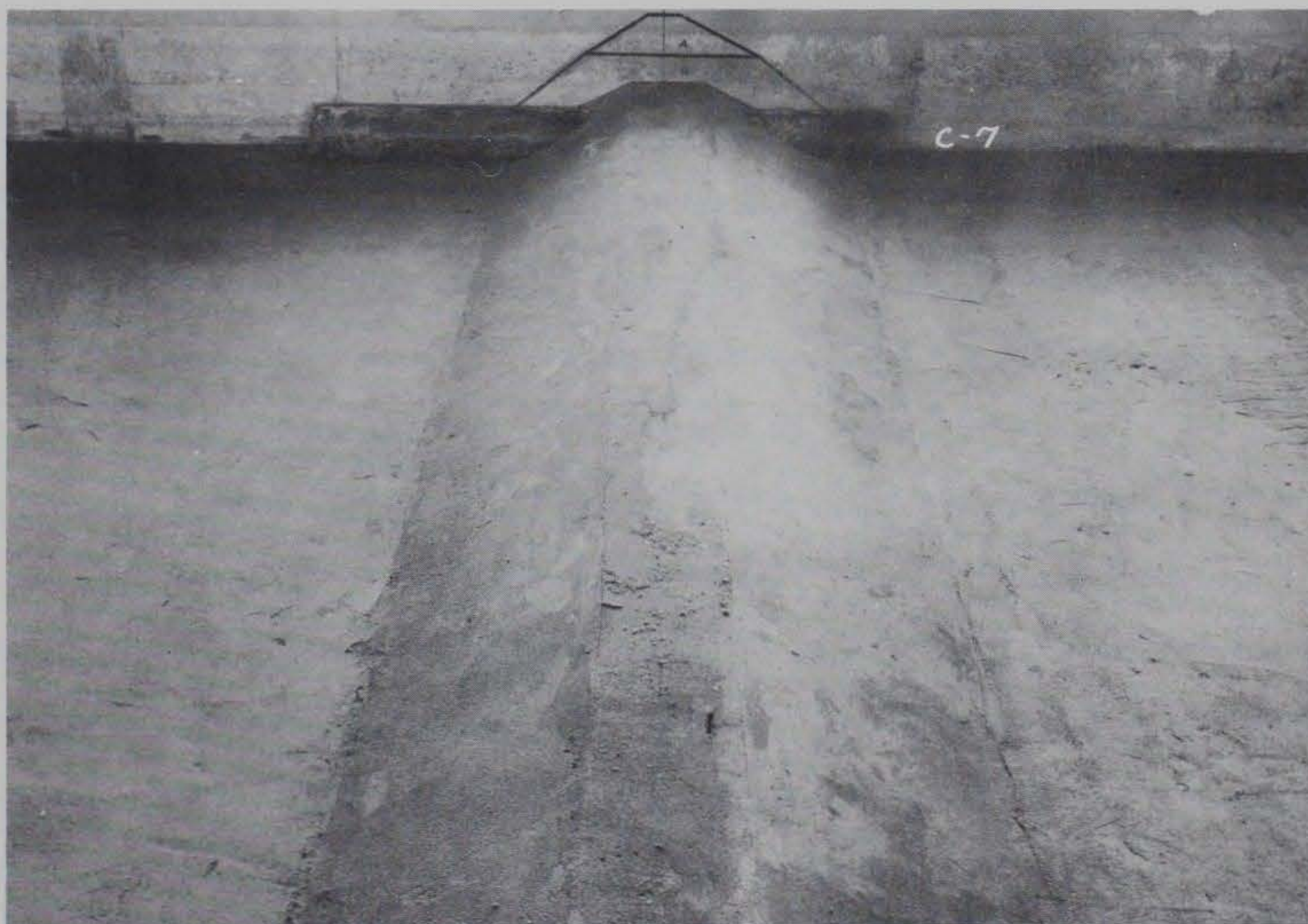
Fig. 5. Class C section before wave attack, 1:45-scale model
