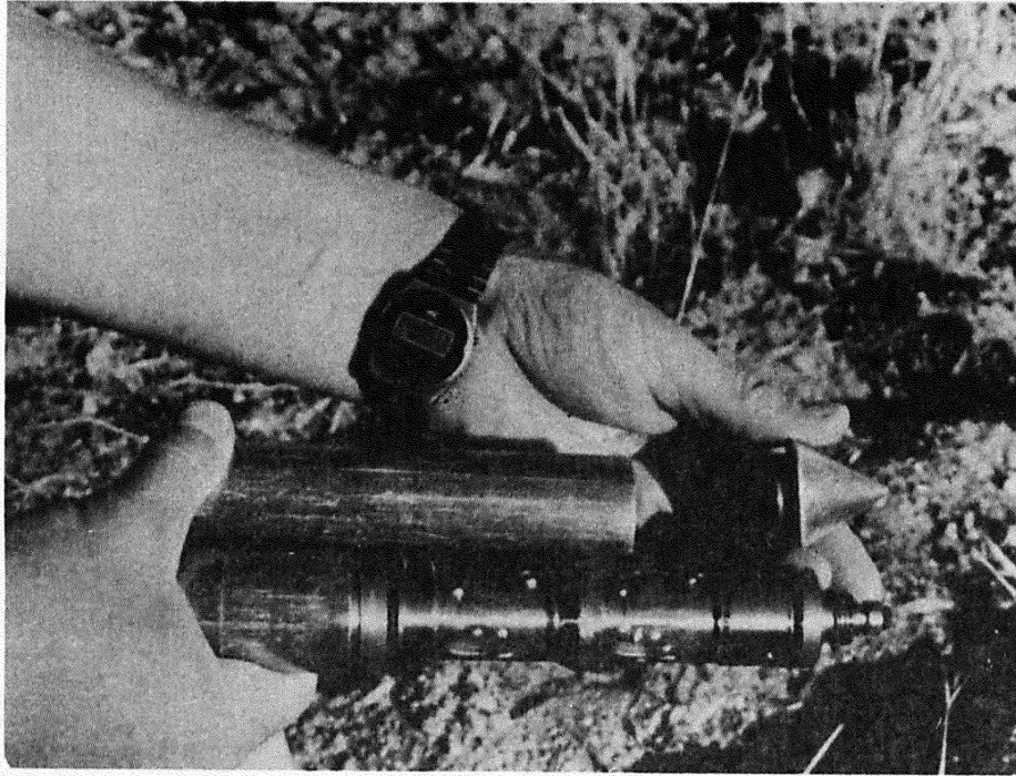
Figure 10. Photograph of Disassembled Electrical Cone Penetrometer Tip, Standard (10 cm 2 ) Size.
