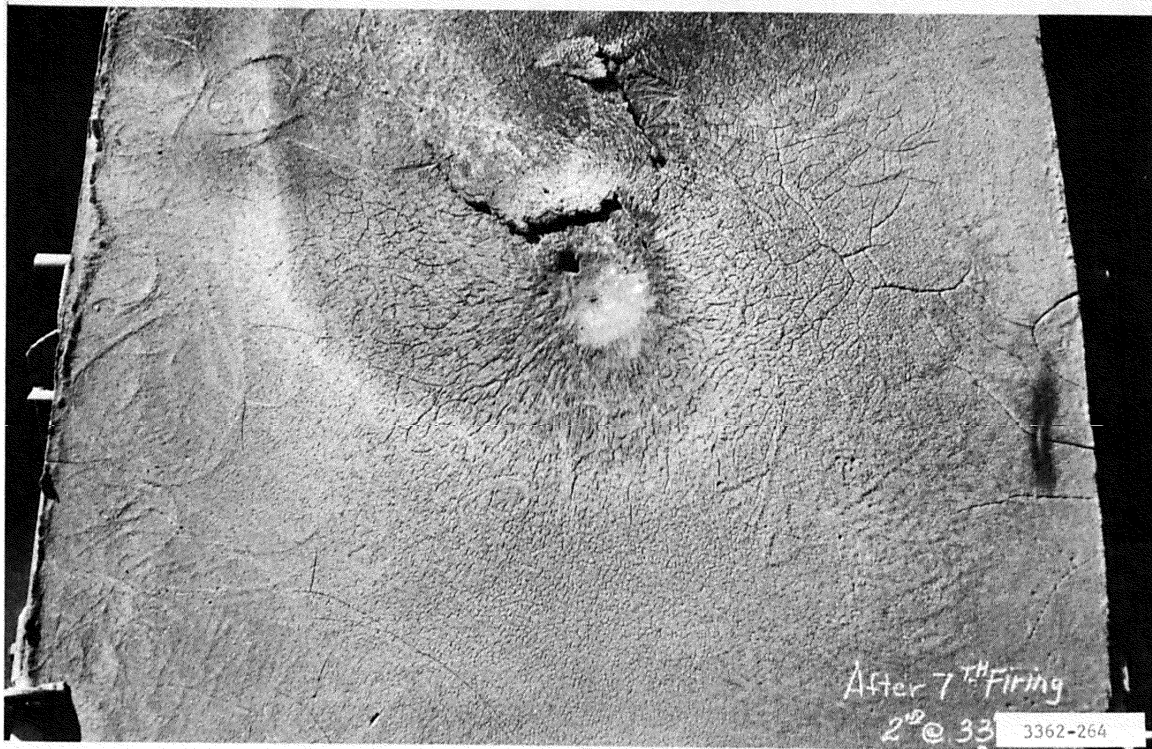
Photograph 10. Hetron 24806 specimen after series of exposures to liquid-propellant motor exhausts
