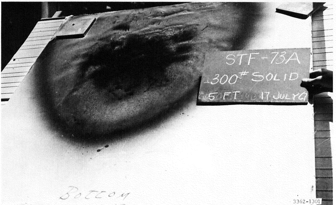
Photograph 4. Reichhold STF 73A specimen after 5-ft-distance, solid-propellant motor test at exposure temperature of 2800 F
