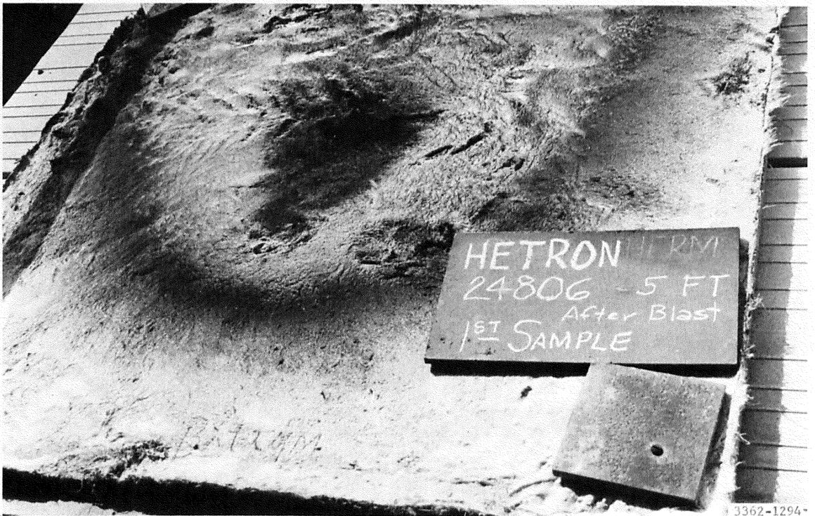
Photograph 8. Hetron 24806 specimen after 5-ft-distance, solid-propellant motor test
