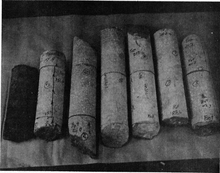
Figure C.1 As-received 6-inch cores.
