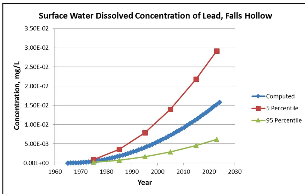
Figure 3. Computed dissolved lead concentration in water at Falls Hollow Bridge with upper and lower 95% confidence bounds for uncertainty in  $K_d$ .
