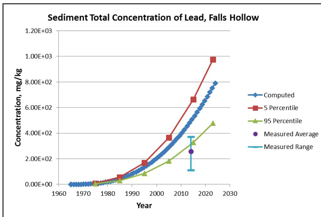
Figure 2. Computed and measured lead total concentration in benthic sediment in Falls Hollow with upper and lower 95% confidence bounds for uncertainty in  $K_d$ .
