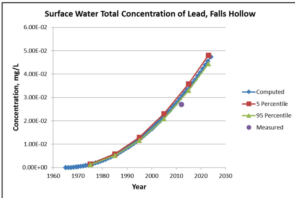
Figure 1. Computed and measured lead total concentration in water at Falls Hollow Bridge with upper and lower 95% confidence bounds for uncertainty in  $K_d$ .
