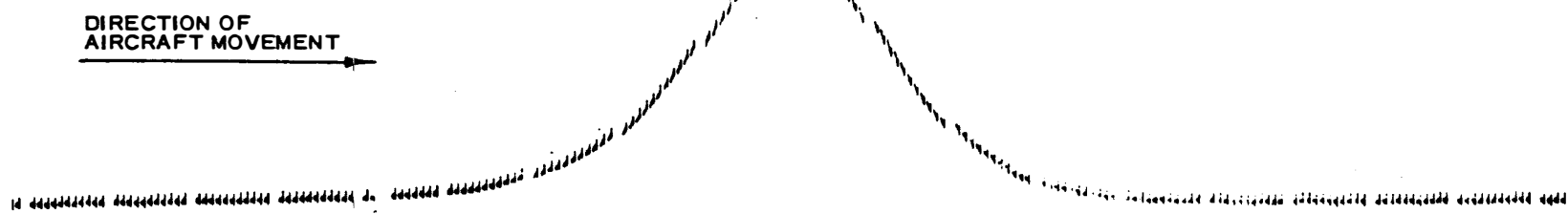
Figure 4. Typical recording for an SE soil pressure cell, 1974
