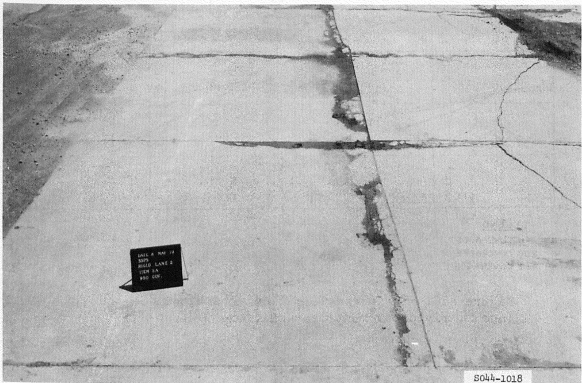
Figure A49. Subitem 5a, lane 2, rigid pavement test section, after 950 coverages by 240-kip twin-tandem assembly
