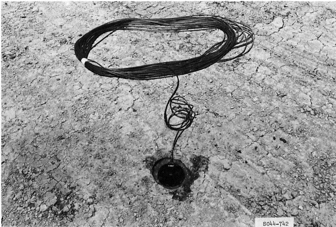
Figure 42. Placement of a Bison strain sensor
