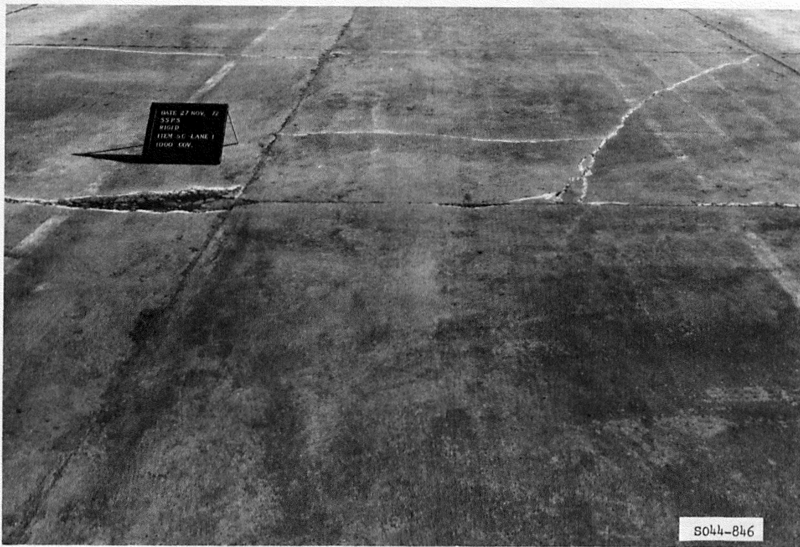
Figure A27. Subitem 5c, lane 1, rigid pavement test section, after 1000 coverages by 200-kip twin-tandem assembly
