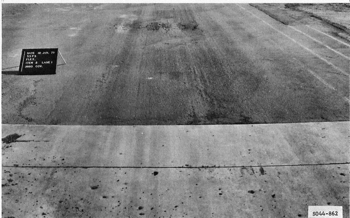
Figure B6. Item 2, lane 1, flexible pavement test section, at 3660 coverages of 200-kip twin-tandem assembly
