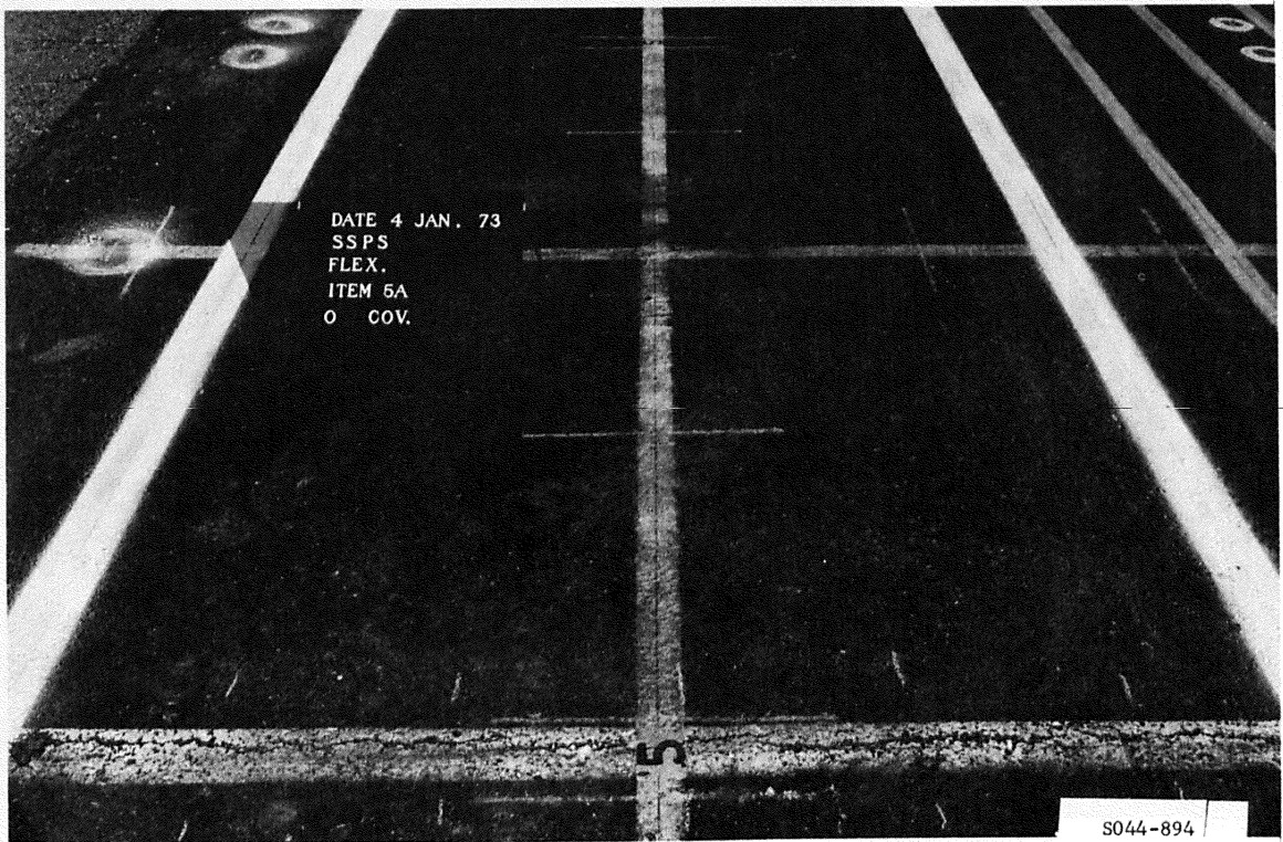
Figure B60. Subitem 5a, lane 3, flexible pavement test section, prior to traffic
