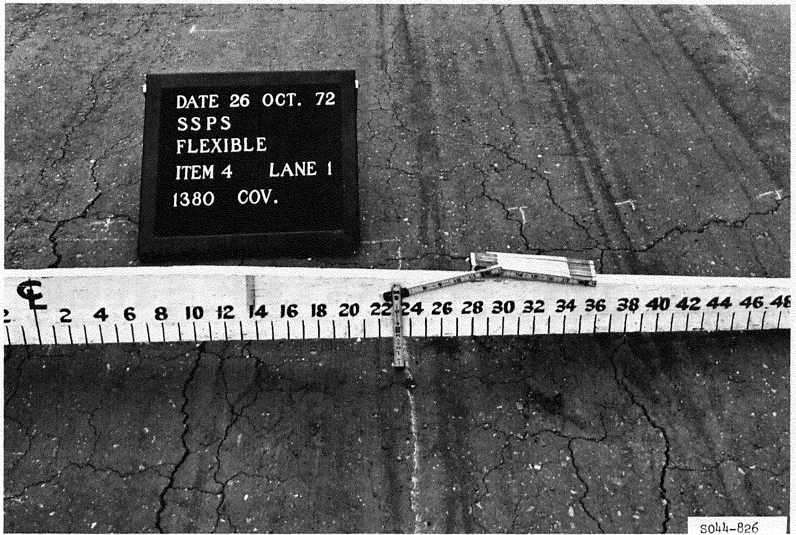
Figure B11. Item 4, lane 1, flexible pavement test section, at 1380 coverages of 200-kip twin-tandem assembly
