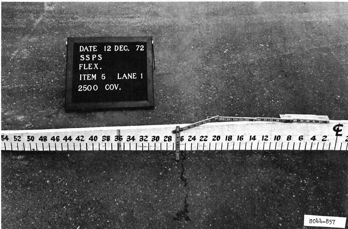
Figure B14. Item 5, lane 1, flexible pavement test section, at 2500 coverages of 200-kip twin-tandem assembly
