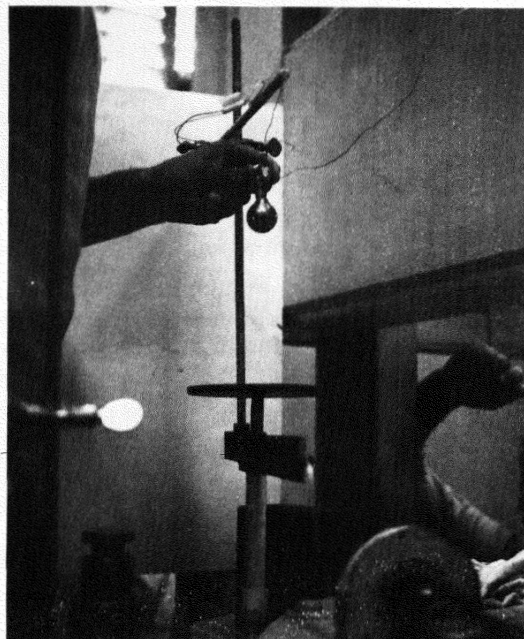
(c) Ball dropped from reference bar height to strike center of plate
