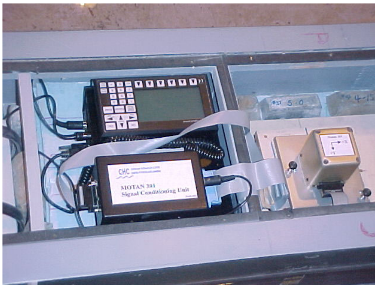
Figure 7. MOTAN motion analysis system installed in the model ship
