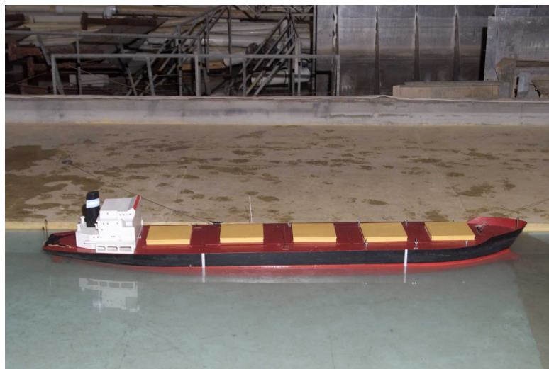
Figure 6. Scale model of the World Utility with remote control operation
