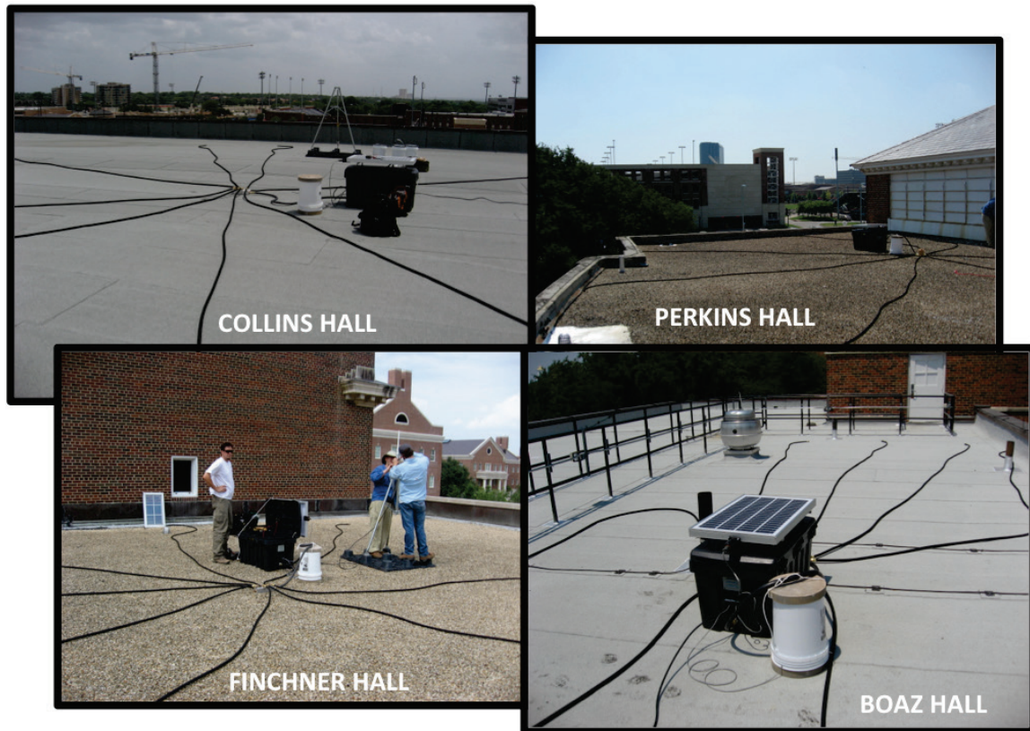
Figure 4. Photographs of the multi-rooftop array. Highlights include the roof infrastructure, roof vents and raised edges, which could create a complex noise environment for the array.
