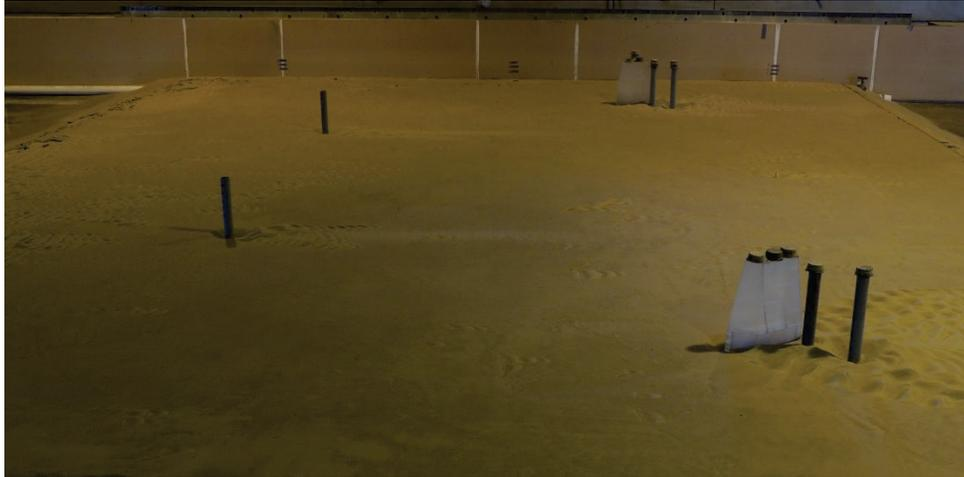
Figure 2. Test configuration of round piers and pier sets for Test 5.
