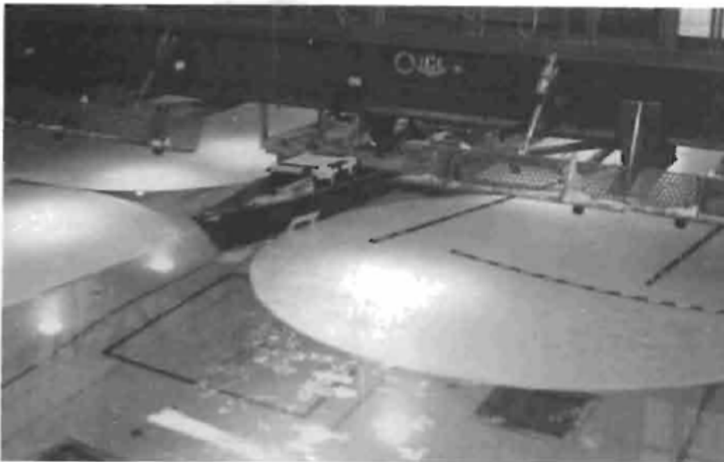
Figure 9. Ice-impact test conducted in CRREL Ice Towing Basin on conceptual navy frigate (Devine and Sodhi 1992). A custom-made pressure-sensing panel ( white box ) recorded local pressures at the ice–ship contact area (image courtesy of U.S. Navy).
