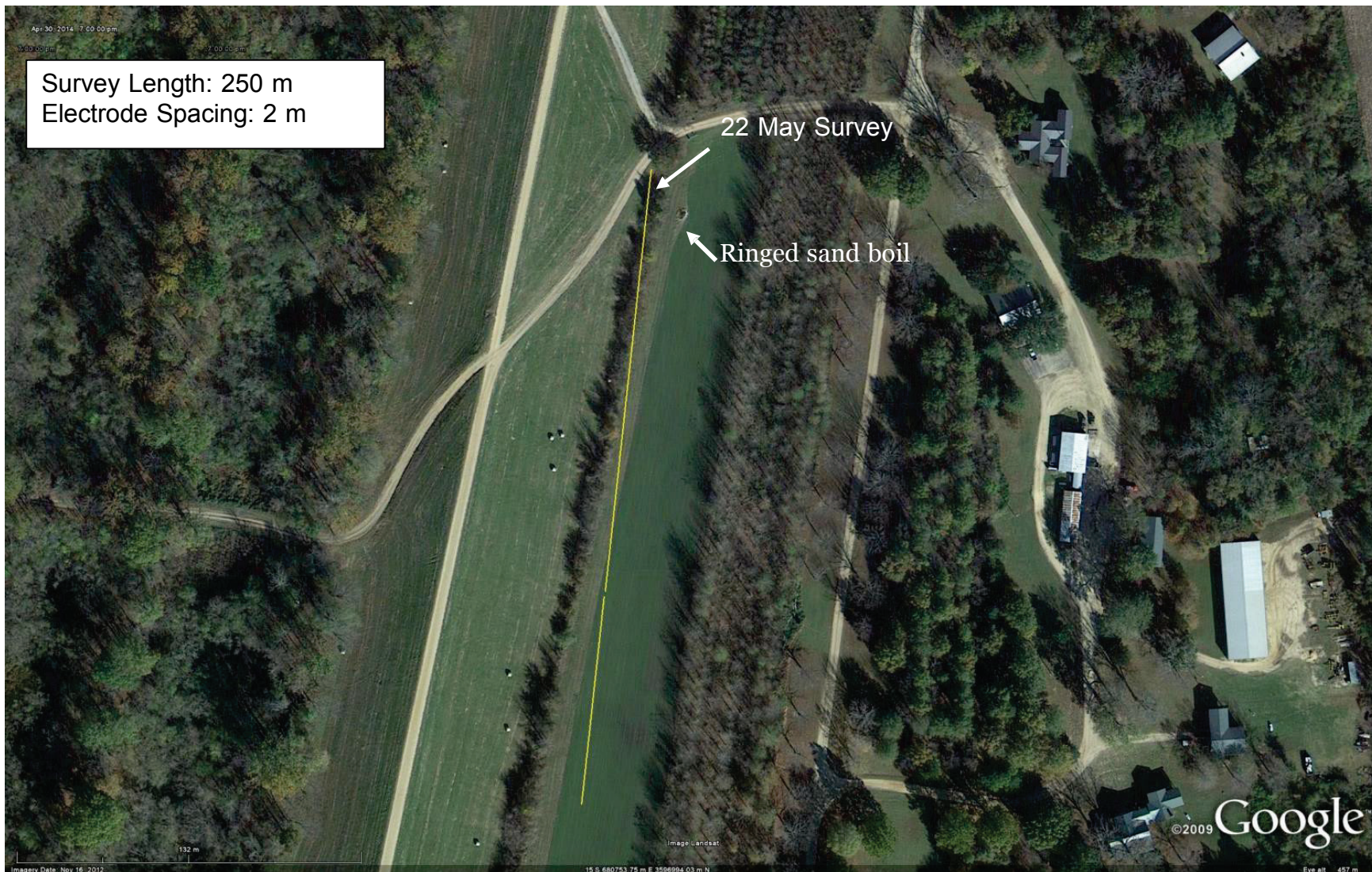
Figure 20. Northern ERT survey transecting areas of seepage. Notice ringed sand boil (Google 2009).
