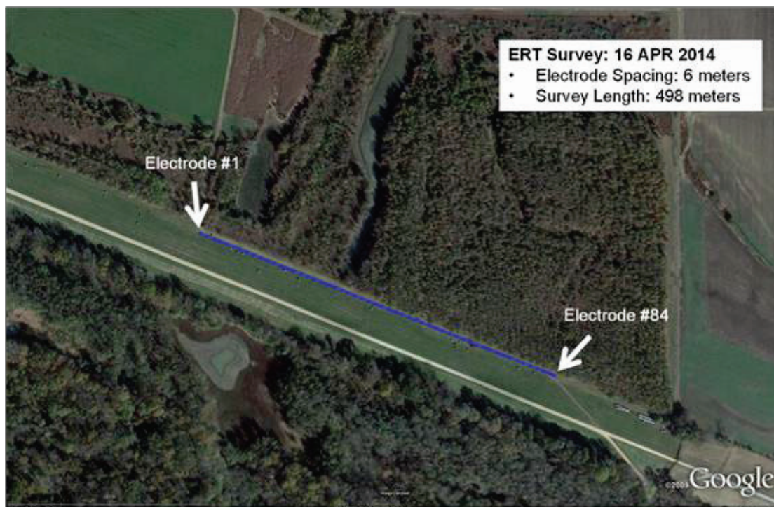
Figure 29. Southern Tara Wildlife Lodge electrical resistivity array (Google 2009).
