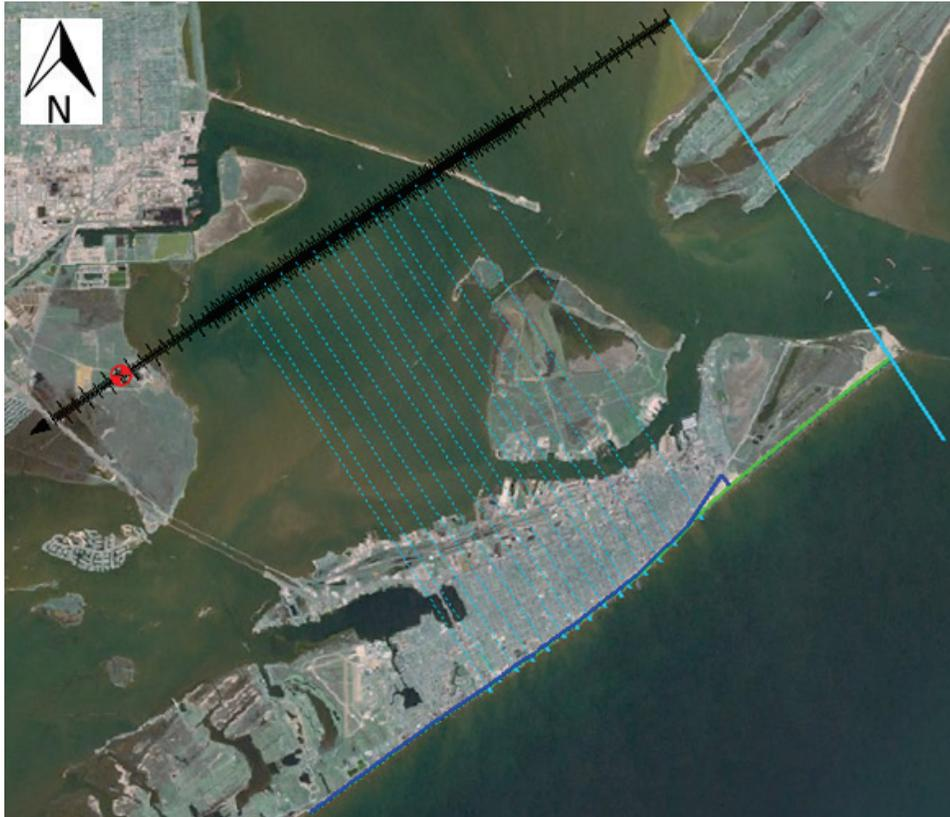
Figure 16. GenCade setup for west end grid.
