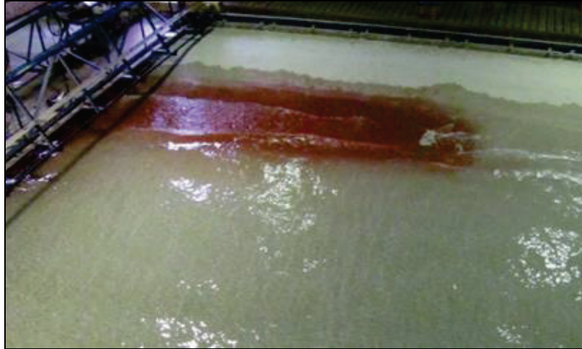
Figure 3. Beneficial use of nearshore placed dredged material (in red) experiments.
