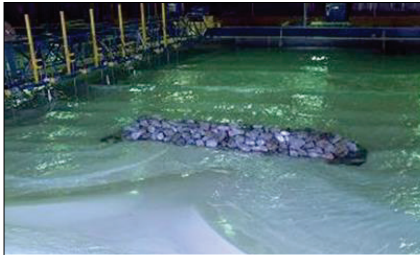
Figure 2. Experiments showing a tombolo forming leeward of a detached breakwater.
