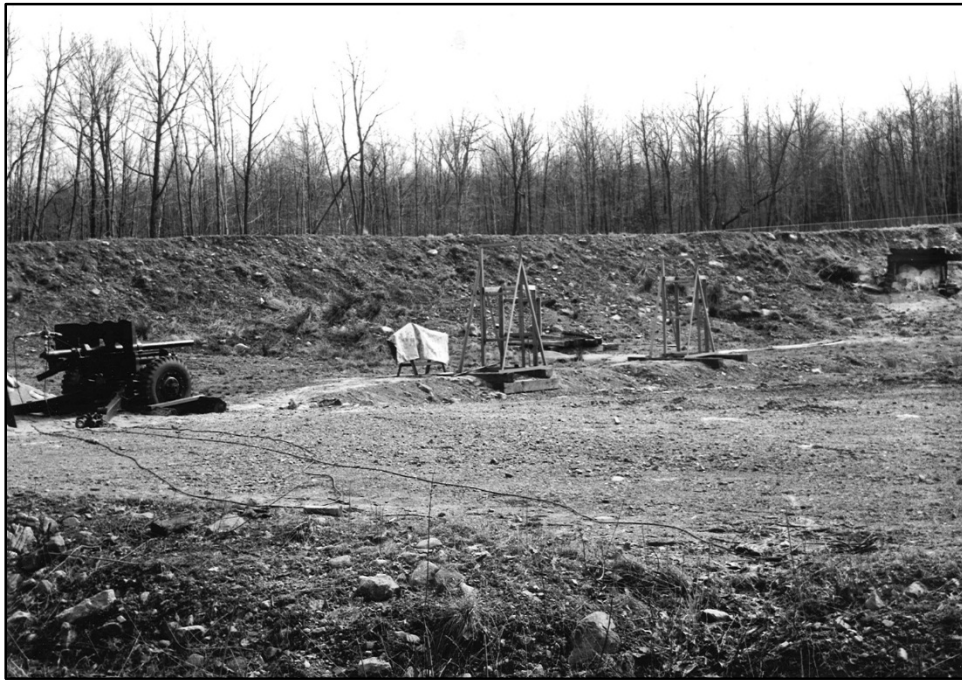
Figure 269. Arrangement of velocity screens for use with 57 mm gun at range at Building 1505, 1951 (Picatinny Arsenal Cultural Resources).
