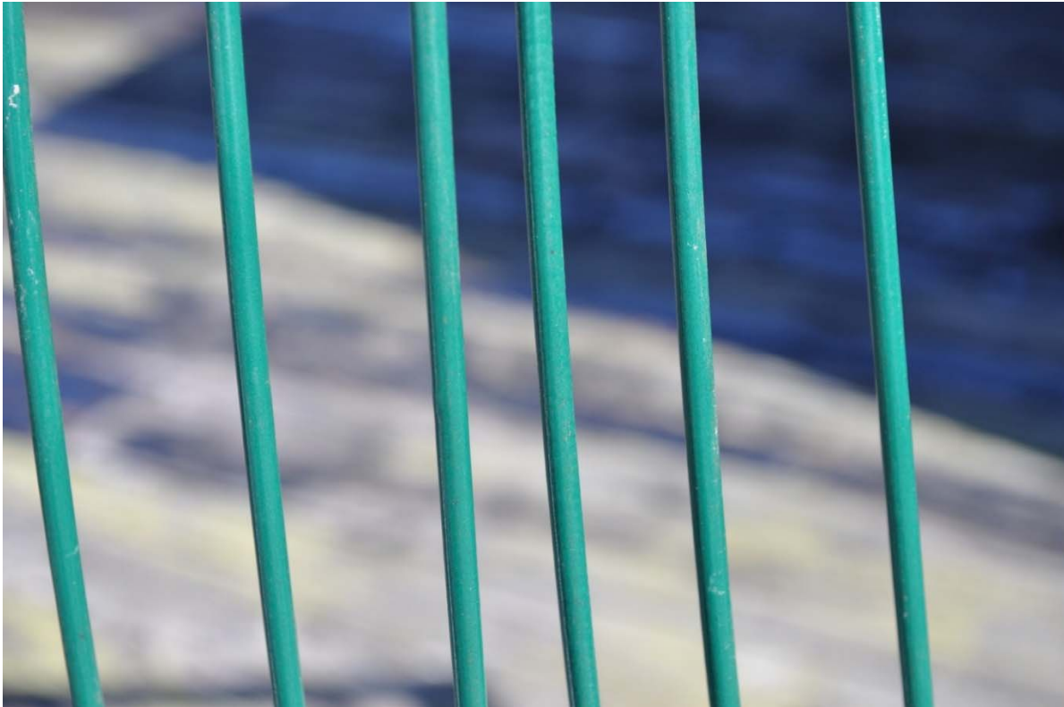
Figure B142. Fuse Bonded PVC Coated Galvanized Wire Coupon
