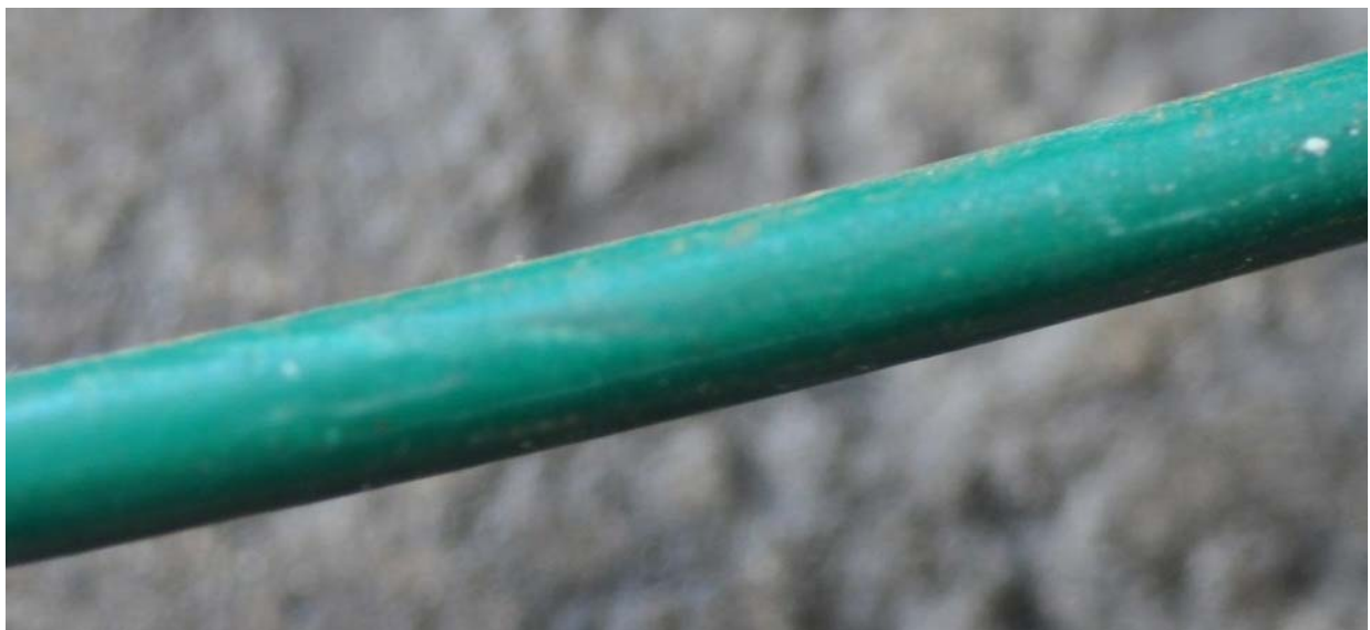
Figure B130. Fuse Bonded PVC Coated Galvanized Wire Coupon
