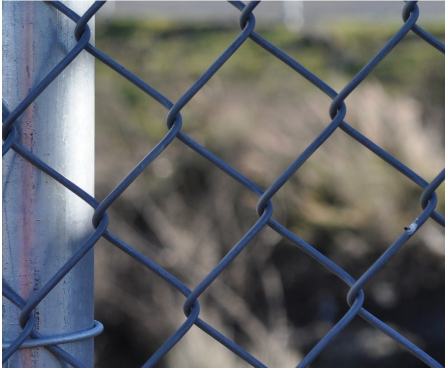
Figure A13. Galvan PVC after 6 months exposure.
