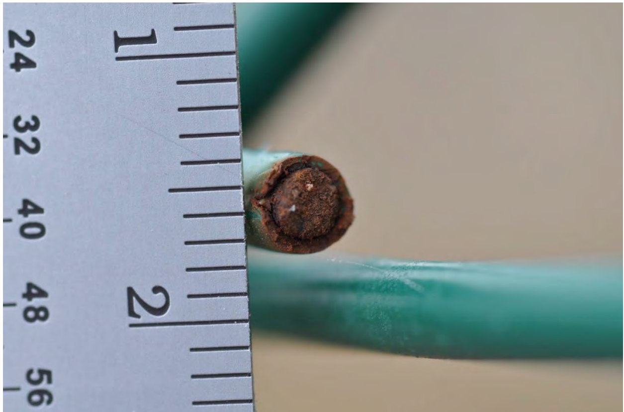
Figure B64. Fuse Bonded PVC Coated Galvanized Wire Fencing Cut Ends
