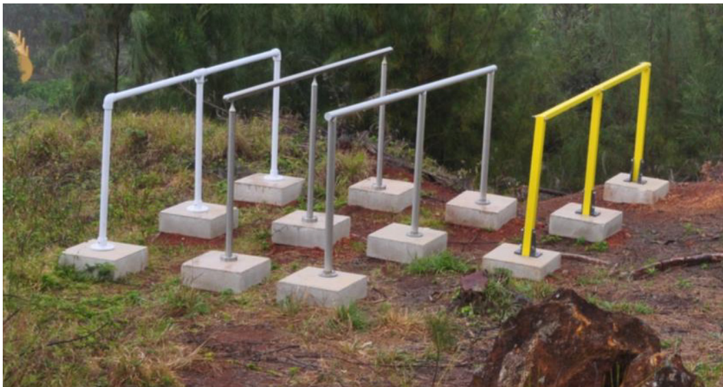
Figure 7. Railing test sections installed at KTA.
