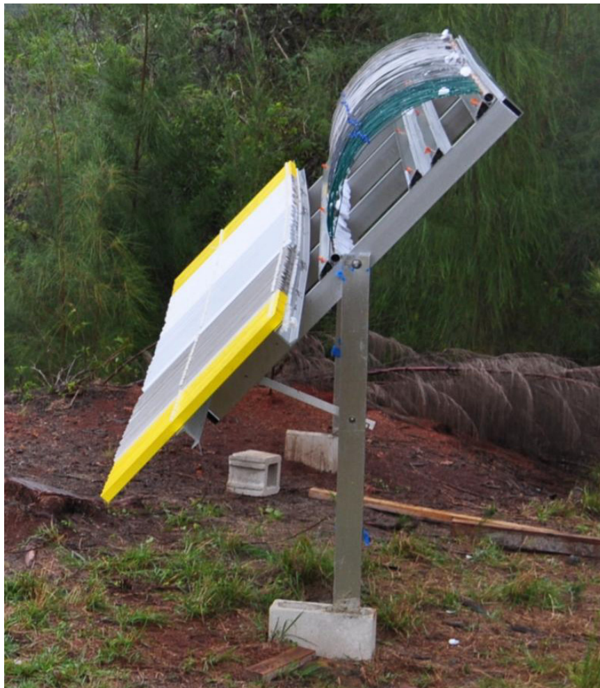
Figure 11. Railing and wire coupons installed on ASTM G7 exposure rack placed a 45 degree angle at KTA.
