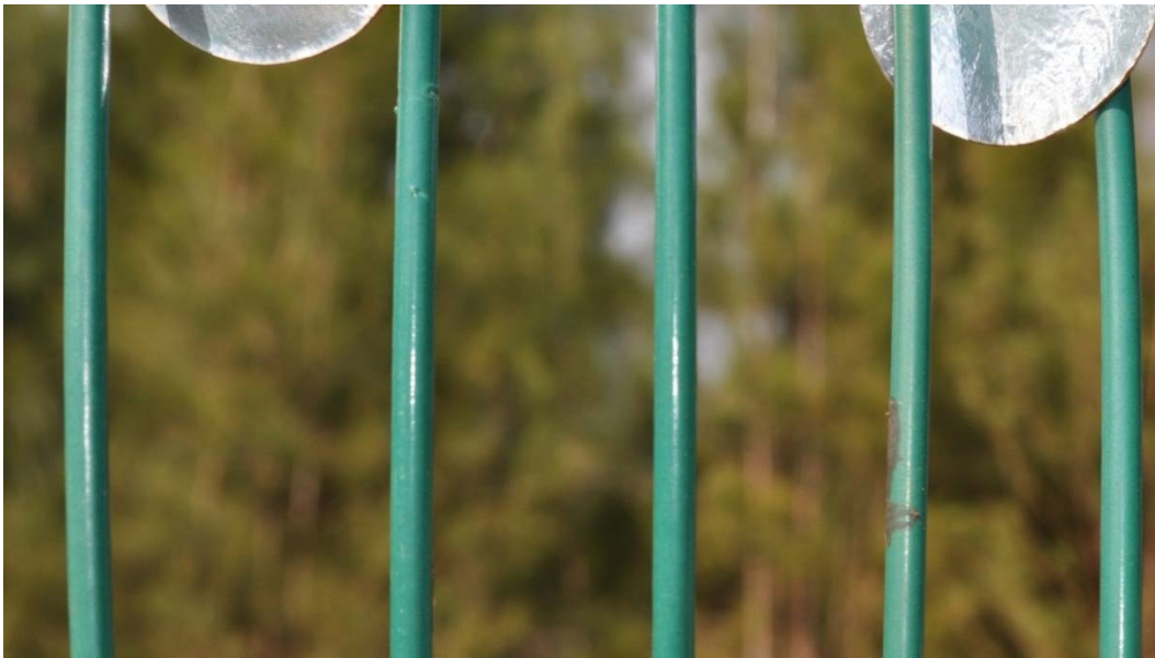
Figure B90. Fuse Bonded PVC Coated Galvanized Wire Coupon
