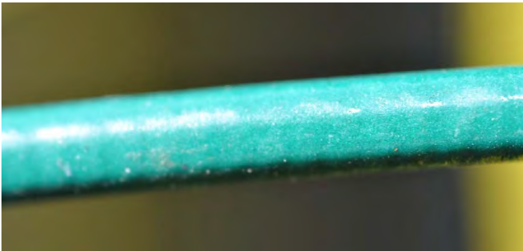
Figure B178. Fuse Bonded PVC Coated Galvanized Wire Coupon
