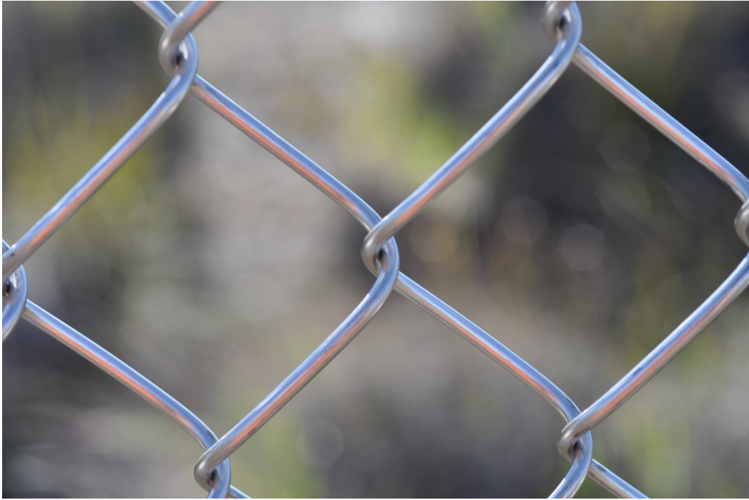
Figure A9. Aluminum after 6 months exposure.
