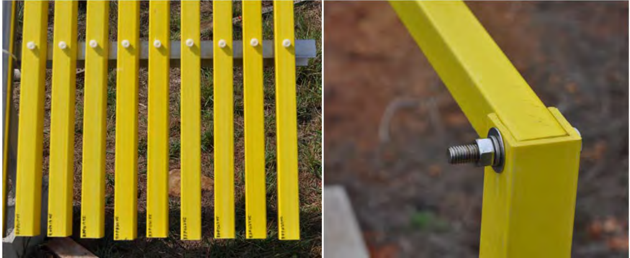
Figure B68. (Left) FRP railing coupons. (Right) FRP railing test section.
