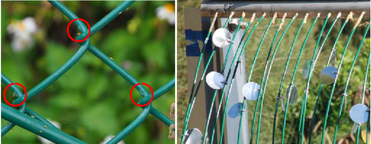
Figure B71. (Left) Fused bonded PVC coated galvanized steel formation damage. (Right) PVC coated galvanized steel wire coupons
