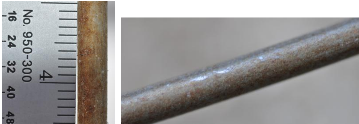
Figure 27. Stainless Steel wire coupon at FRF (left) and KTA (right) after 12 months of exposure.
