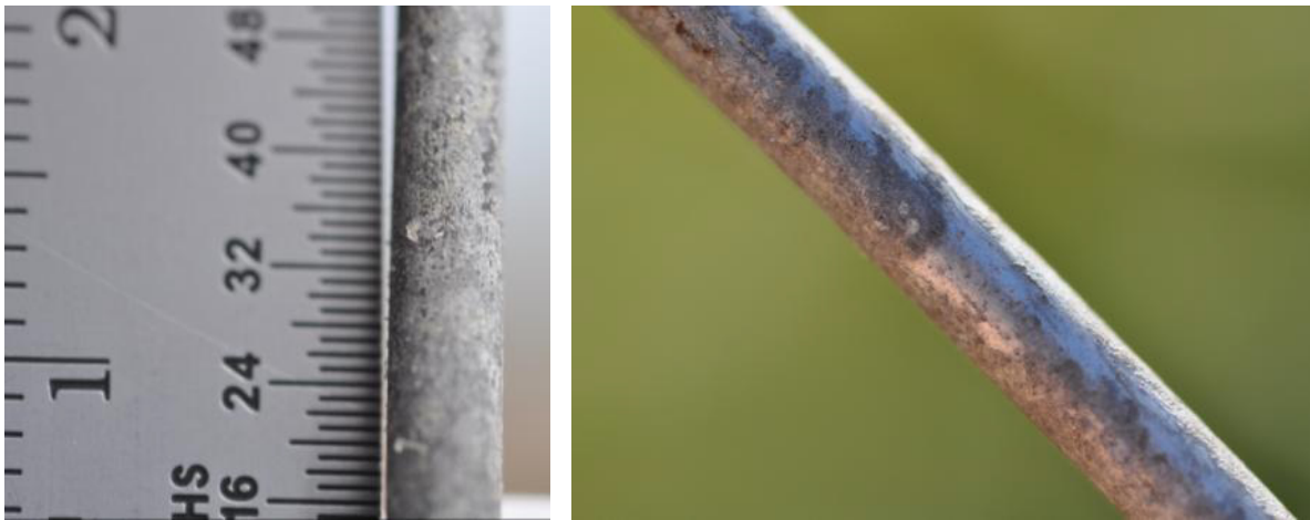
Figure 24. Aluminized steel wire coupon at FRF (left) and KTA (right) after 12 months of exposure.
