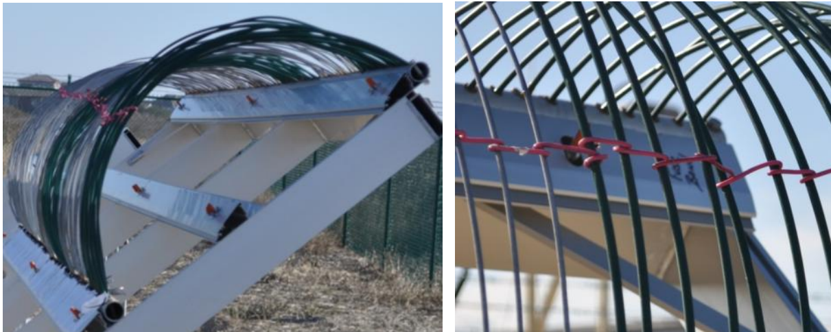
Figure 9. Profile of wire coupons on ASTM G7 rack (left) and method of separating specimens using a plastic-coated wire (right).
