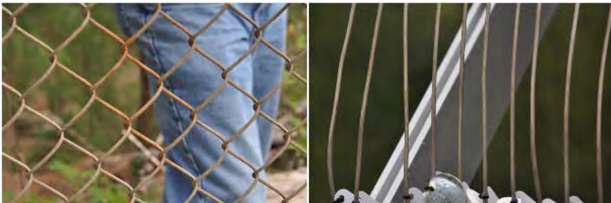
Figure B70. (Left) Stainless steel fence after 3 months exposure. (Right)Stainless steel wire coupons after 3 months exposure.
