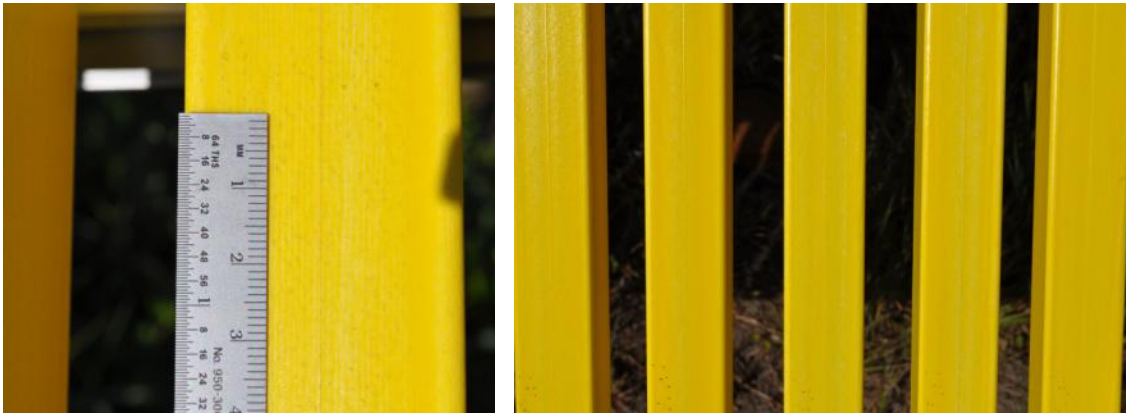
Figure 29. FRP railing coupon at FRF (left) and KTA (right) after 6 months of exposure.
