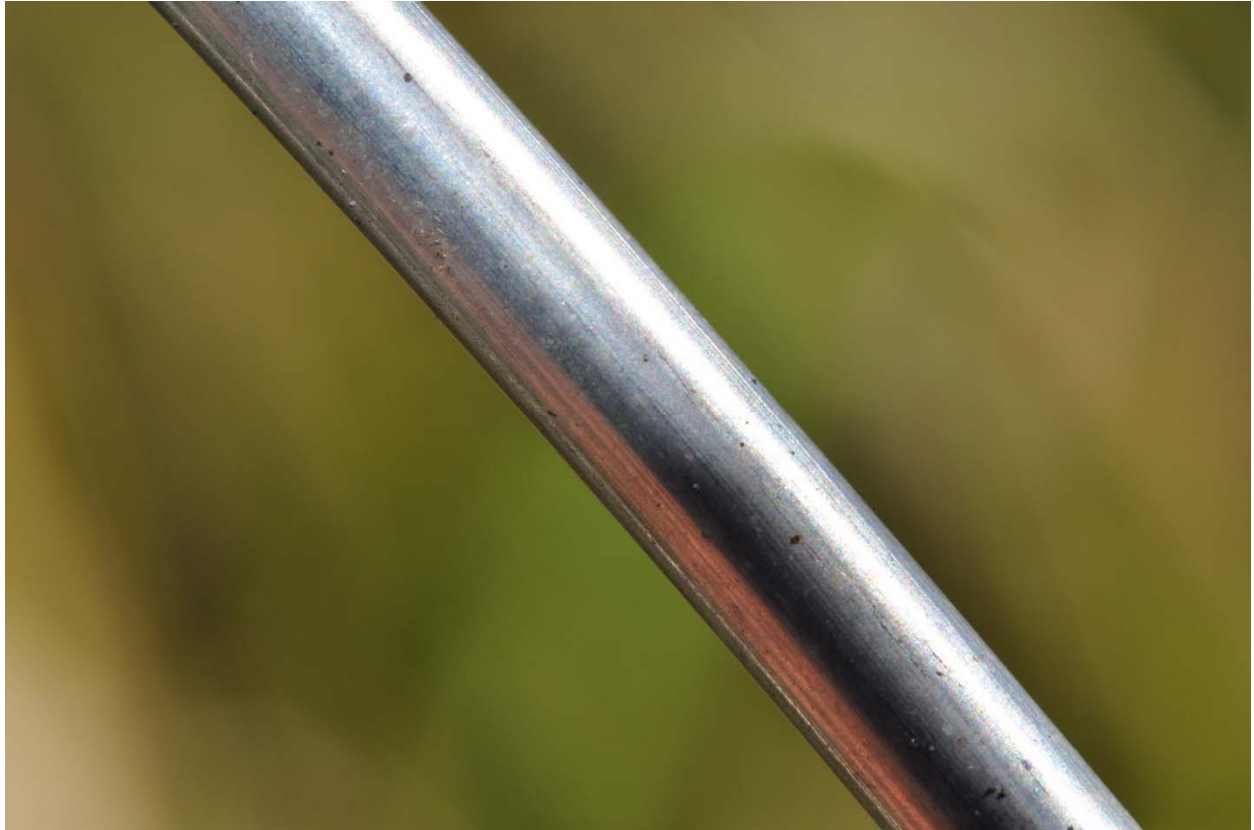
Figure B131. Aluminum Wire Fencing
