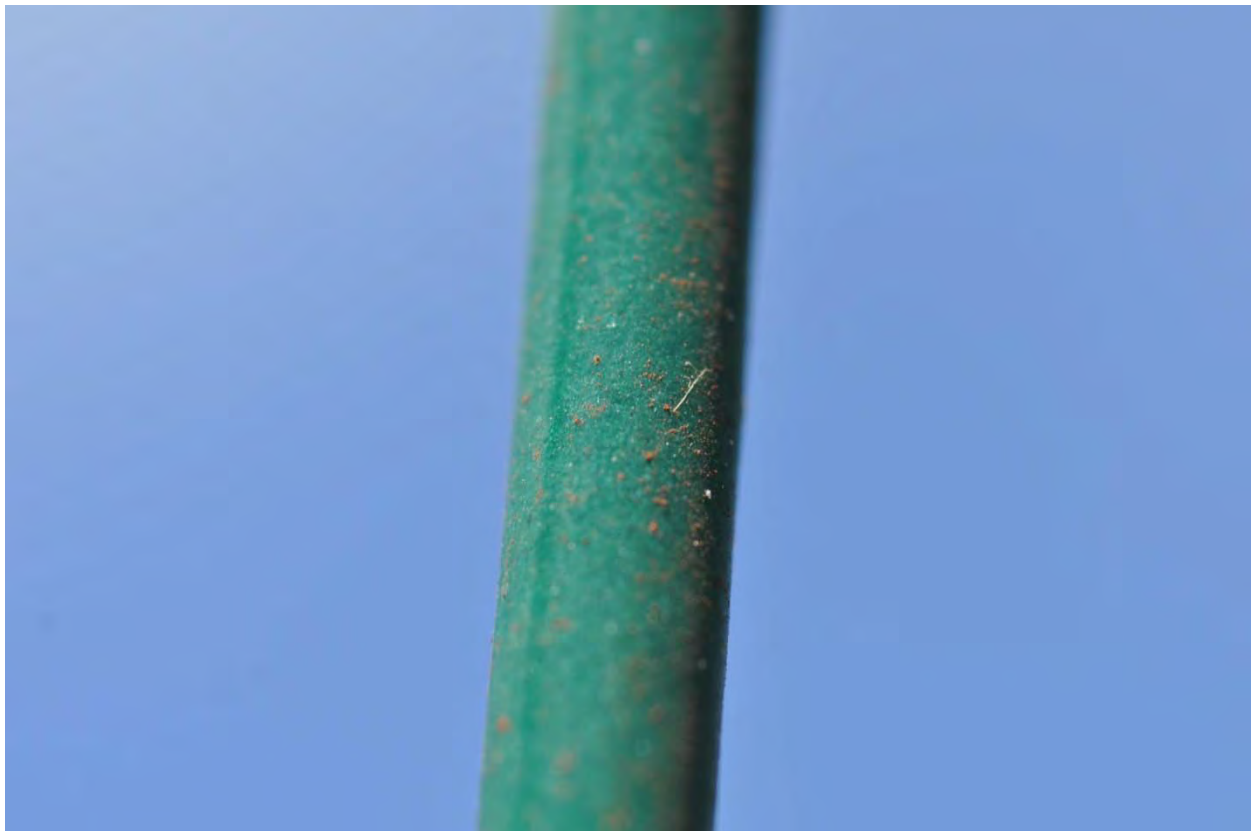
Figure B109. Fuse Bonded PVC Coated Galvanized Wire Coupon
