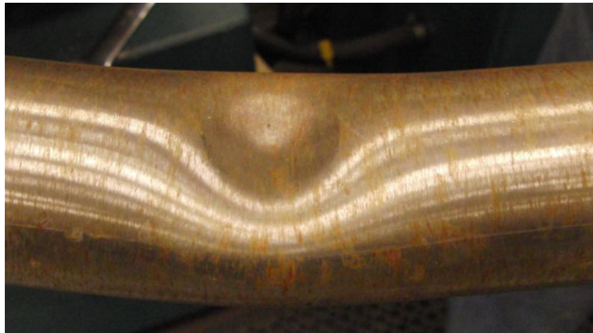
Figure 47. Cross sectional collapse of a stainless steel pipe under flexure testing.
