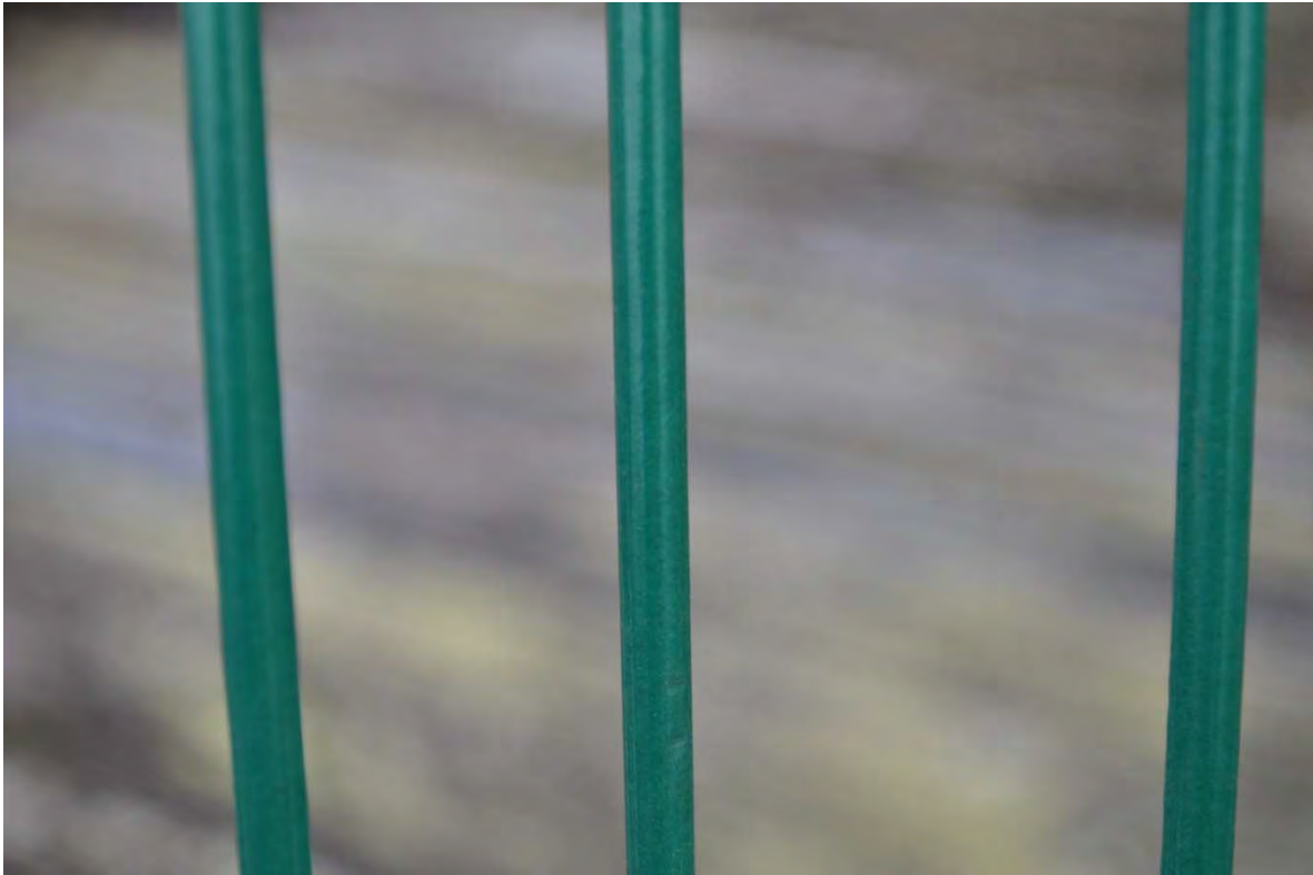
Figure B156. Fuse Bonded PVC Coated Galvanized Wire Coupon
