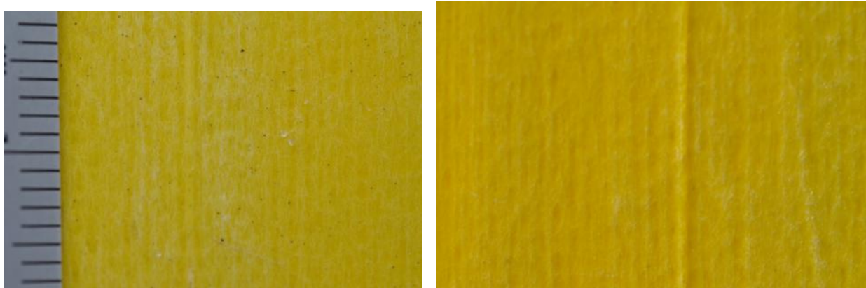
Figure 33. FRP railing coupon at FRF (left) and KTA (right) after 12 months of exposure.
