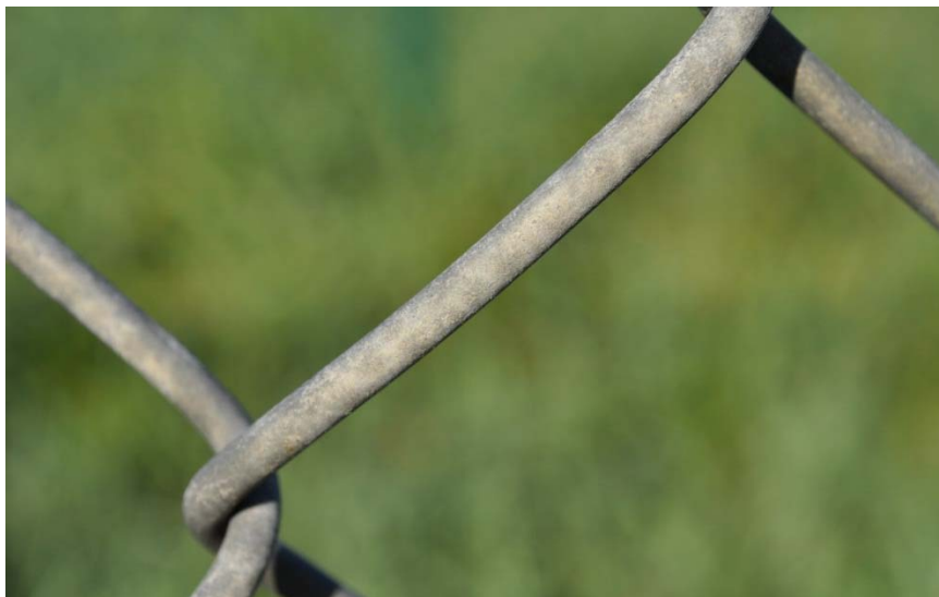
Figure B41. Galvan Wire Fencing
