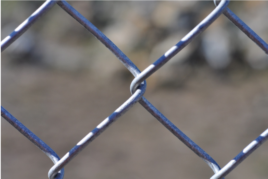
Figure A11. Aluminized after 6 months exposure.
