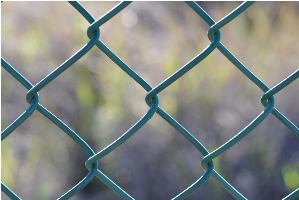
Figure A12. Standard PVC after 6 months exposure.
