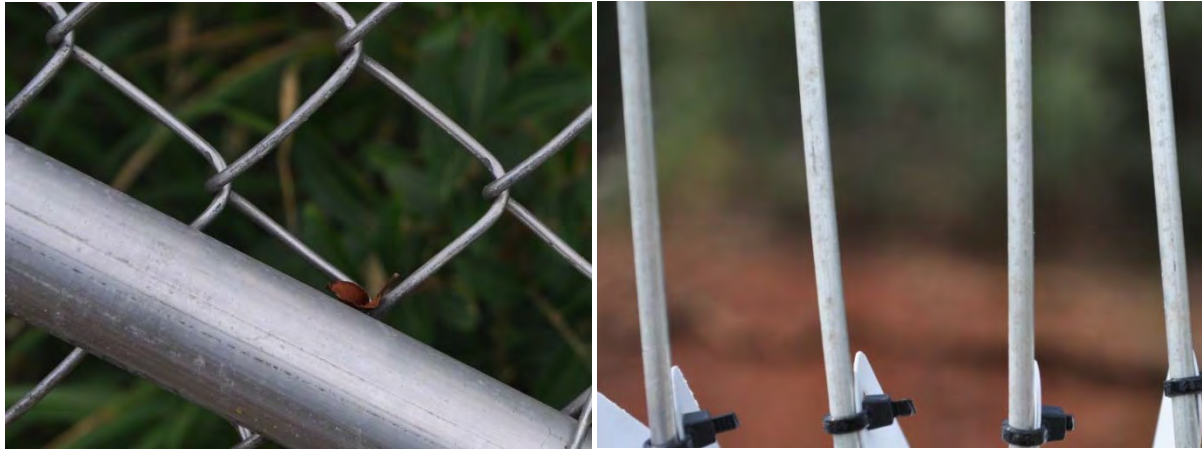
Figure B74. (Left) Aluminum fabricated fencing. (Right) Aluminum Wire Coupons
