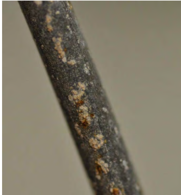
Figure B136. Galfan Wire Coupon
