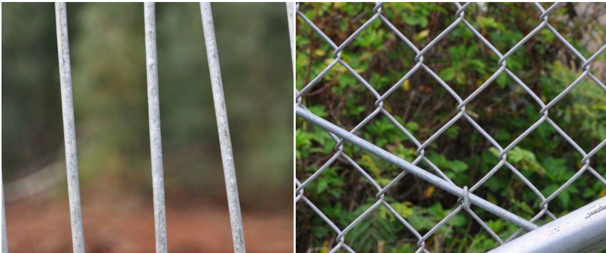
Figure B72. (Left) Aluminized Steel Wire Coupons. (Right) Aluminized Steel fabricated fencing
