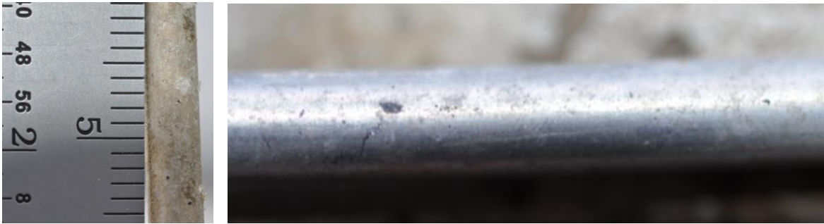
Figure 26. Aluminum wire coupon at the FRF (left) and KTA (right) after 12 months of exposure.
