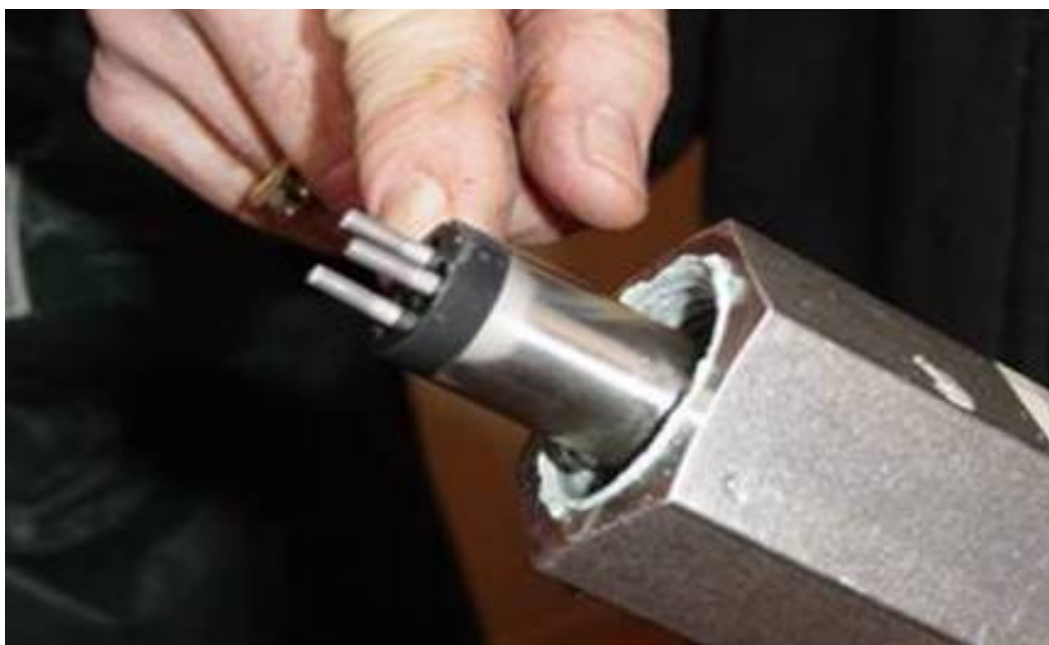
Figure 2. Electrodes on corrosion rate probe.
