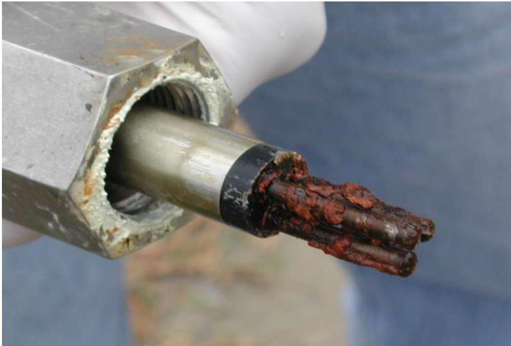
Figure 23. As-removed appearance of LPR probe electrodes from Simmons Army Airfield.
