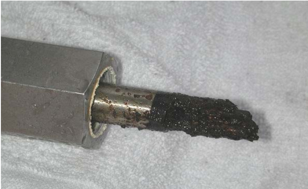
Figure 21. As-removed appearance of LPR probe electrodes from the raw water location.
