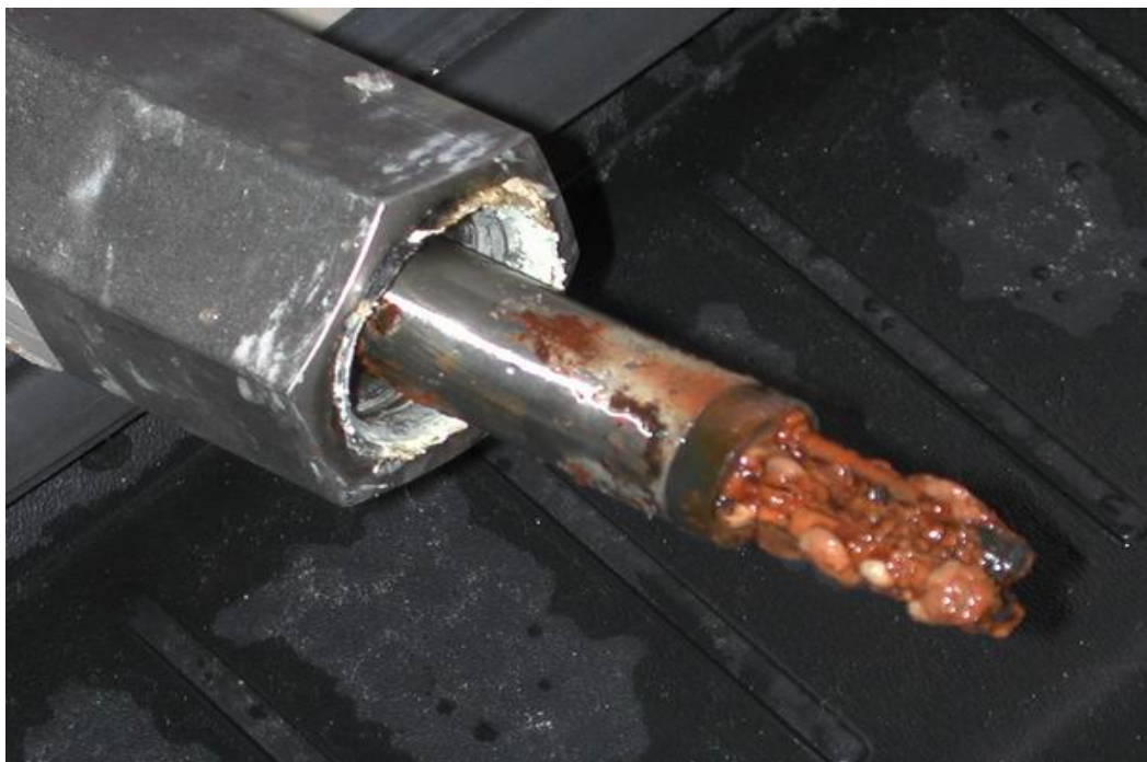
Figure 24. As-removed appearance of LPR probe electrodes from Tank Hill.
