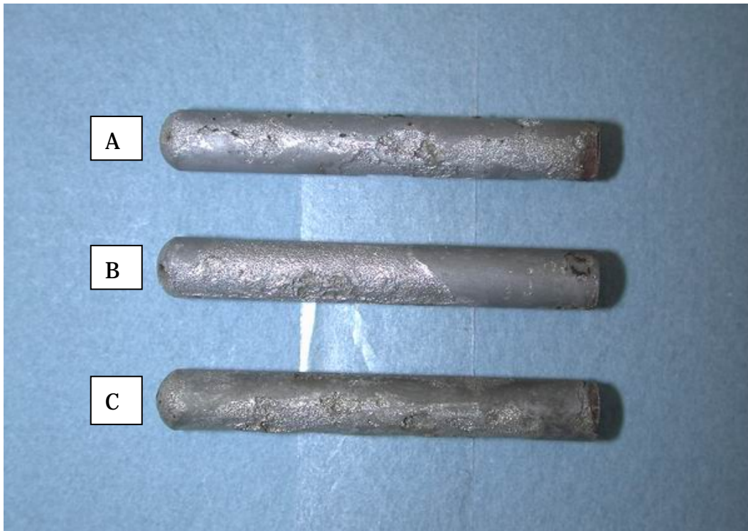
Figure 27. After-cleaning appearance of LPR probe electrodes from the Simmons Army Airfield (item C is freely corroding electrode).
