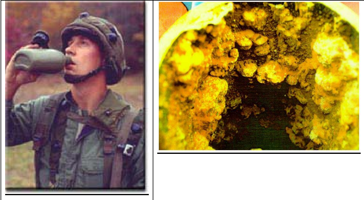
Figure 1. a. Water is vital to Army readiness; b. Severely corroded water distribution pipe.
