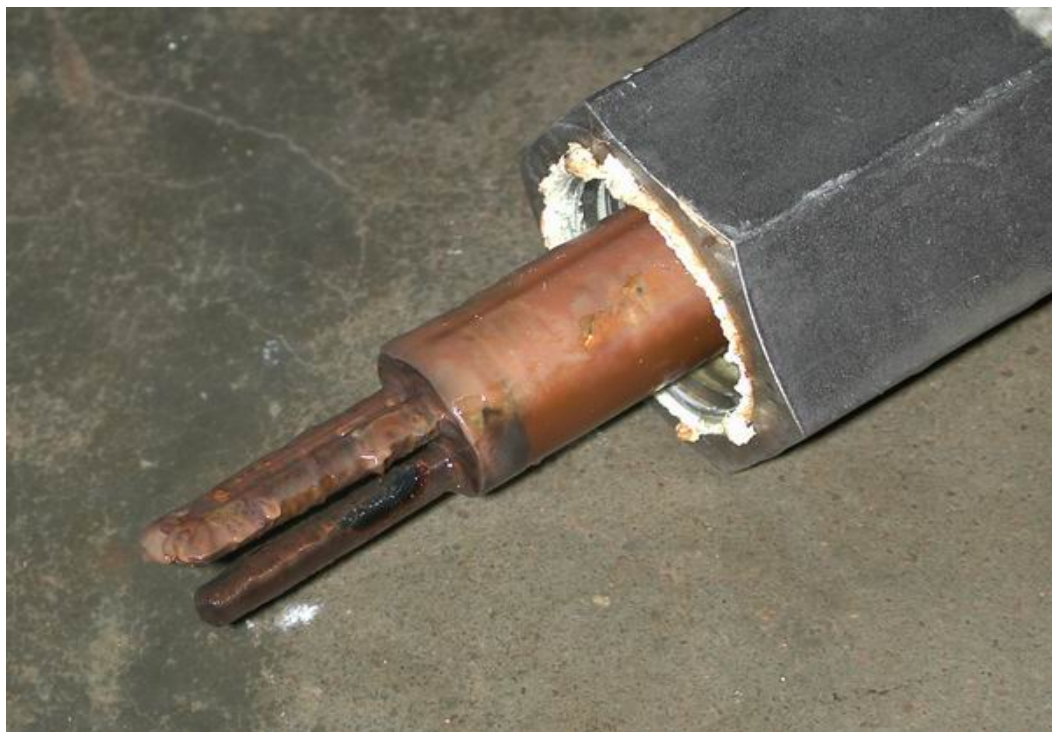
Figure 22. As-removed appearance of LPR probe electrodes from the treated water location.
