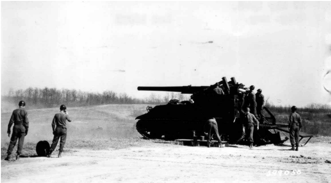
Figure 132. Members of gun crew prepare to fire a self-propelled 155 mm gun at Fort Knox, KY, 1947 (NARA College Park, RG 111-SC WWII, box 602, photo SC299050).
