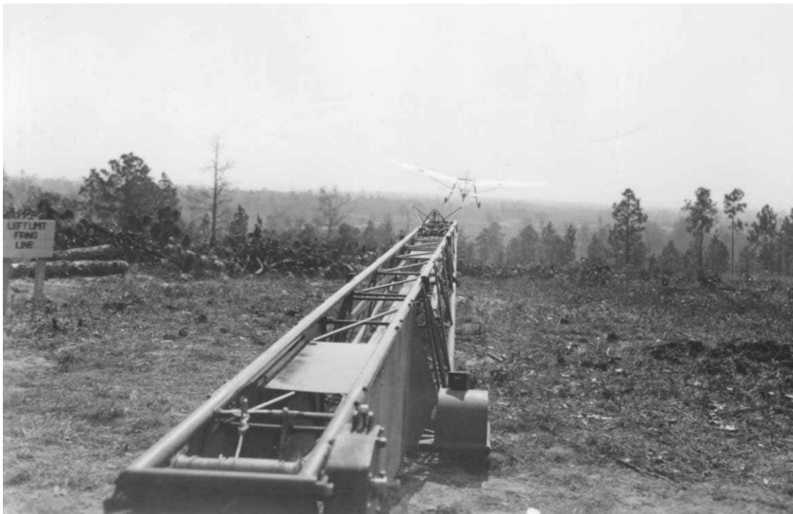
Figure 52. Radio-controlled airplane target OQ-2A taking off from catapult at the AA range at Fort Jackson, SC, 1 November 1943 (NARA College Park, RG 111-SC WWII, box 415, photo SC246692).
