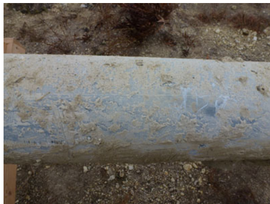
Bare steel pipe after exposure with cathodic protection in native soil (top); soil cement (bottom left); and flowable fill (bottom right)
