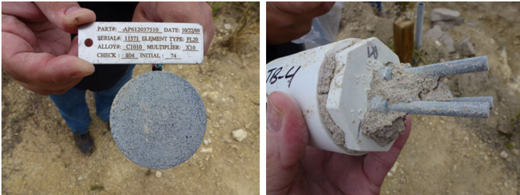
Figure 26. ER probe (left) and LPR probe (right) after extraction from flowable fill with JB4.
