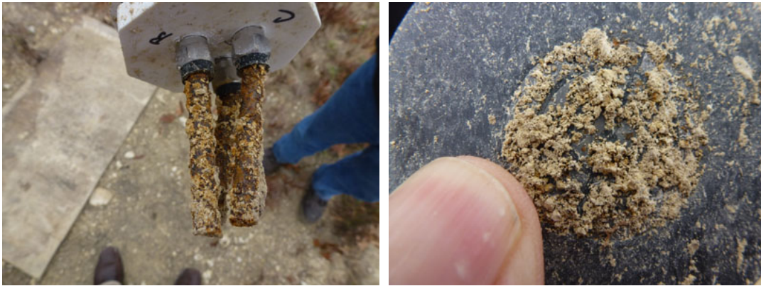
Figure 21. LPR probe (left) and ER probe (right) after extraction from native soil with JB3.
