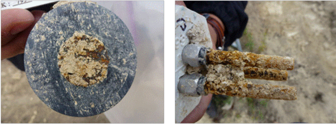
Figure 36. ER probe (left) and LPR probe (right) after extraction from native-soil backfill with JB6.
