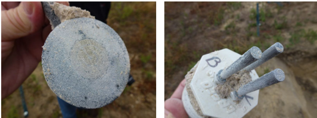
Figure 10. ER probe (left) and LPR probe (right) after extraction from flowable fill specimen JB1.
