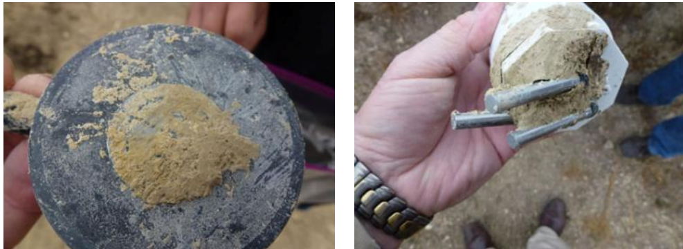
Figure 16. ER probe (left) and LPR probe (right) after extraction from the soil cement with JB2.
