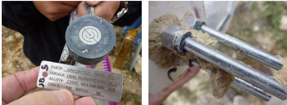
Figure 31. ER probe (left) and LPR probe (right) after extraction from soil cement with JB5.
