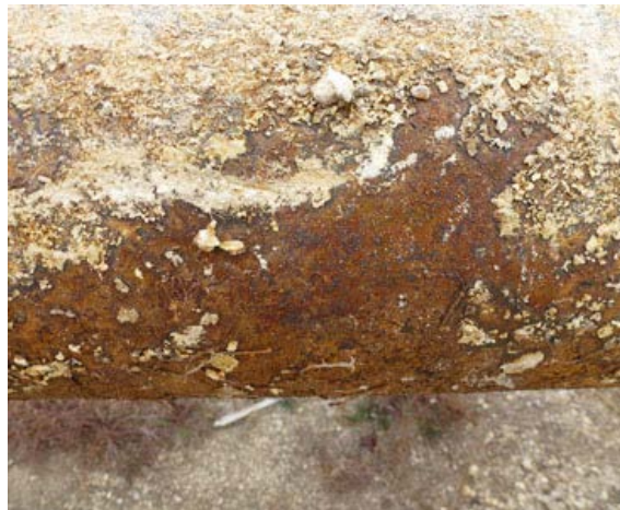
Bare steel pipe after exposure with cathodic protection in native soil (top); soil cement (bottom left); and flowable fill (bottom right)
